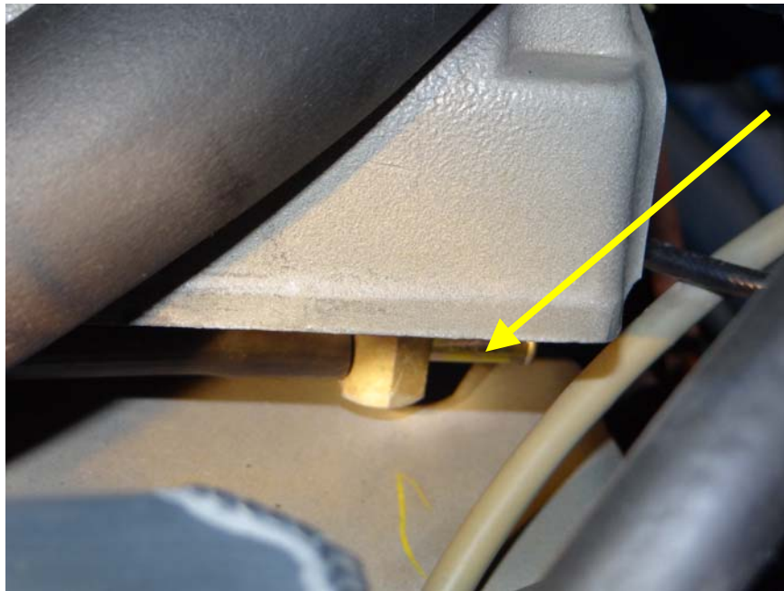
Step 8: Insert new hose over intake nipple.
