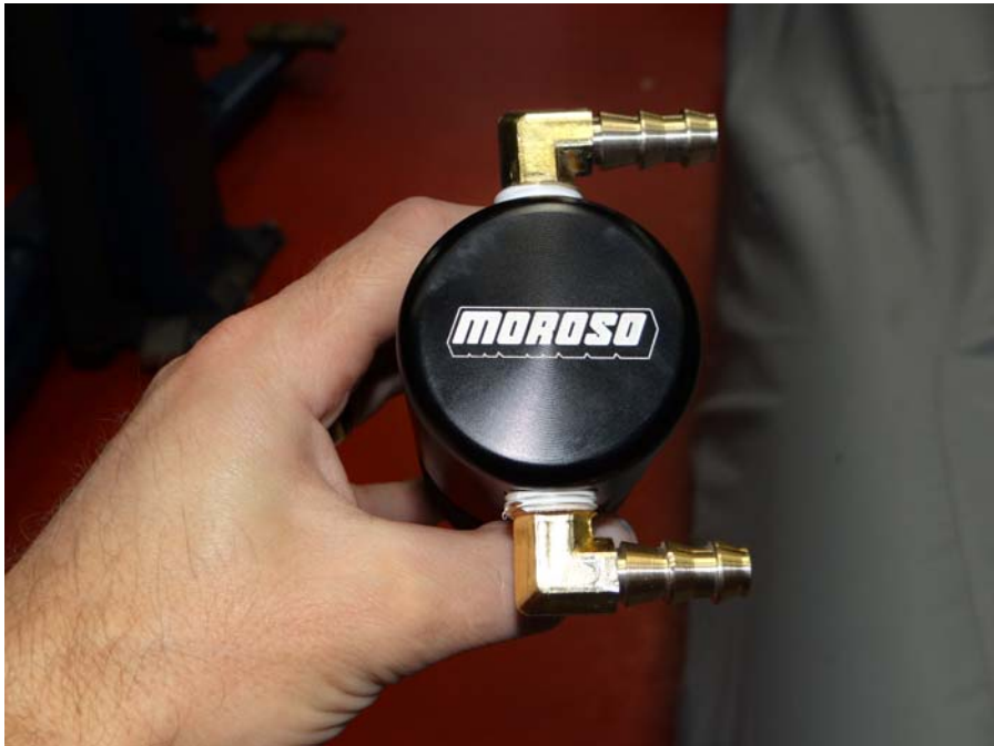
Step 14: Assemble Air Oil Separator as shown using Teflon tape on fittings.
