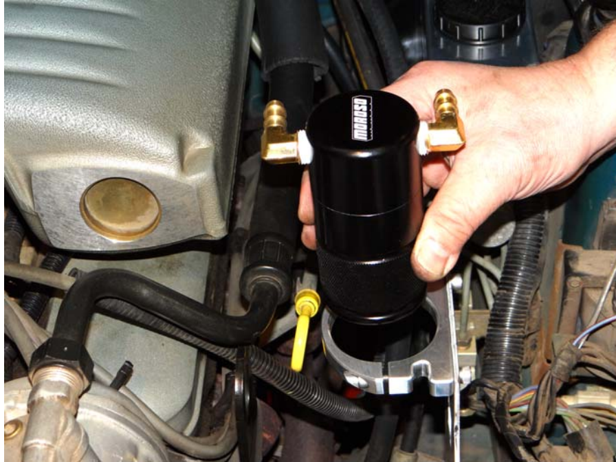
Step 15: Insert Air Oil Separator into billet clamp.
