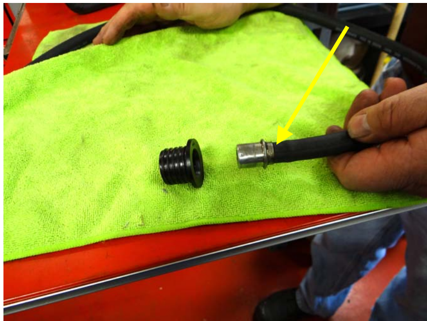
Step 4: Insert new hose over PCV valve nipple.
