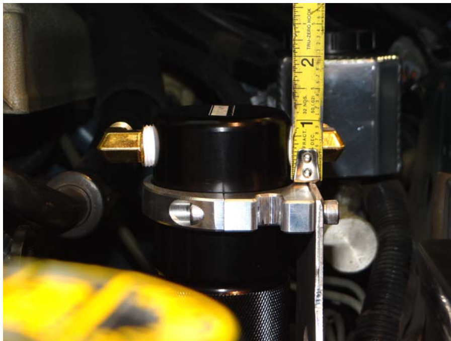
Step 16: Set height to 1'-1 1/8'' and tighten clamp.
