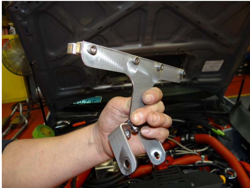
Step 17: Assemble billet clamp saddles to stainless steel mount using (4) \frac{1}{4} -20x \frac{5}{8} SHCS.
