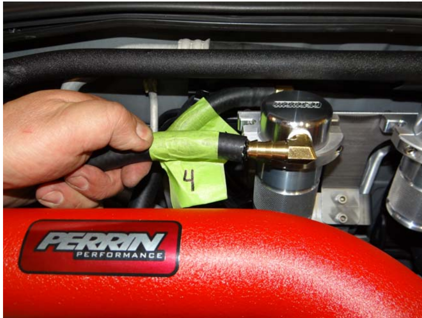
Step 27: Install 1/2" hoses (3) and (4) as shown.
