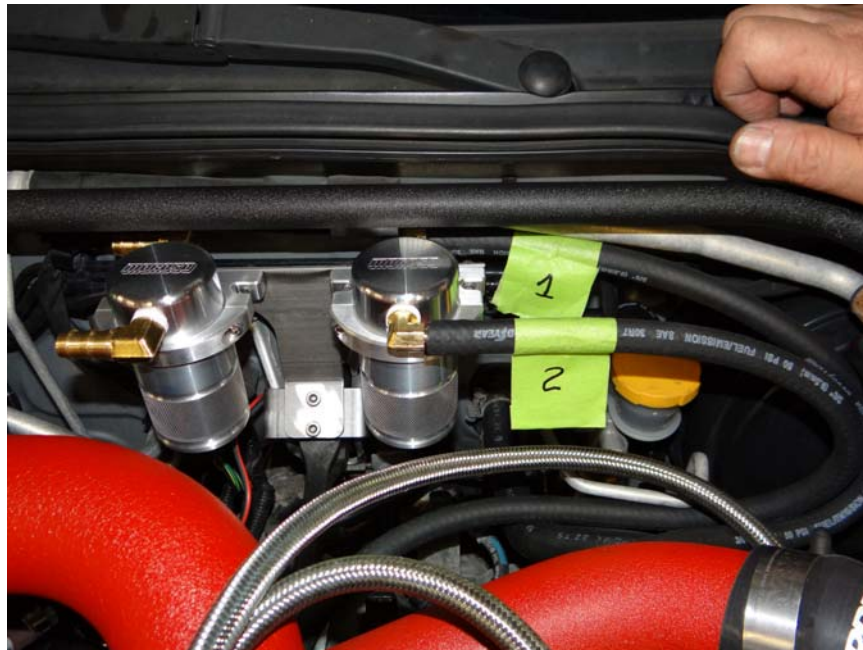
Step 26: Install 3/8" hoses (1) and (2) as shown.
