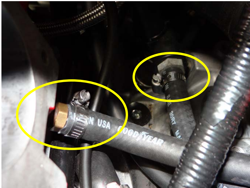
Step 2: Locate and remove stock PCV hose from vehicle, using 3/8" hoses provided in kit install as shown with hose clamps.
