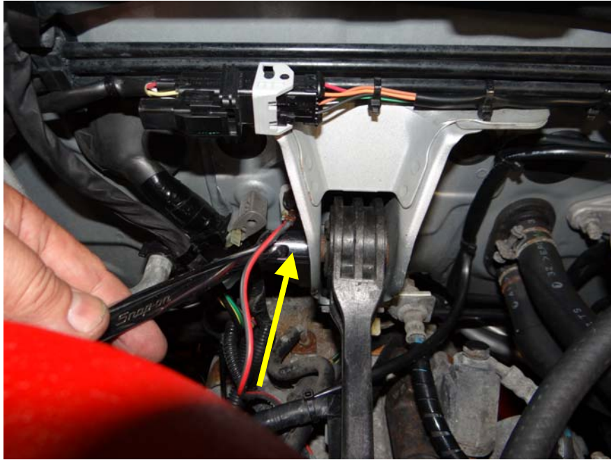
Step 18: Locate and remove rear torque arm bolt.
