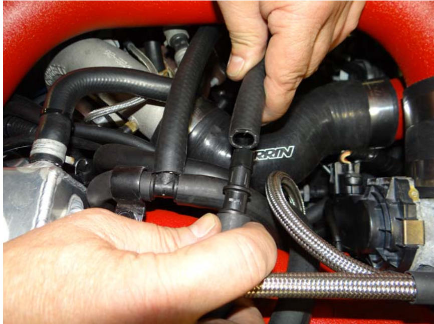
Step 14: Insert other 1/2" hose provided in kit over 1/2" coupling and route as shown.
