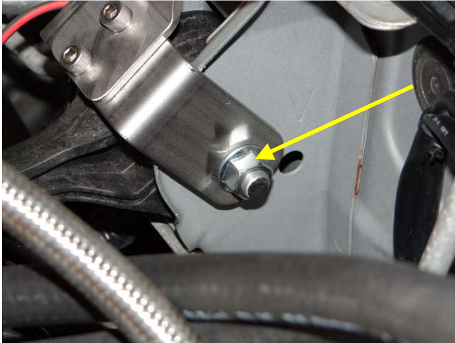
Step 20: Install and tighten jam nut and lockwasher.
