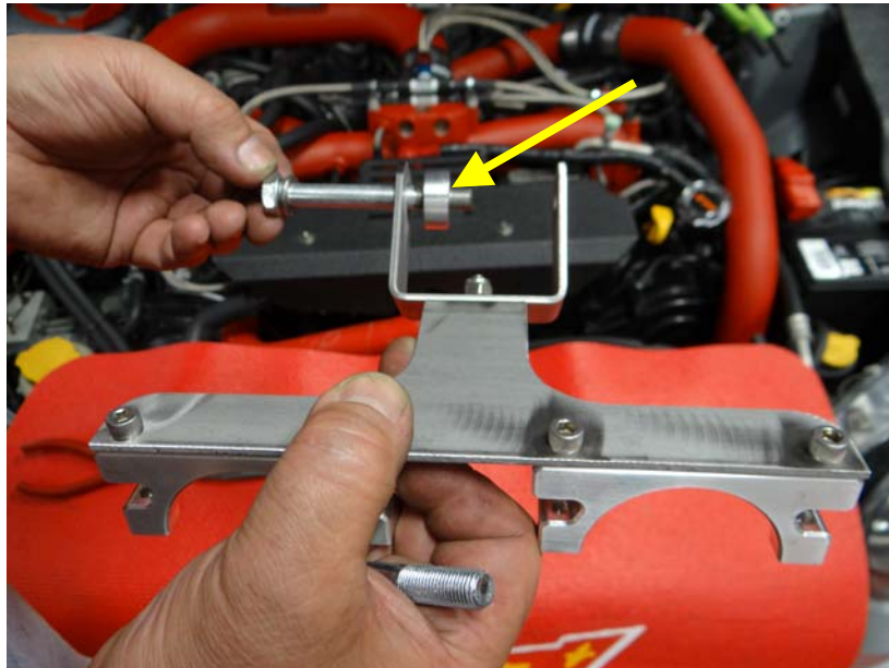
Step 19: Using bolt flat washer and spacer provided in kit assemble as shown above with spacer on inside of stainless bracket
