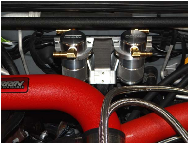
Step 24: Repeat step 23 using air oil separator with 1/2" barbed fittings.
