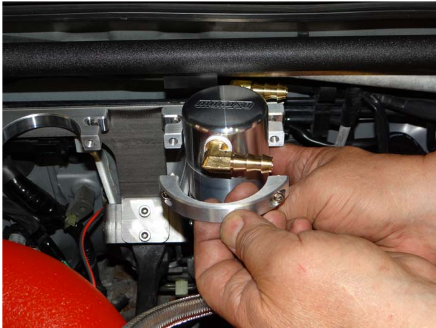
Step 23: Install air oil separator with 3/8" barbed fitting as shown using (2) 1/4-20x5/8 SHCS.
