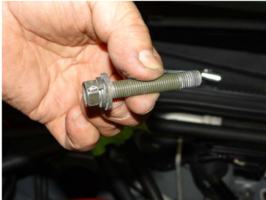
Step 18: Locate and remove rear torque arm bolt.
