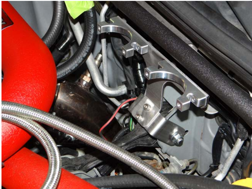
Step 20: Install and tighten jam nut and lockwasher.
