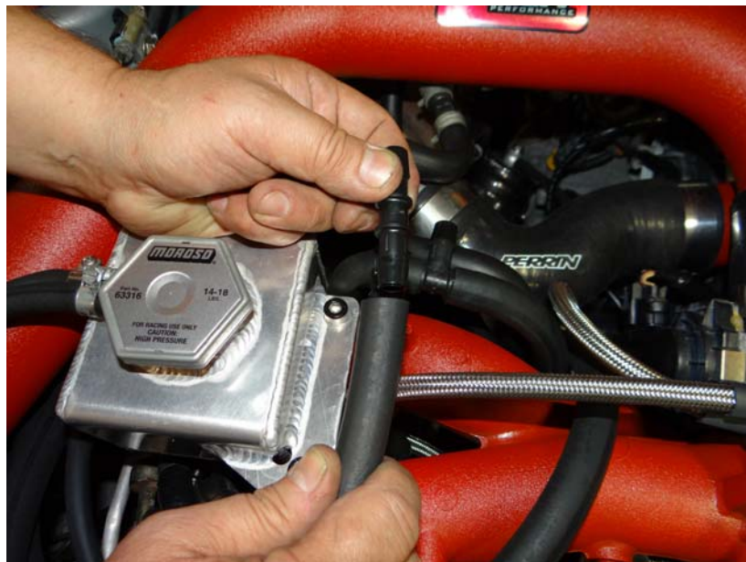
Step 11: Insert 1/2" coupling provided in kit into original hose running to cold air intake tube.
