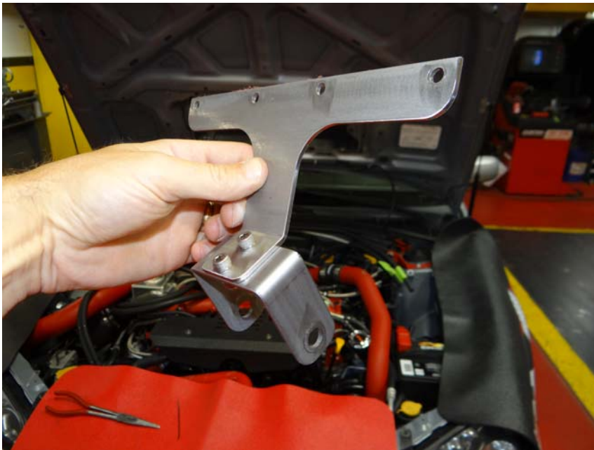
Step 16: Assemble stainless steel mounting bracket as shown using (2) 1/4-20x5/8 SHCS and (2) 1/4-20 nuts
