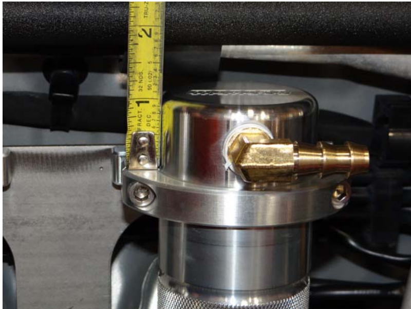
Step 25: Set height on both air oil separators to 1" to 1 1/8".
