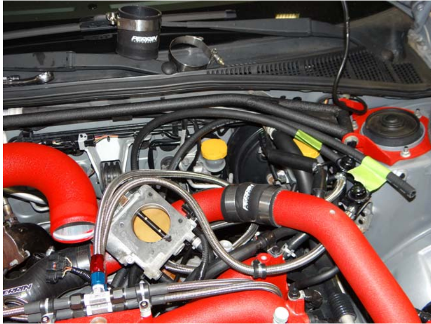
Step 4: Route hose to rear of engine as shown.
