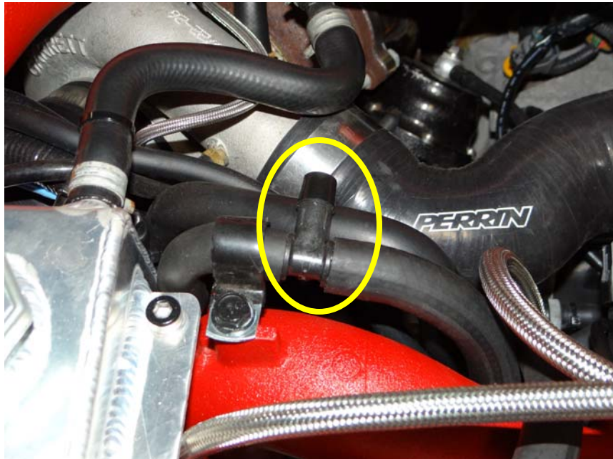
Step 10: Rotate "T" towards firewall / rear of engine.
