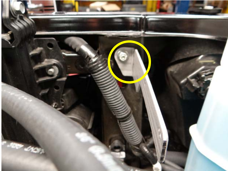
Step 8: Install stainless steel mounting bracket as shown using 5/16-18x1 HHCS, 5/16-18 nylock nut and 5/16 flat washer.
