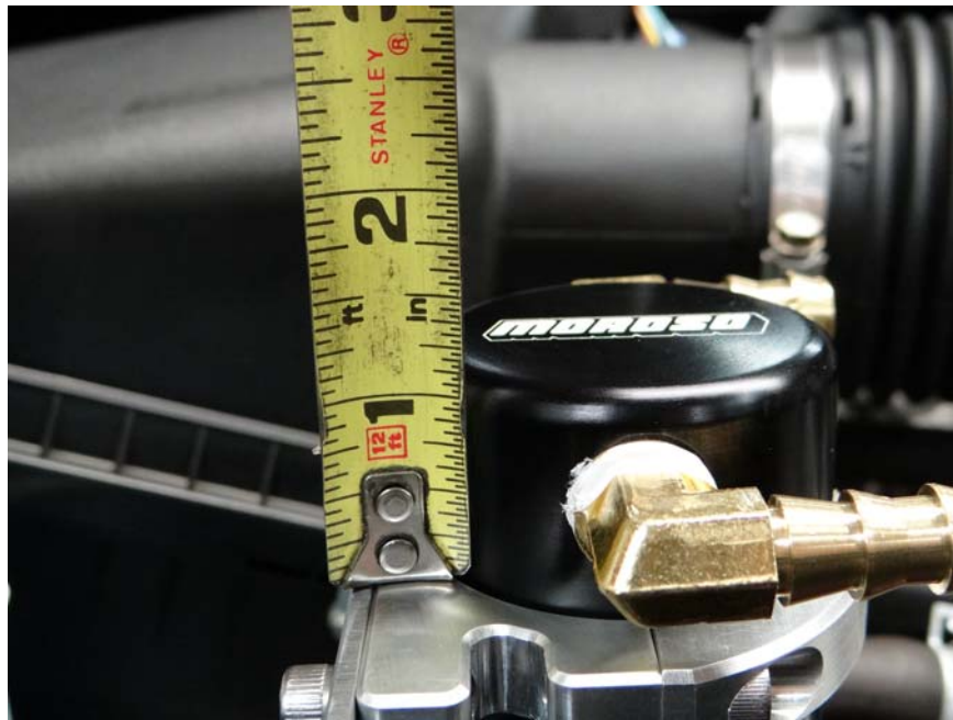
Step 13: Set height to 1 1/8" as shown and tighten clamp bolts with fittings facing engine.
