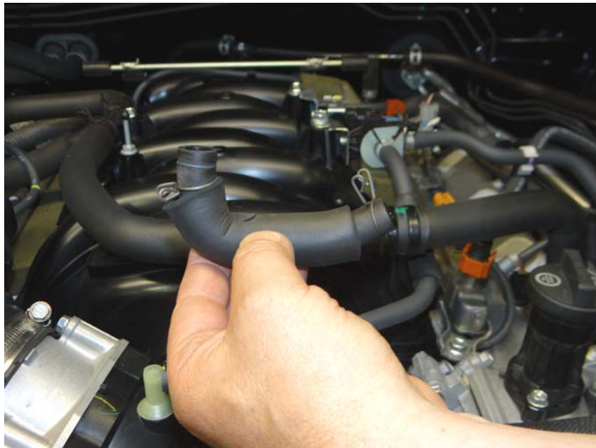
Step 3: Remove PCV line from vehicle.
