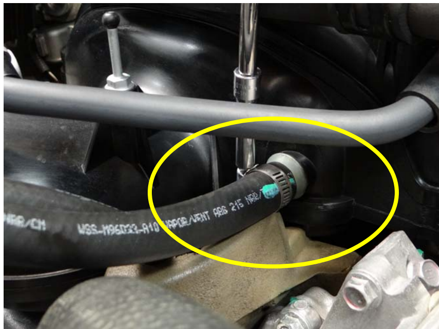
Step 5: Using 1/2" length of hose and hose clamp install over intake nipple.
