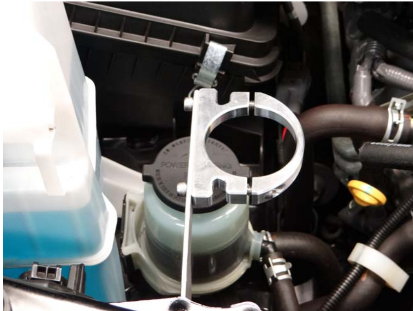
Step 10: Assemble billet clamp assembly to stainless steel mounting bracket using (2) 1/4-20x5/8 SHCS, make sure relief's are facing down.
