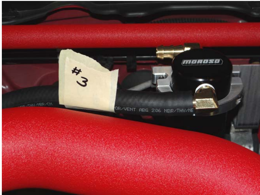
Step 40: Install line #3 and line #4 to Air Oil Separator as shown.
