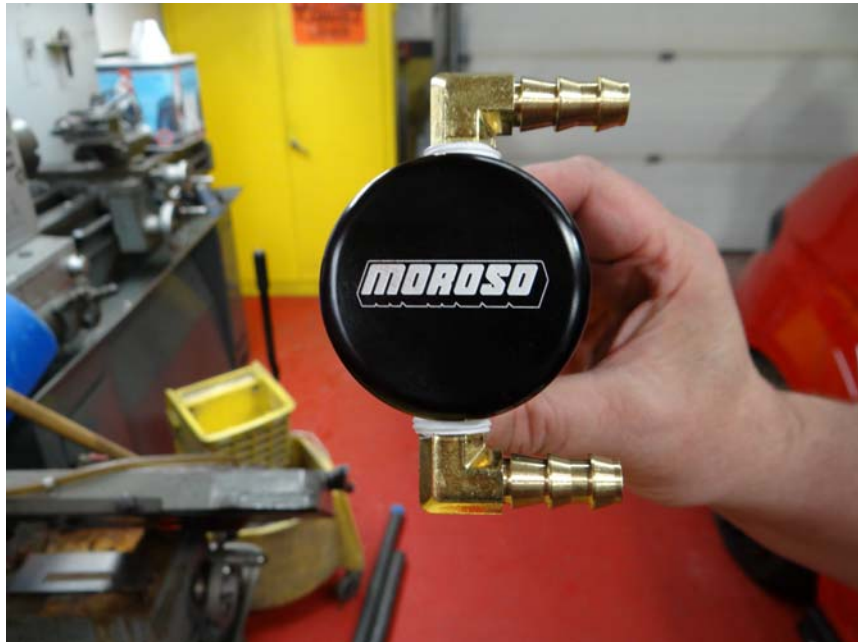
Step 36: Assemble second Air Oil Separator as shown using (2) 3/8" barbed fittings, apply Teflon tape to fittings.
