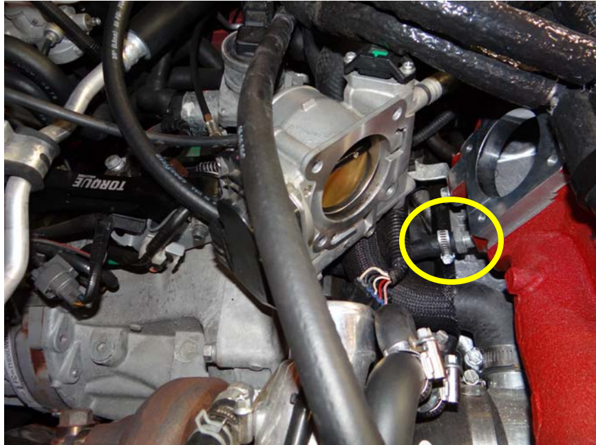
Step 18: Install one over PCV valve nipple and secure with hose clamp.
