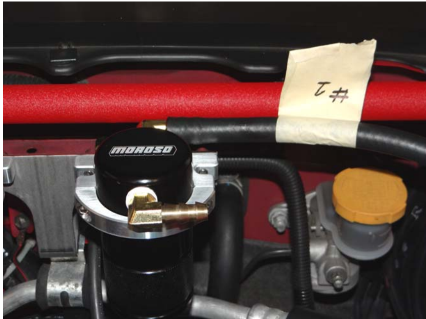
Step 39: Install line #1 and line #2 to Air Oil Separator as shown.
