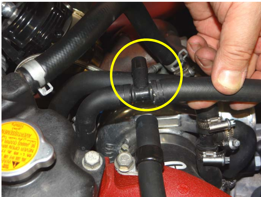
Step 25: Rotate valve cover breather tee towards firewall as shown.
