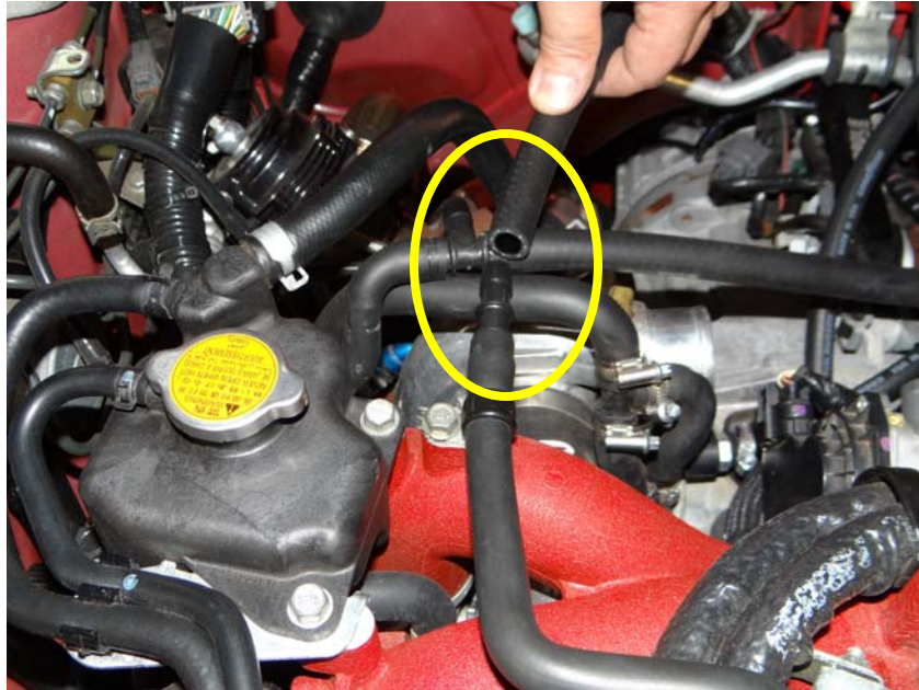
Step 27: connect one end of 18"x 1/2" id hose to coupling as shown.
