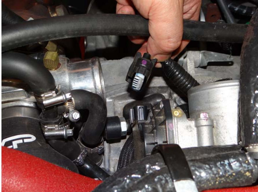
Step 10: Remove electrical connectors from throttle body.
