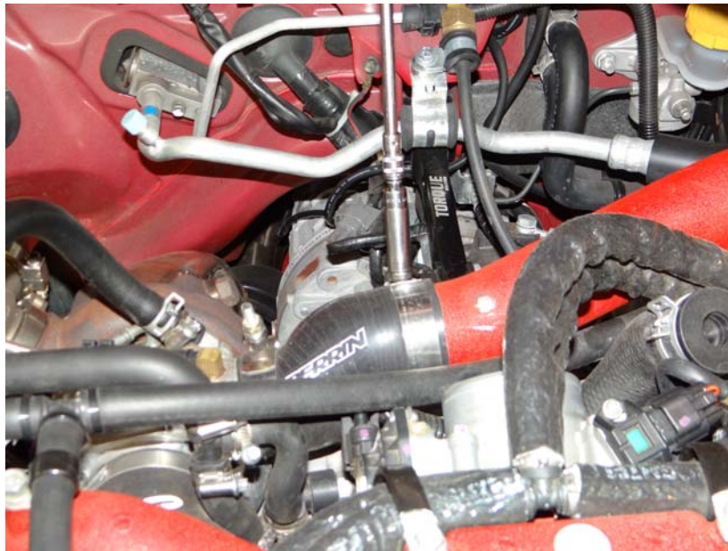
Step 6: Loosen turbo to intercooler tube clamps as shown.
