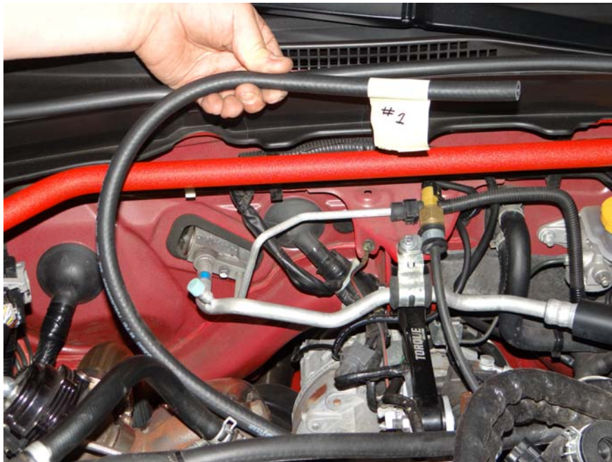
Step 21: Route other end of hose as shown and label #1.
