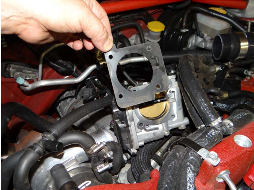
Step 13. Remove and discard throttle body gasket.
