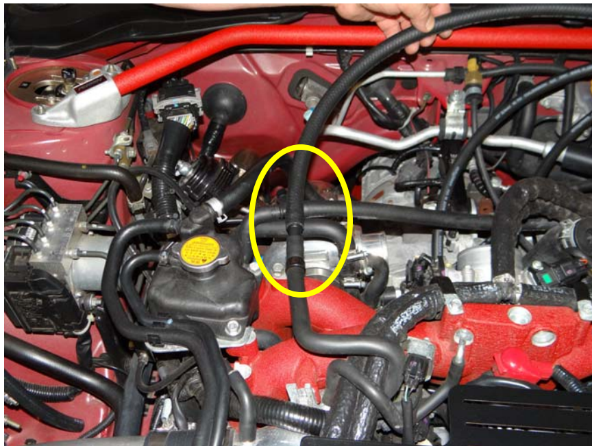
Step 27: connect one end of 18"x 1/2" id hose to coupling as shown.
