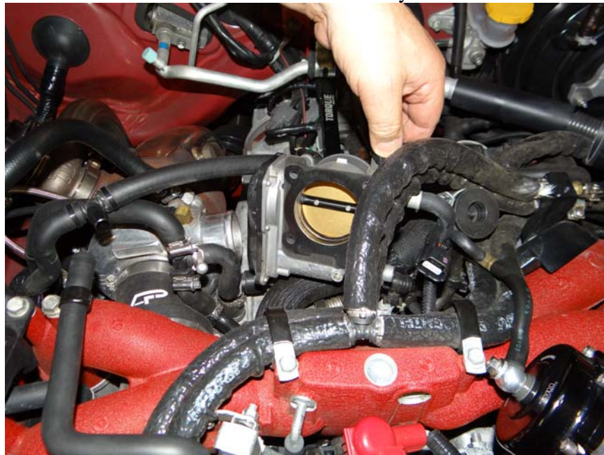
Step 12: Separate throttle body from intake and position out of way.
