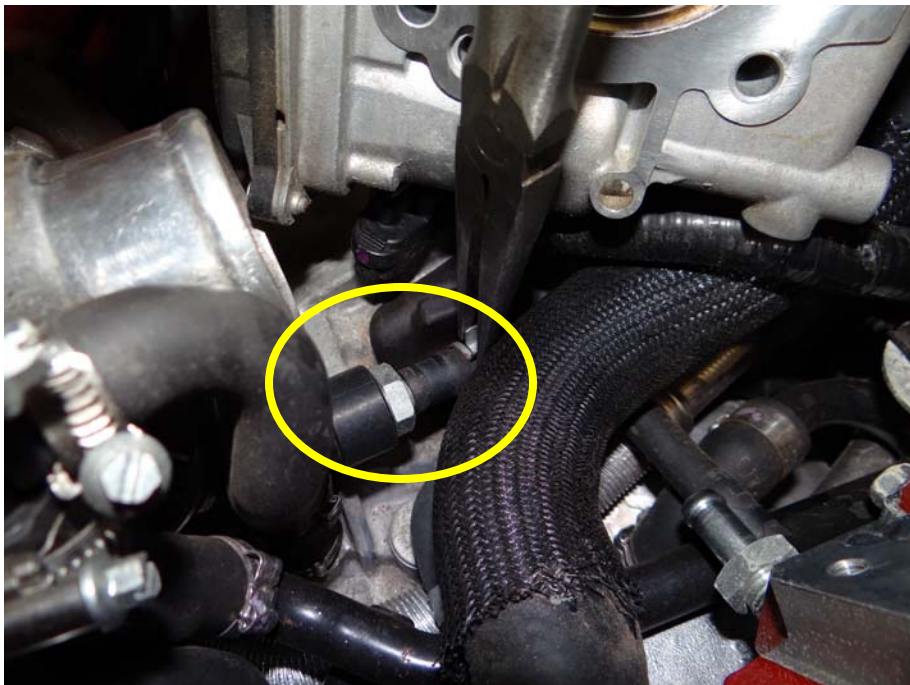
Step 16: Locate and remove other end of hose from crank case nipple.
