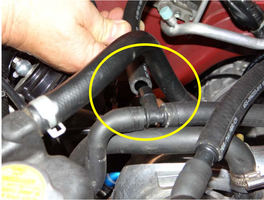
Step 30: connect one end of 18"x 1/2" id hose to tee as shown.
