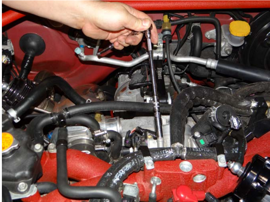
Step 11: Remove bolts securing throttle body to intake manifold. Do not remove coolant lines from throttle body.
