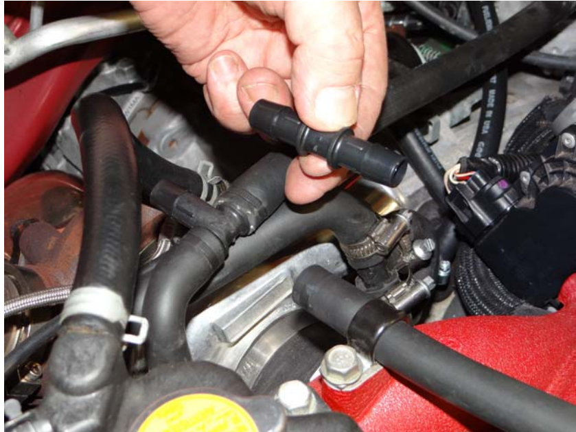
Step 26: Insert coupling into valve cover breather hose.
