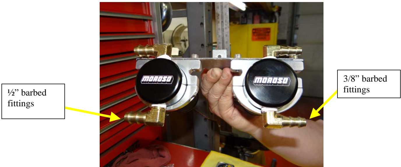
Step 37: Insert Air Oil Separators into billet clamps as shown, position Air Oil Separator in clamp so the bottom can be unthreaded for oil removal.
