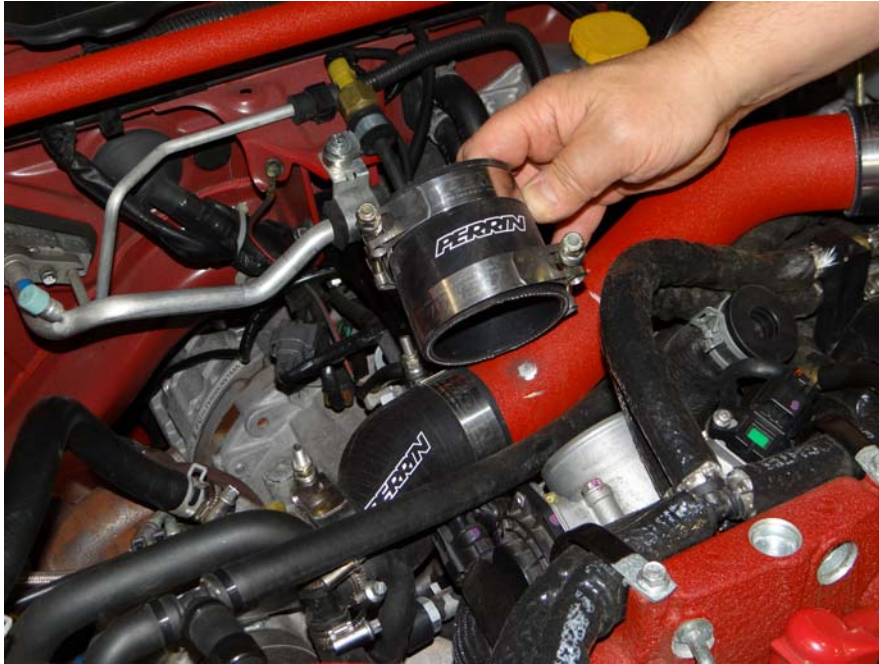
Step 5: Remove throttle body hose.
