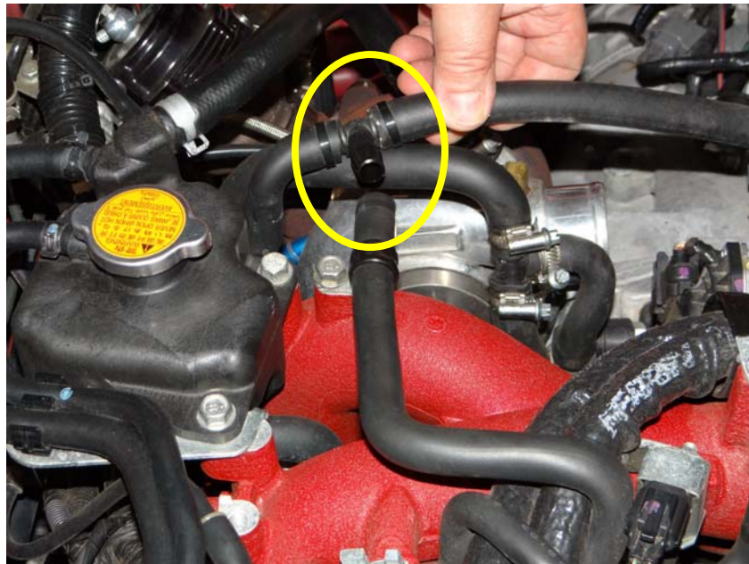
Step 9: Locate and remove valve cover breather hose tee as shown.
