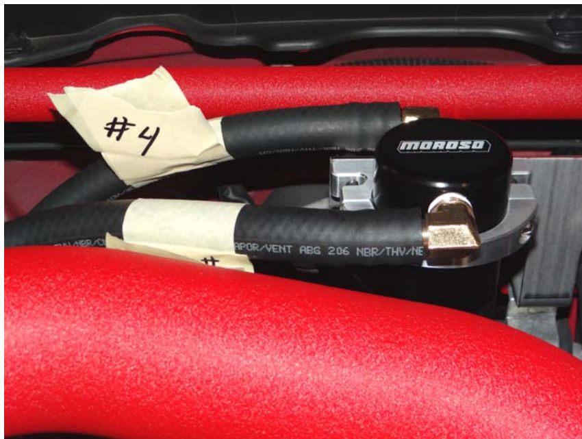
Step 40: Install line #3 and line #4 to Air Oil Separator as shown.
