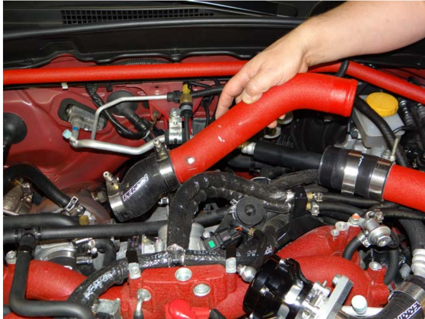
Step 8: Remove turbo to intercooler tube.
