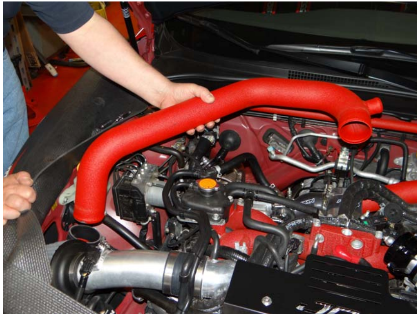
Step 3: Remove intercooler to throttle body tube.
