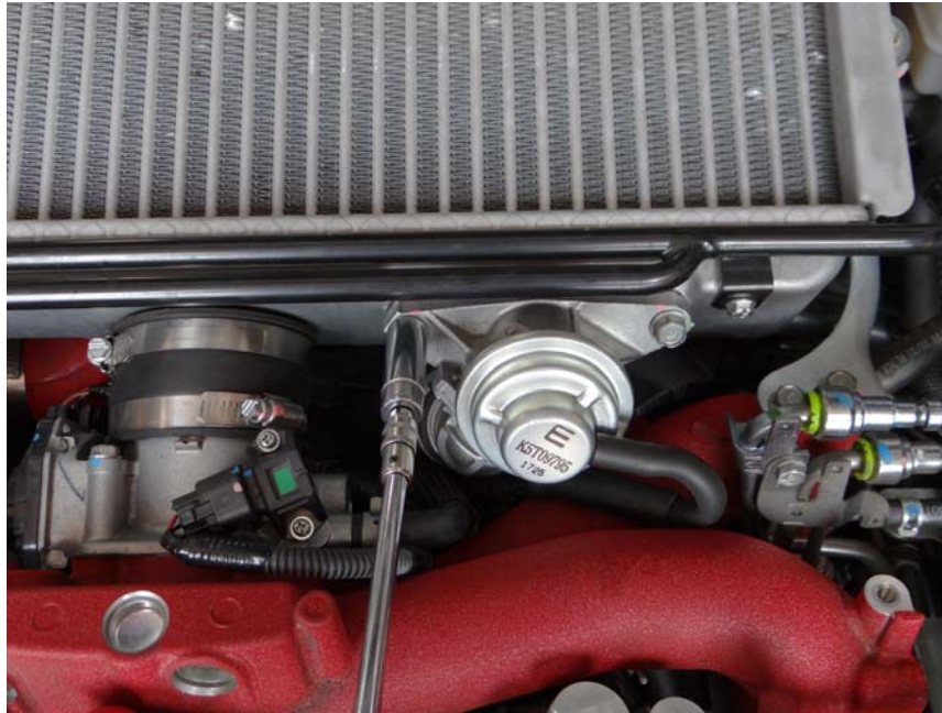
Step 5: Remove relief valve mounting bolts from intercooler.
