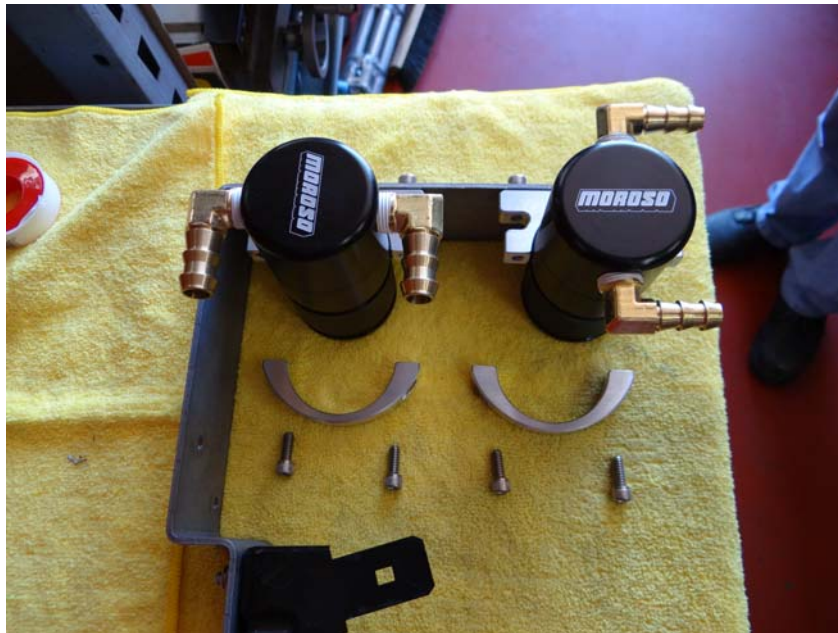
Step 36: Assemble Air Oil Separators to stainless mounting bracket as shown in above illustration.
