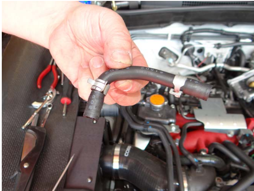
Step 15: Locate other end of PCV line and remove from vehicle.
