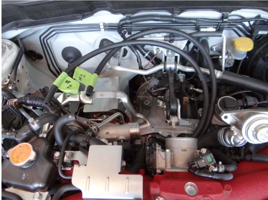
Step 22: Re-install throttle body.
