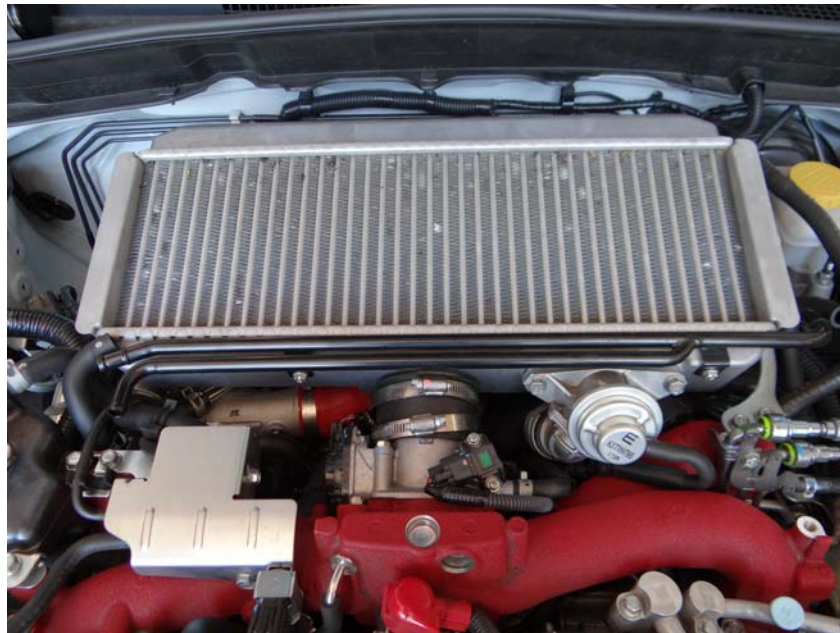
Step 23: Re-install intercooler.
