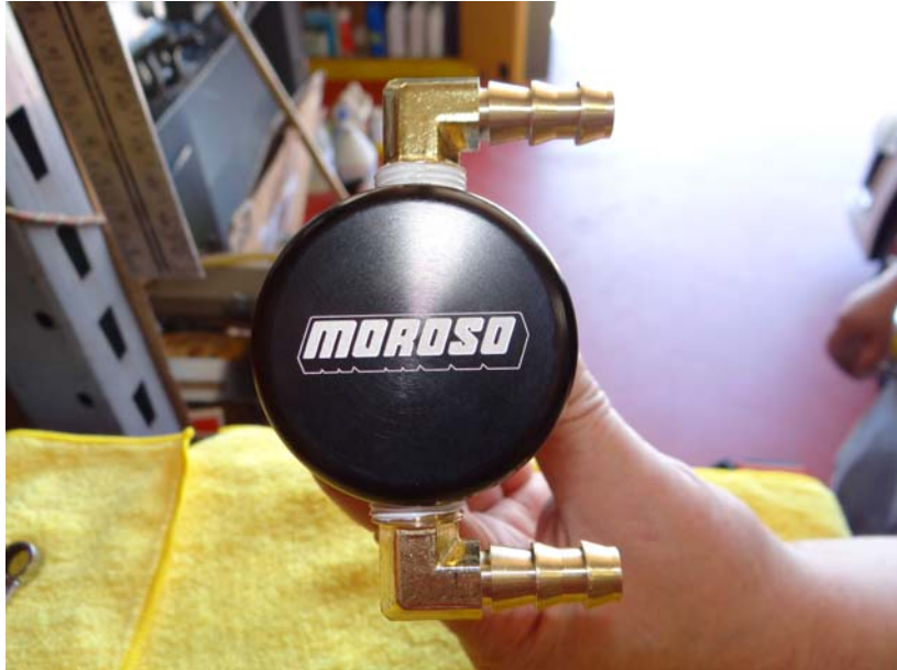
Step 35: Assemble (1) Air Oil Separator as shown using (2) 3/8" barbed fittings using Teflon tape.
