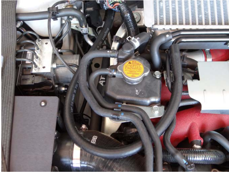
Step 46: Route hose #4 to Air oil separator, mark and trim.
