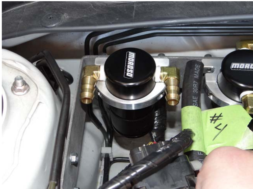
Step 46: Route hose #4 to Air oil separator, mark and trim.
