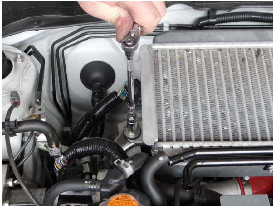
Step 8: Remove intercooler mounting bolts.
