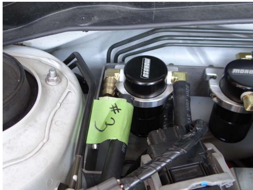
Step 48: Route hose #3 to Air oil separator, mark and trim.
