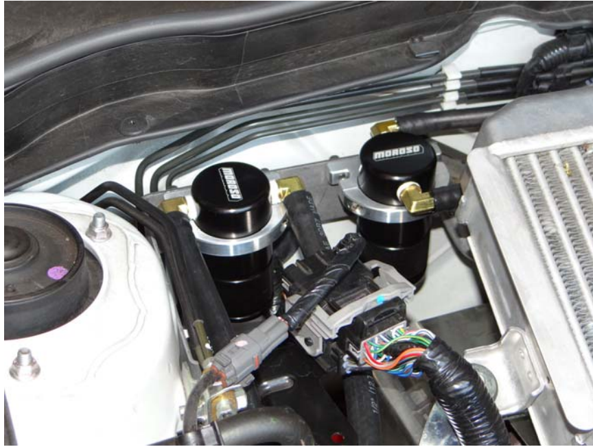
Step 49: Install hose #3 to Air Oil Separator.
