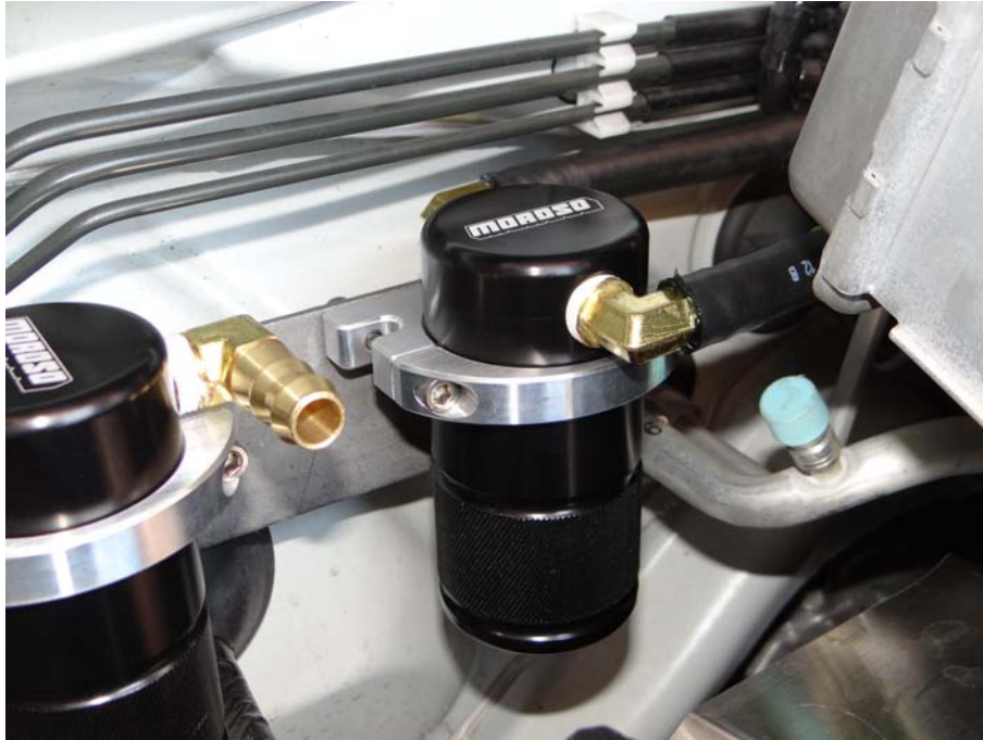
Step 44: Install hose #2 to Air Oil Separator.
