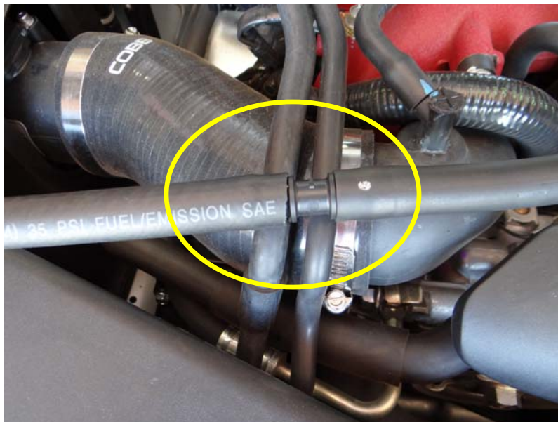
Step 27: Using 32" long 1/2 I.D.hose insert over 1/2" coupling.
