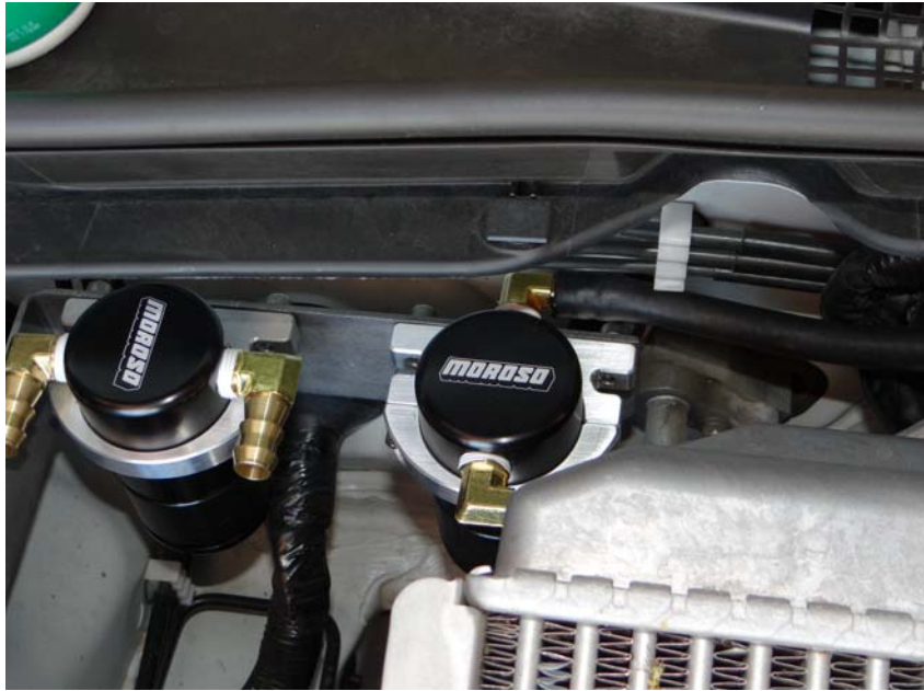
Step 41: Install hose #1 to Air Oil Separator.
