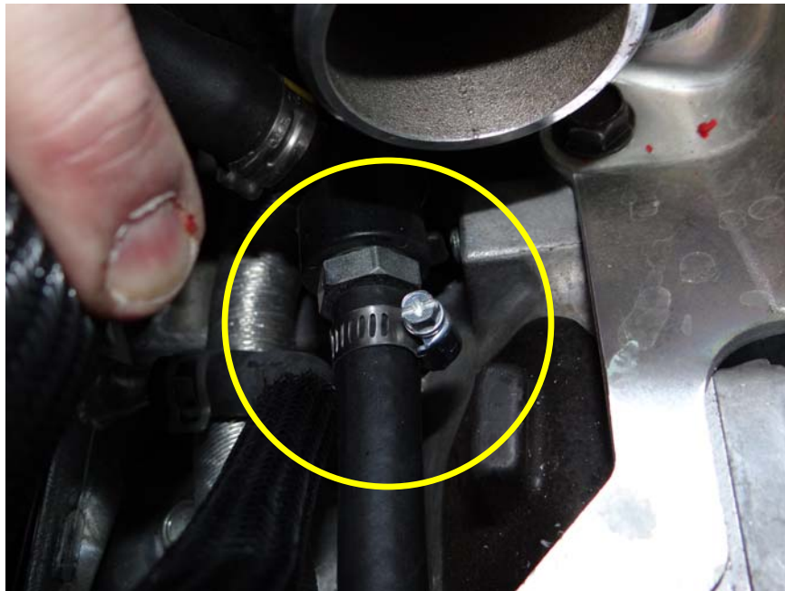
Step 16: Using 36" long 3/8 I.D.hose and clamp insert over PCV line nipple shown.
