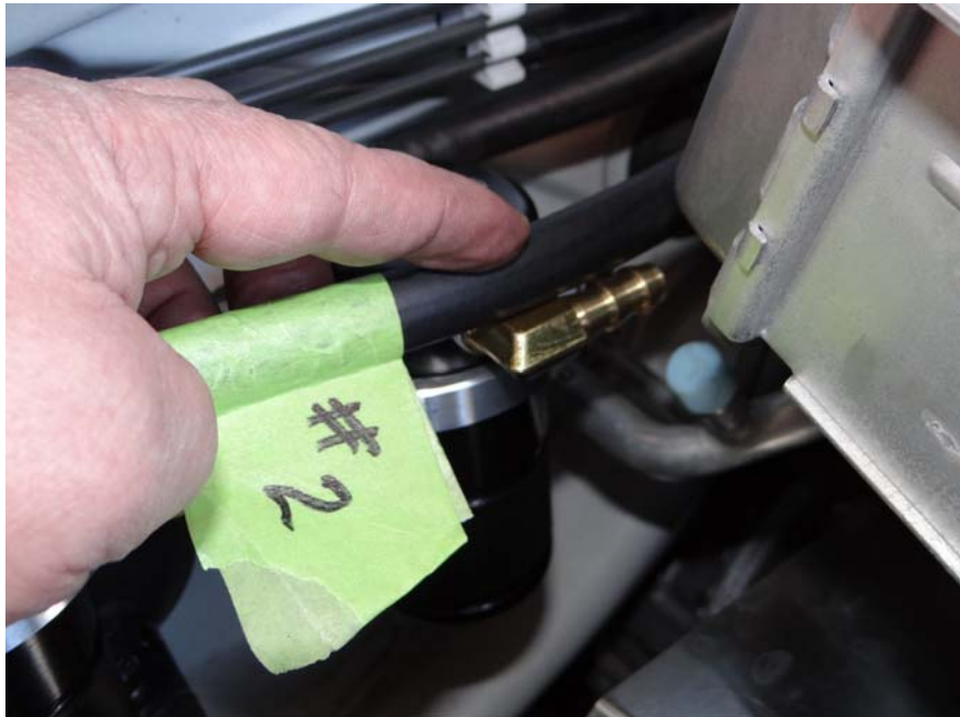
Step 42: Route hose #2 to Air Oil Separator and mark or triming.
