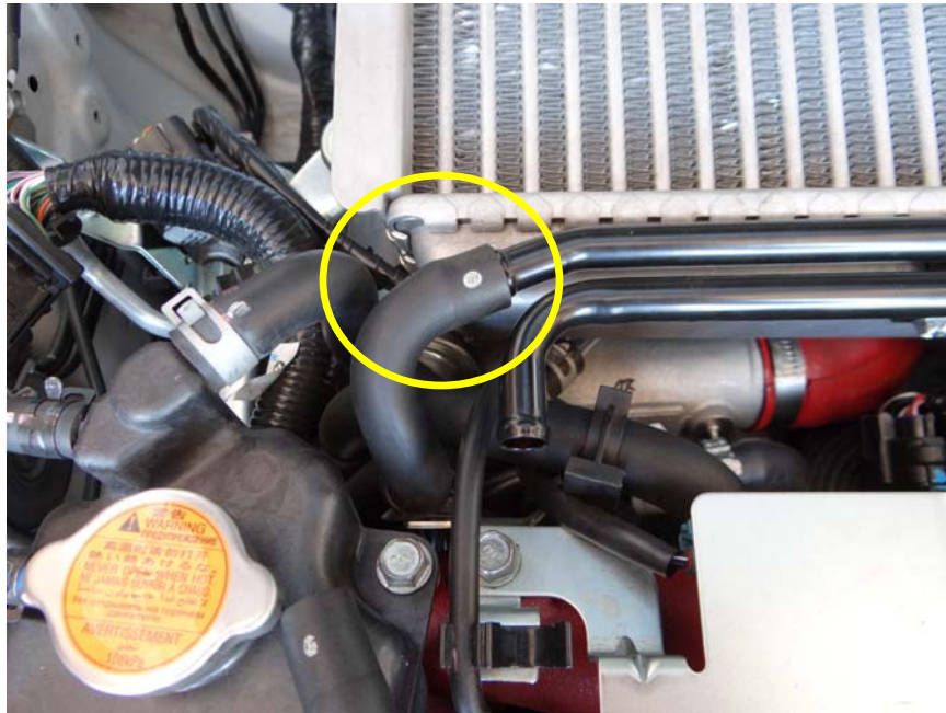
Step 25: Reinstall vacuum line shown to cross over tube on passenger's side.
