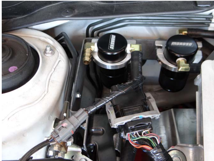
Step 47: Install hose #4 to Air Oil Separator.
