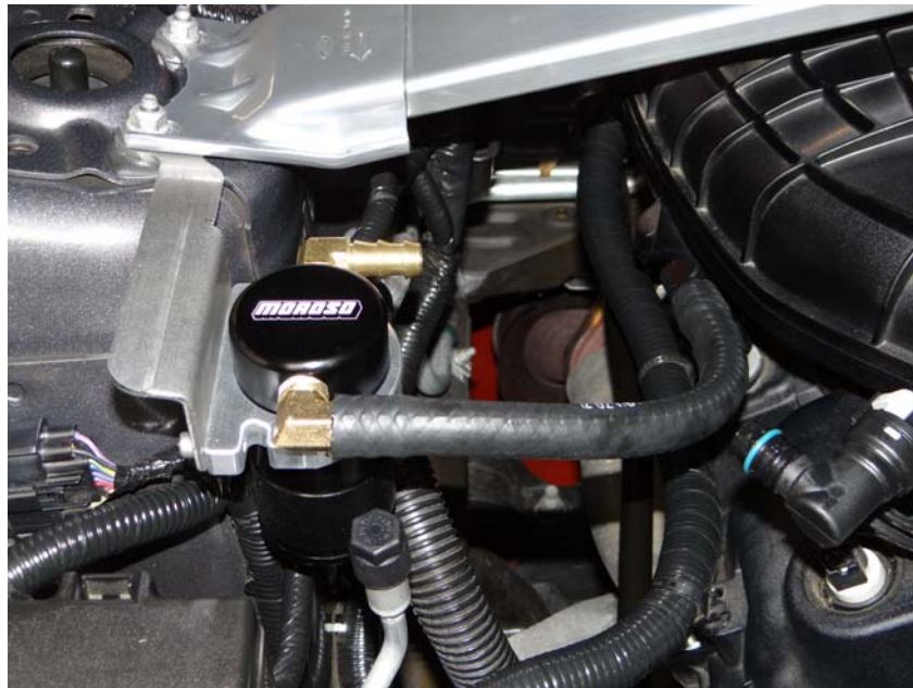
Step 14: Route hose to Air Oil Separator and install.
