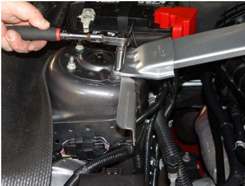
Step 5: All vehicles tighten nut-securing bracket as shown.
