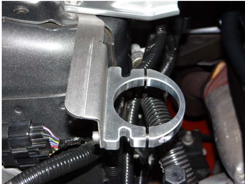
Step 10: Install billet clamp with (2) 1/4-20x5/8 SHCS, do not tighten.
