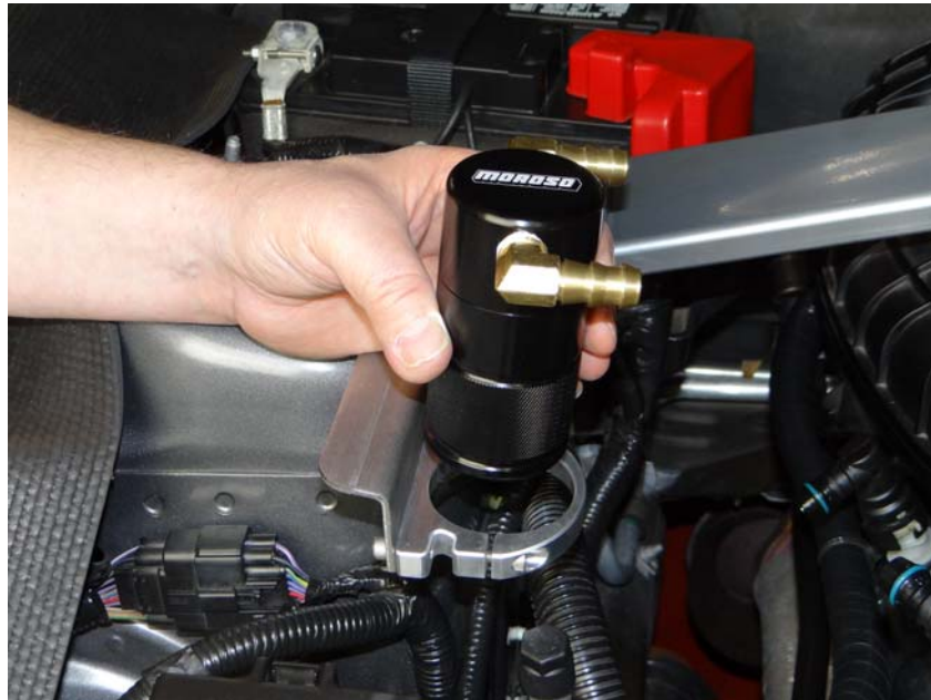
Step 12: Install Air Oil Separator in billet clamp as shown and tighten.
