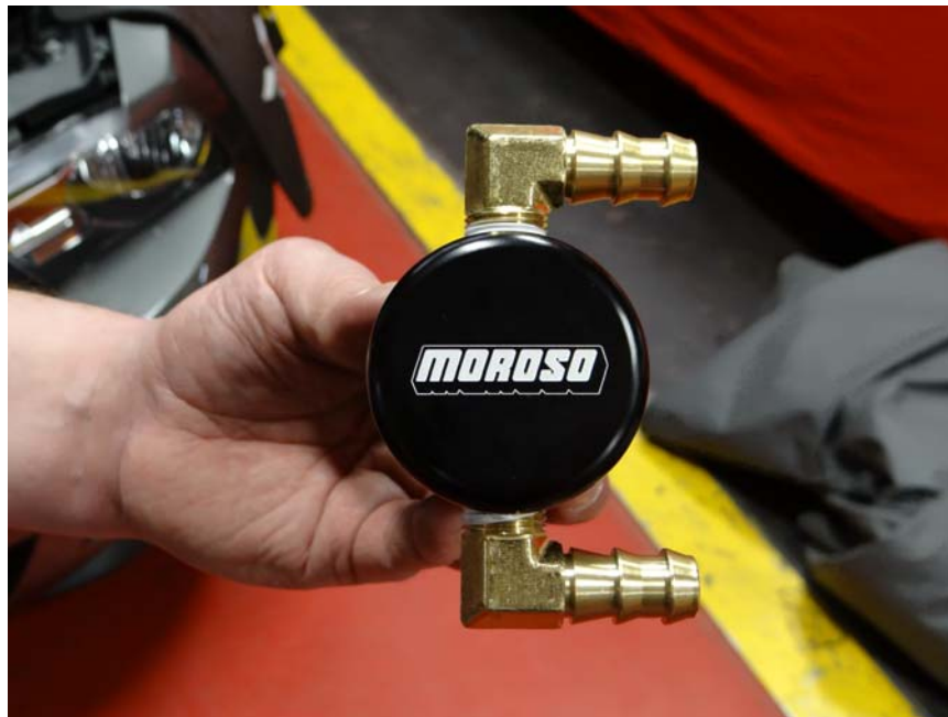
Step 11: Assemble fittings in Air Oil Separator as shown using Teflon tap.
