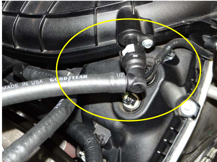
Step 15: Install 8 1/4" long hose to air intake fitting.
