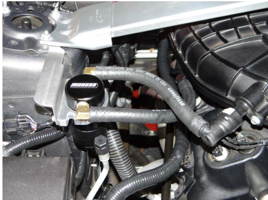
Step 16: Route hose to Air Oil Separator and install.
