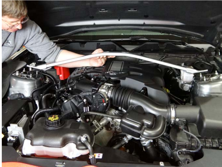
Step 1: If vehicle is equipped with strut tower brace remove.
