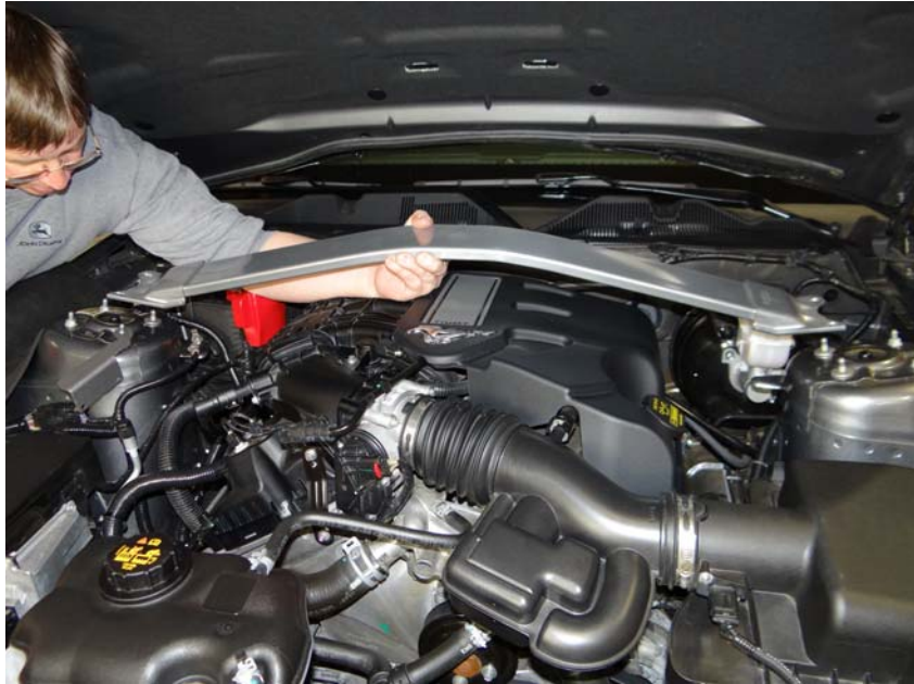
Step 4: Re-install strut tower brace if applicable.
