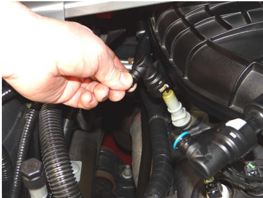
Step 8: Re-install 90 degree fitting in original location.
