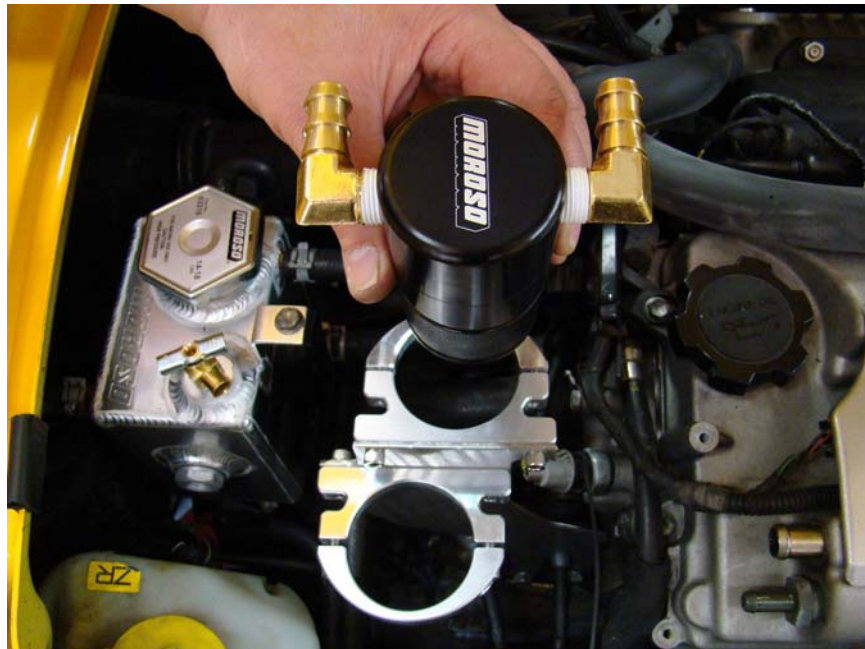
Step 9: Install Air Oil separator with 1/2" 90 degree fittings (towards front of vehicle) in front billet clamp.
