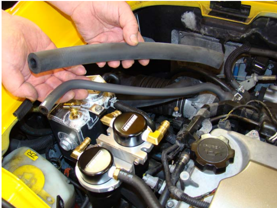
Step 15: Remove outer shell from line previously marked line #1.
