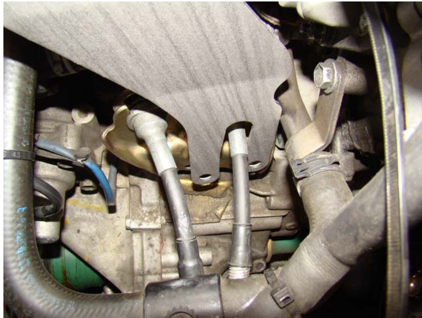
Step 4: Install stainless mounting bracket as shown.
