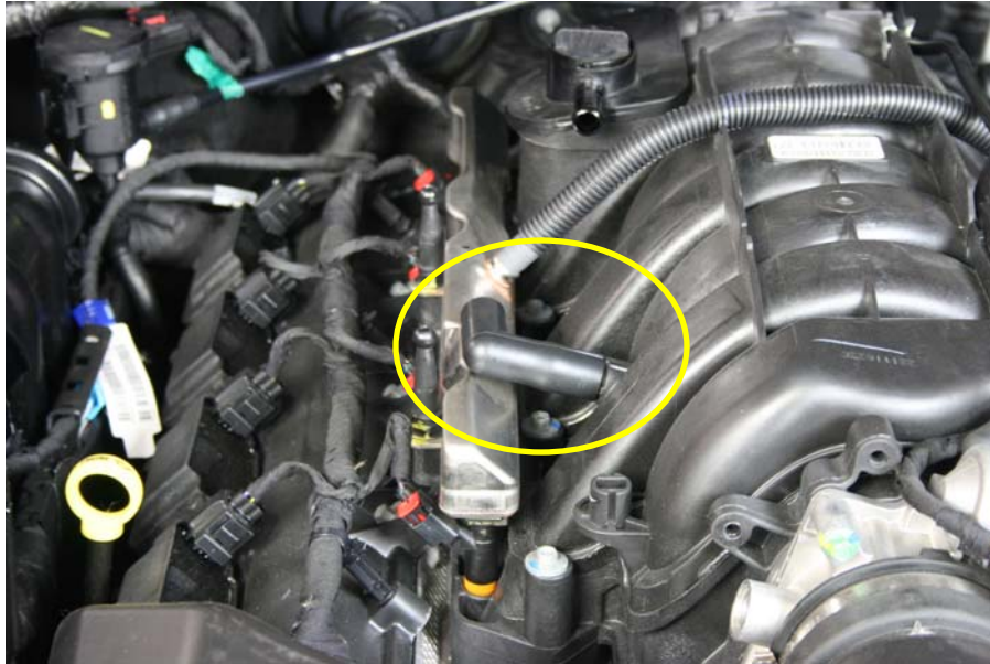
Step 3: Re-install 90 degree elbow in original location.
