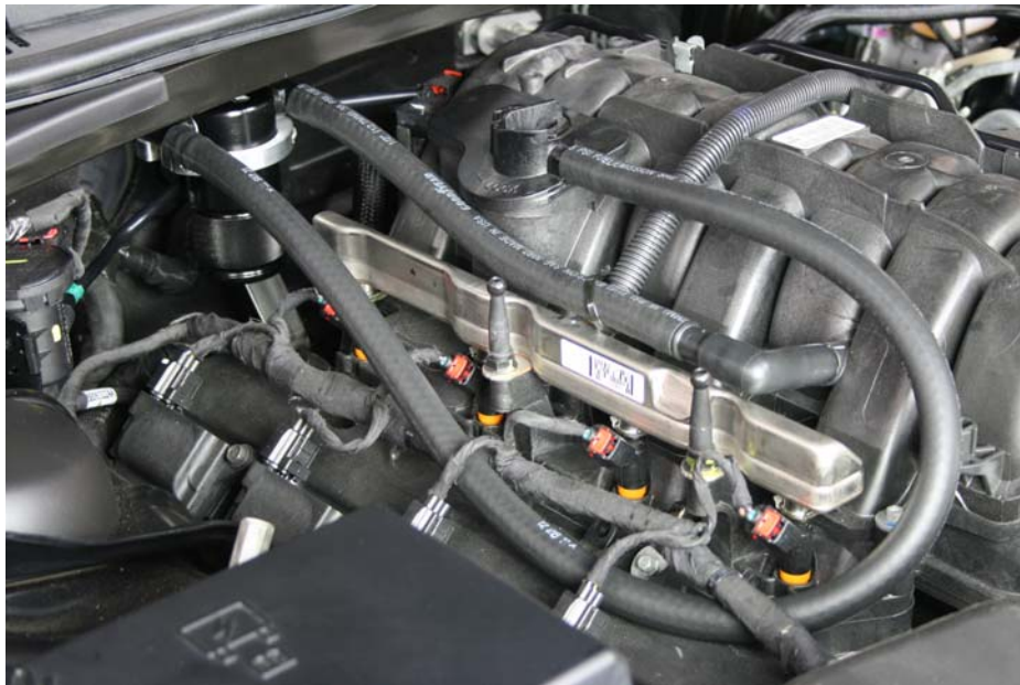
Step 16: Install 36" hose to PCV nipple, route hose to Air Oil Separator, and install hose to barbed fitting.
