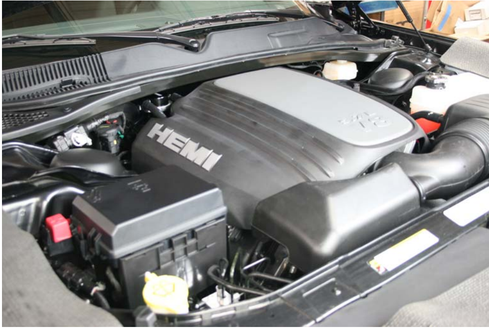
Step 17: Re-install engine cover. Installation complete.
