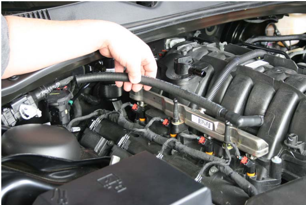
Step 14: Insert 5/8" end of coupling into original 90 degree elbow.
