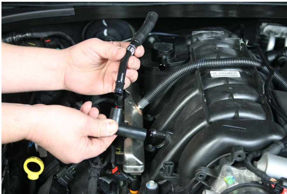
Step 2: Locate and remove PCV line.
