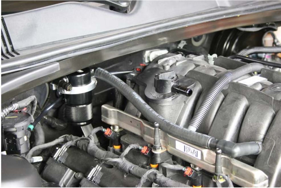
Step 15: Route hose to Air Oil Separator and install hose to barbed fitting shown.
