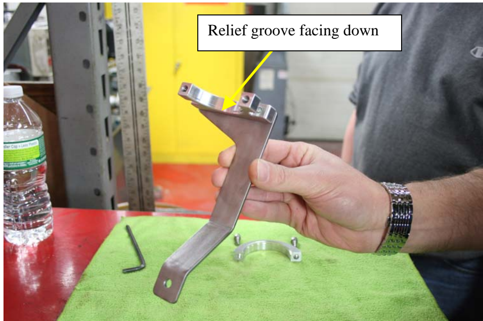
Step 5: Install clamp saddle to stainless mounting bracket using (2) 1/4-20 x 5/8 SHCS.
