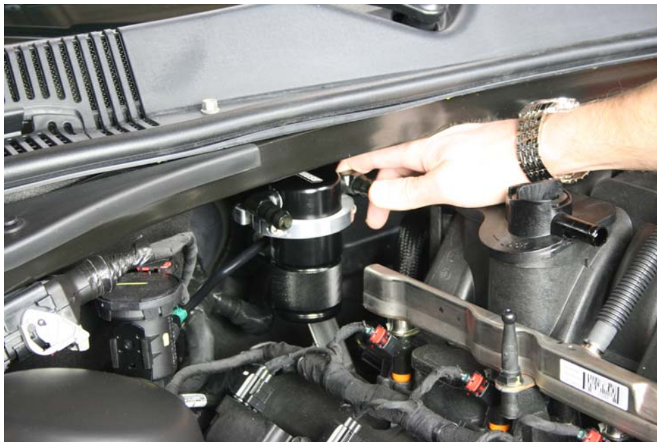
Step 12: Install assembly as shown over stud, and re-install wiring bracket and nut.
