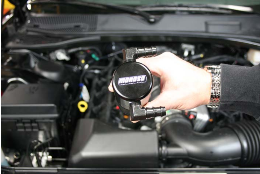
Step 7: Install fittings in Air Oil Separator as shown using Teflon Tape.
