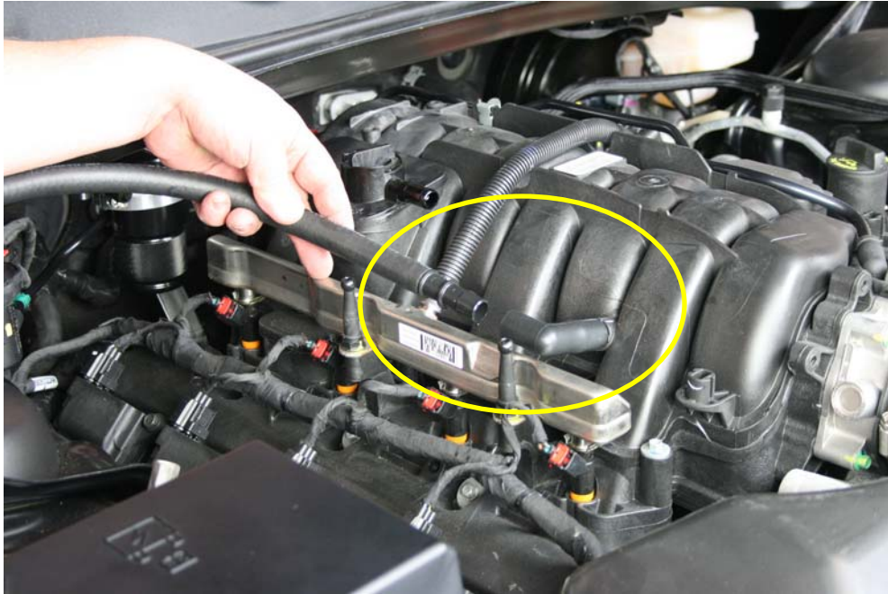
Step 14: Insert 5/8" end of coupling into original 90 degree elbow.
