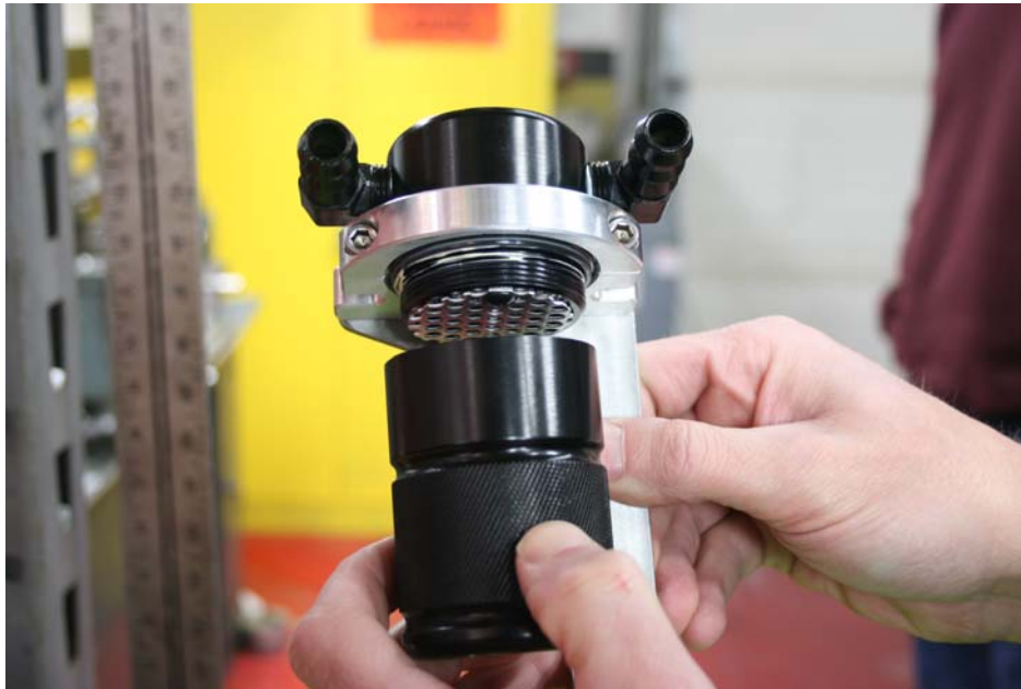
Step 9: Make sure bottom cup can be removed, if not adjust clamp position.
