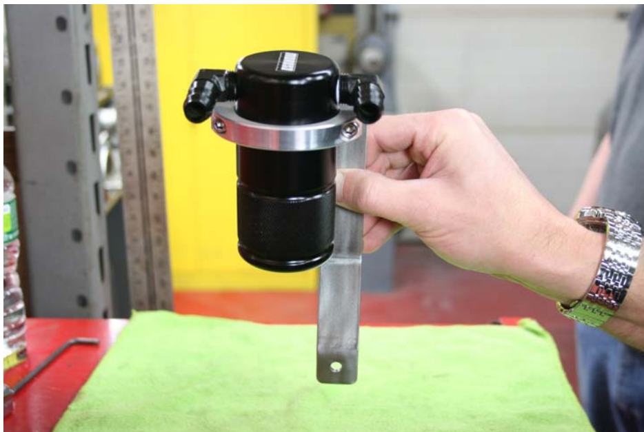
Step 9: Make sure bottom cup can be removed, if not adjust clamp position.
