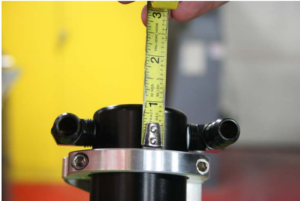
Step 8: Insert Air Oil Separator into billet clamp, measure as shown, leaving 1" to 1 1/8" from top of Air Oil Separator to top of billet clamp.
