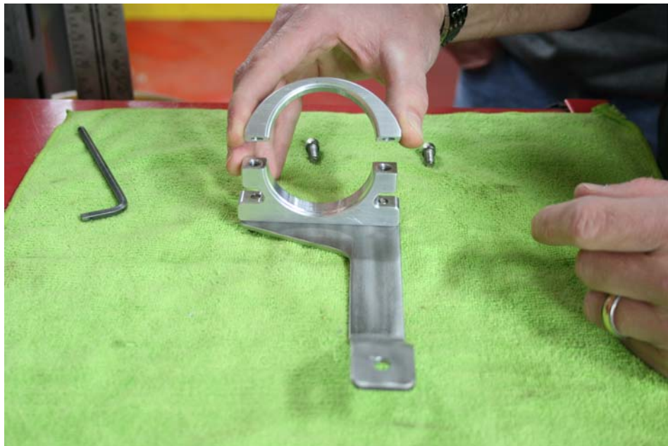
Step 6: Install billet clamp using (2) 1/4-20 x 5/8 SHCS, do not tighten and make sure relief grooves are facing bottom of stainless mounting bracket.
