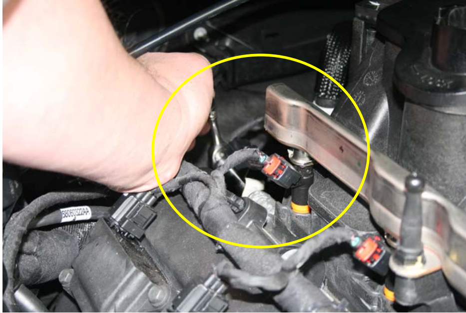
Step 11: Remove nut and wiring bracket.
