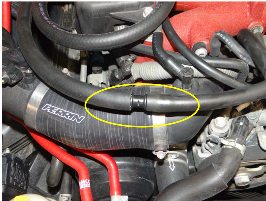
Step 22: Install 2 nd length of 1/2" hose over nylon coupling.
