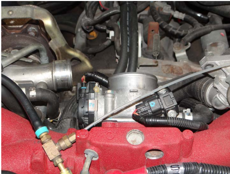
Step 15: Reinstall throttle body with new throttle body gasket supplied with kit.
