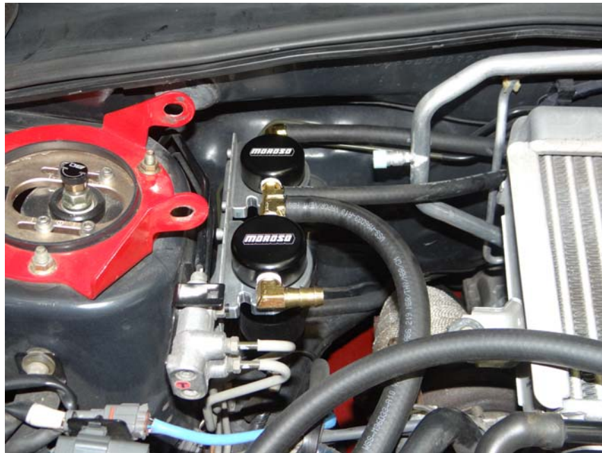
Step 34: Install 1/2" hose labeled #3 to Air Oil separator with 1/2" barbed fittings.
