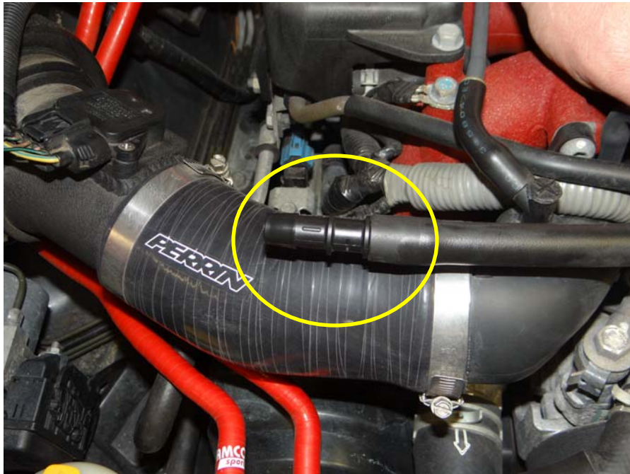
Step 18: Insert nylon coupling into end of breather hose.
