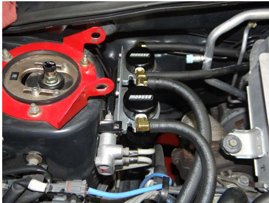
Step 35: Install 1/2" hose labeled #4 to Air Oil separator with 1/2" barbed fittings.
