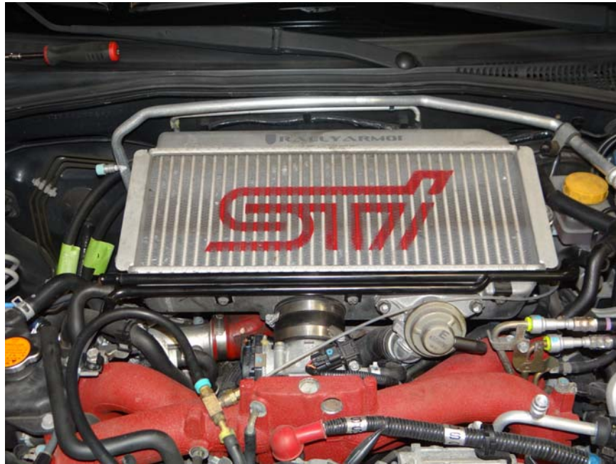
Step 16: Reinstall intercooler.
