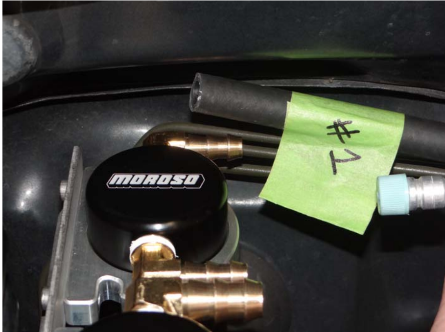
Step 32: Install 3/8" labeled #1 to Air Oil separator with 3/8" barbed fittings.
