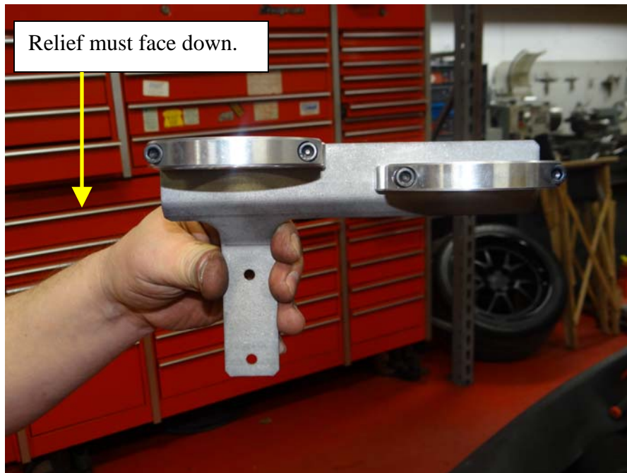
Step 25: Assemble billet clamps to stainless mounting bracket as shown using (4) 1/4-20x5/8 SHCS.
