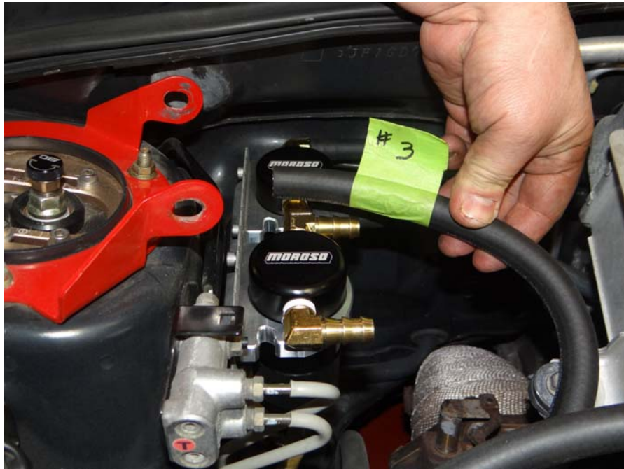
Step 34: Install 1/2" hose labeled #3 to Air Oil separator with 1/2" barbed fittings.
