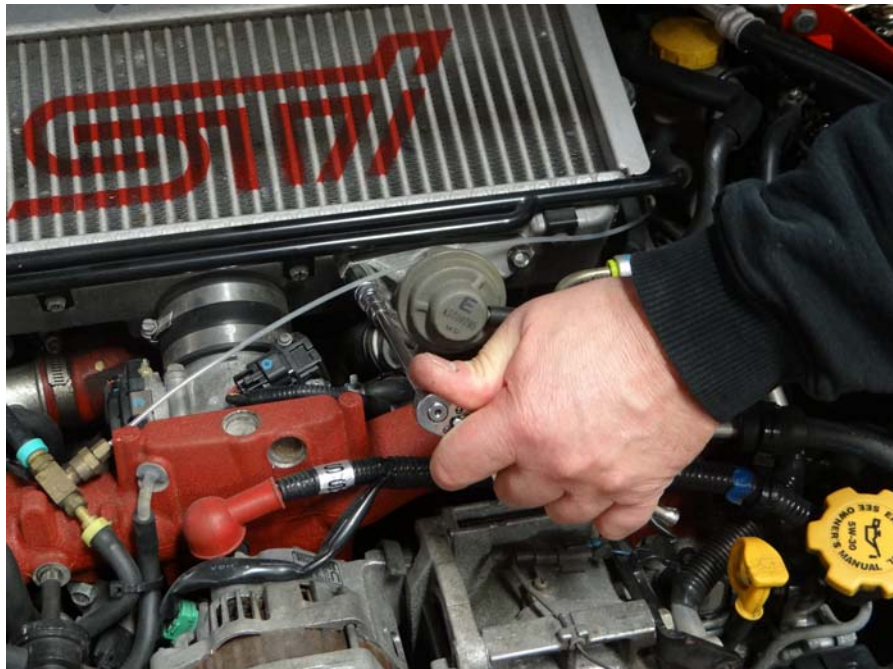
Step 1: Remove By-Pass / Blow-Off Valve from intercooler.
