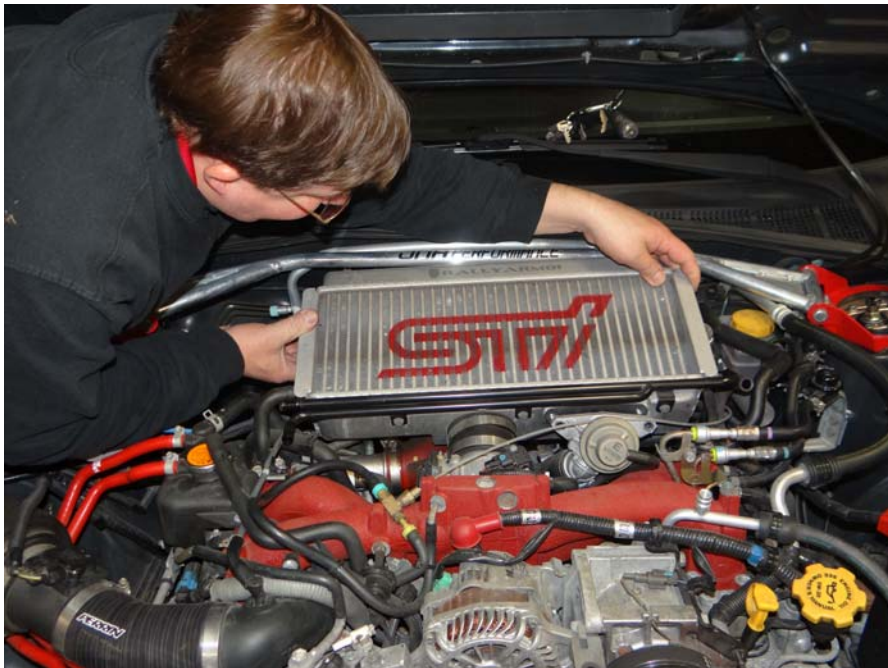
Step 5: Remove intercooler from vehicle.
