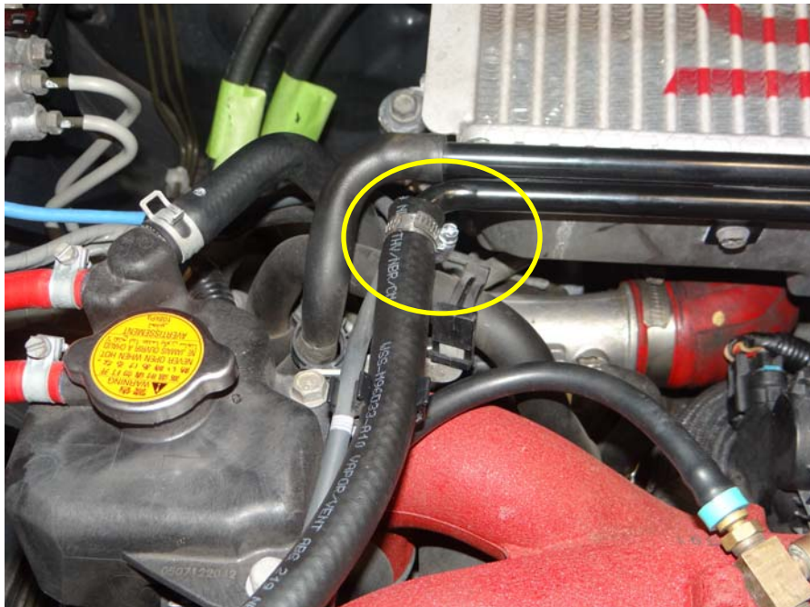
Step 19: Install hose clamp over 1/2" hose and install to crossover tube as shown.
