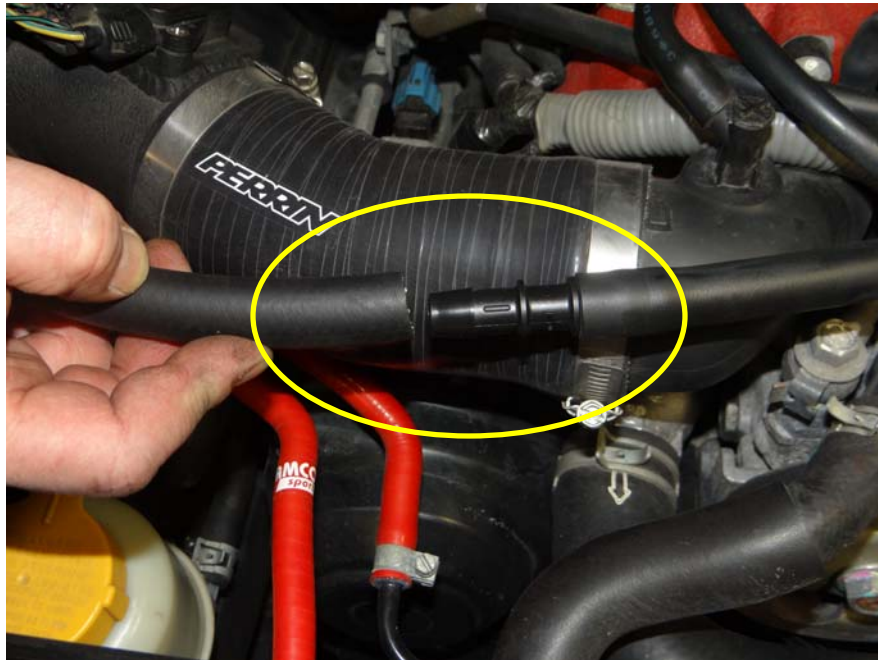
Step 22: Install 2 nd length of 1/2" hose over nylon coupling.
