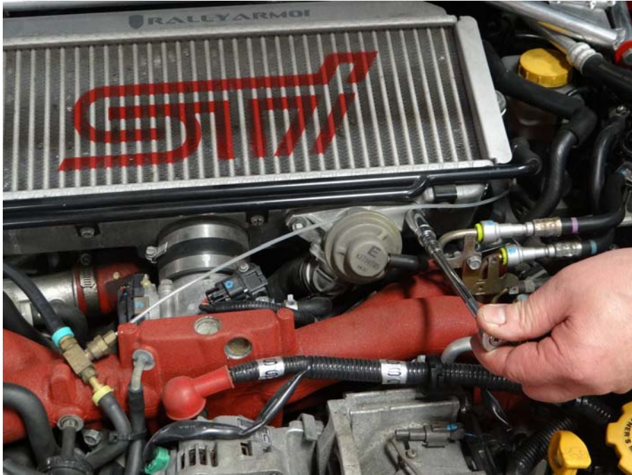
Step 1: Remove By-Pass / Blow-Off Valve from intercooler.
