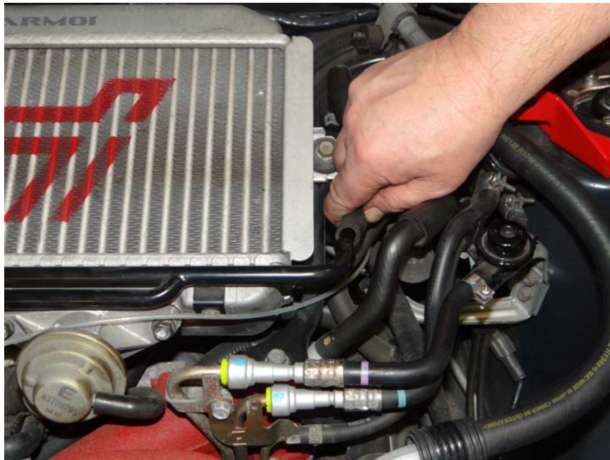
Step 16: Reinstall intercooler.
