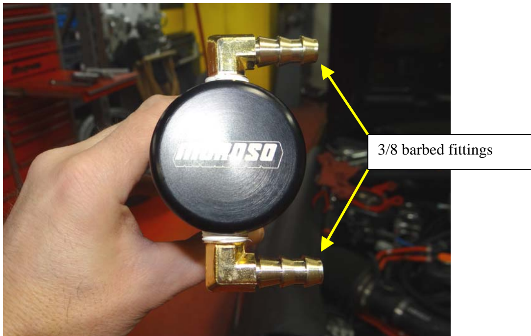
Step 27: Install (2) 3/8 barbed fitting as shown applying Teflon Tape.
