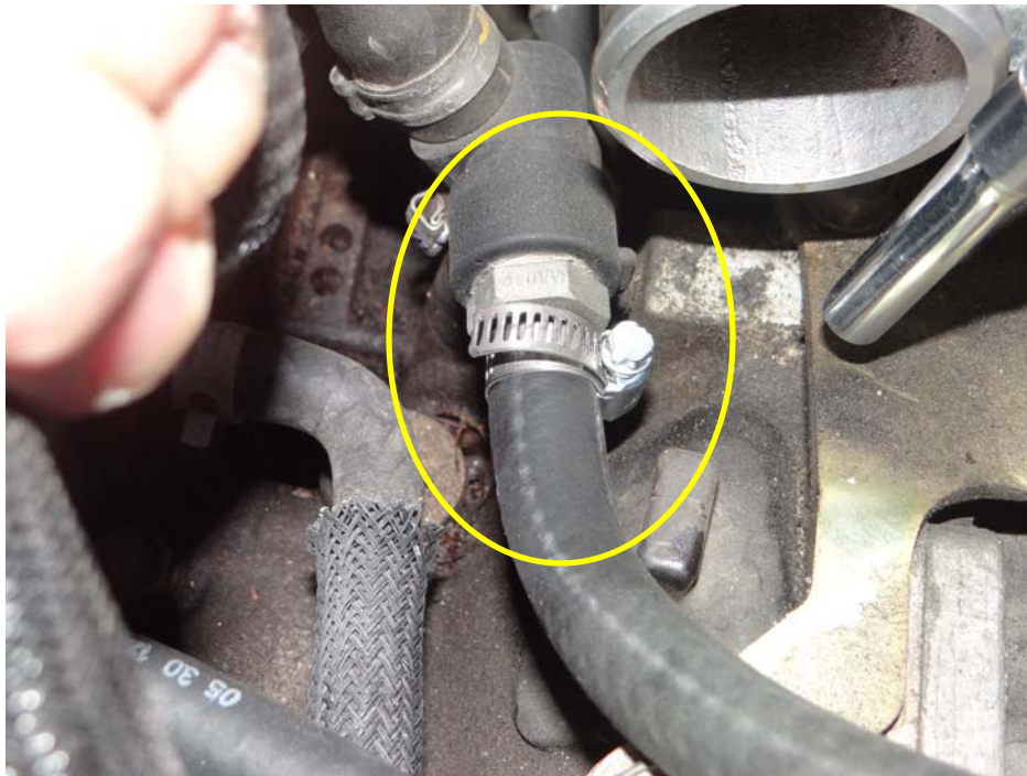
Step 12: Install hose clamp over 2 nd 3/8 hose and install over crank case vent nipple.
