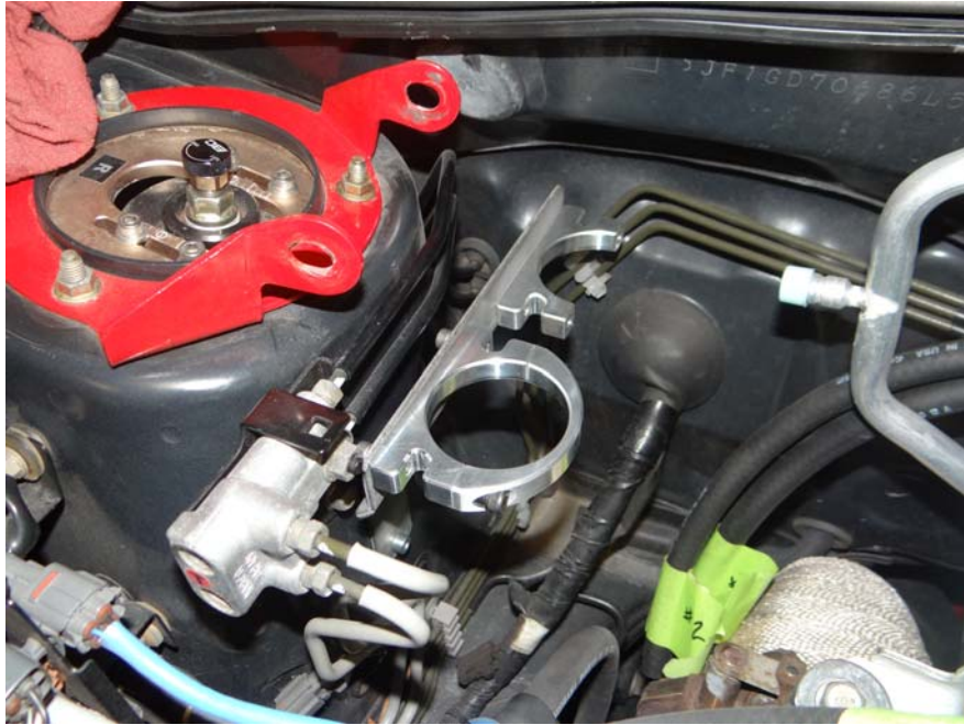
Step 28: Remove rear clamp saddle and insert Air Oil Separator.
