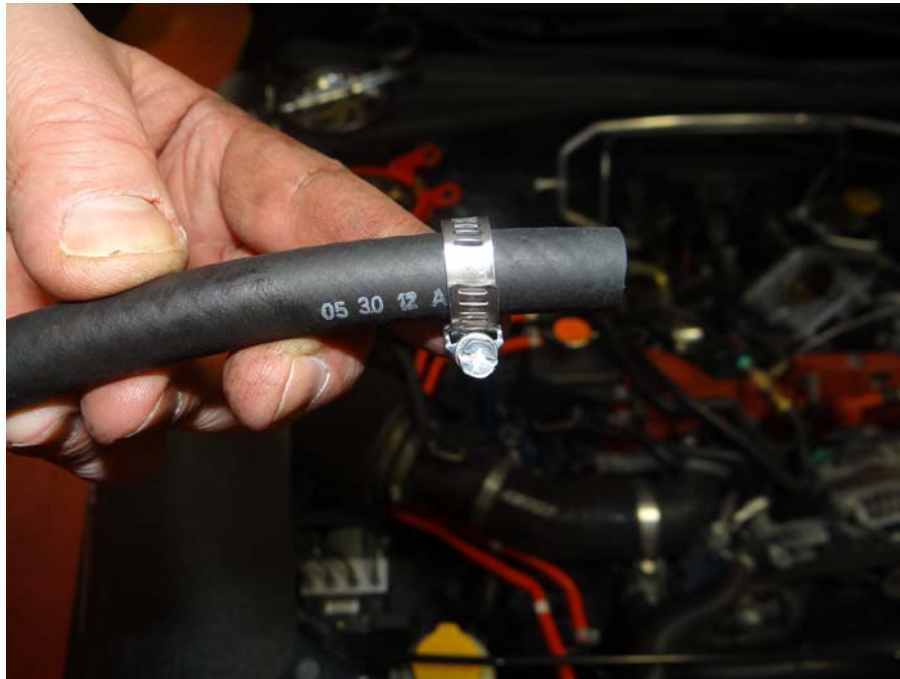
Step 9: Install hose clamp over one end of 3/8 hose.
