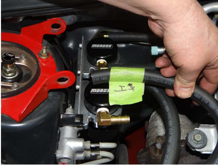
Step 35: Install 1/2" hose labeled #4 to Air Oil separator with 1/2" barbed fittings.
