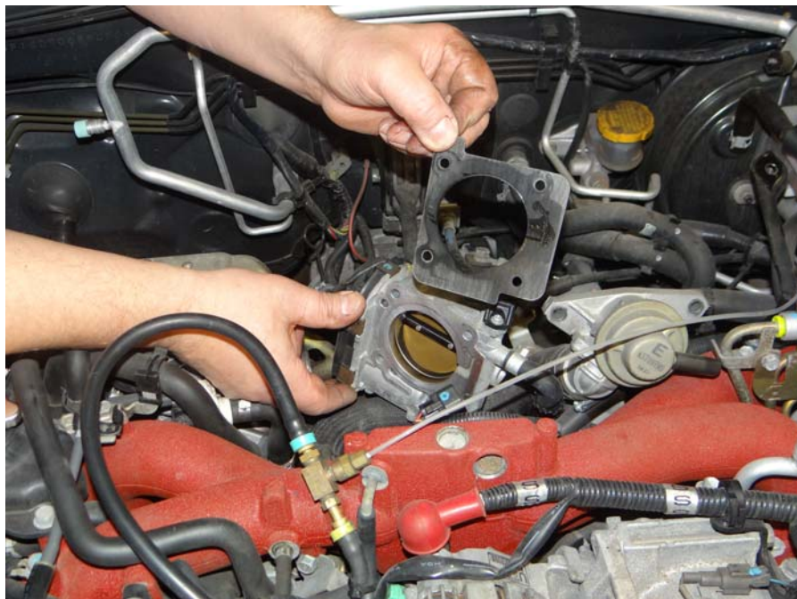
Step 7: Remove and discard throttle body gasket.
