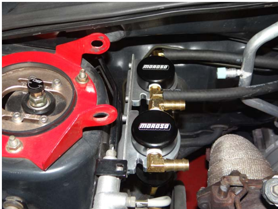
Step 33: Install 3/8" labeled #2 to Air Oil separator with 3/8" barbed fittings.
