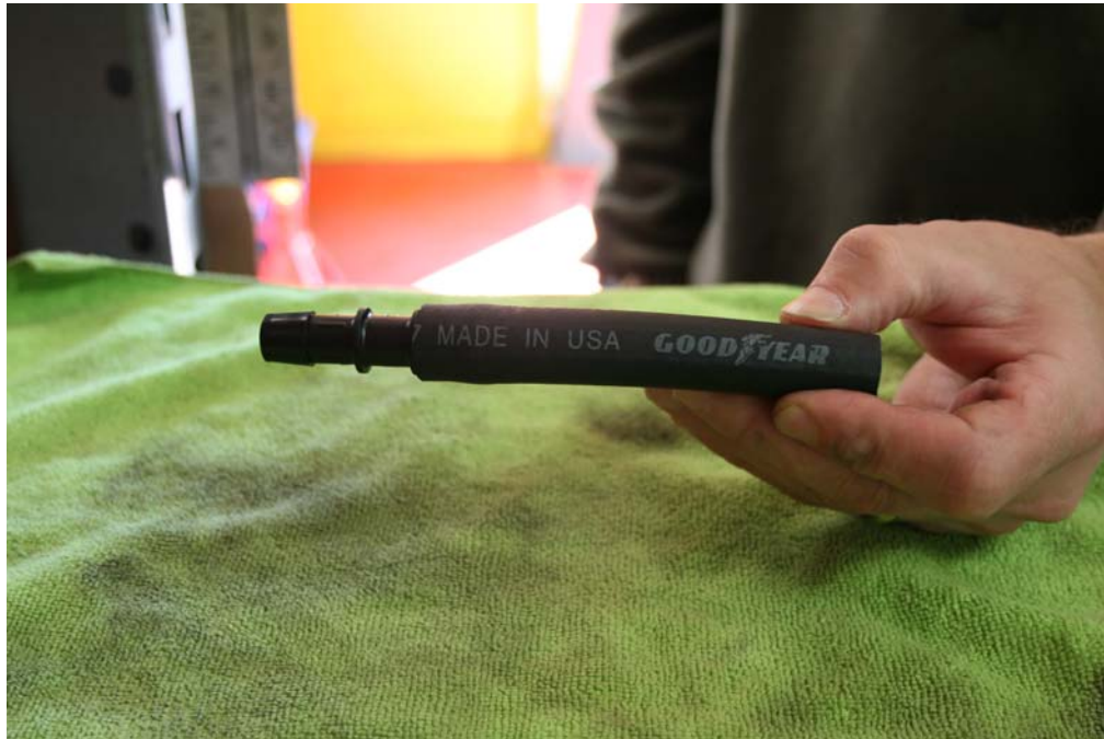
Step 25: Insert ½ coupling into end of 4 ½ long ½ hose.
