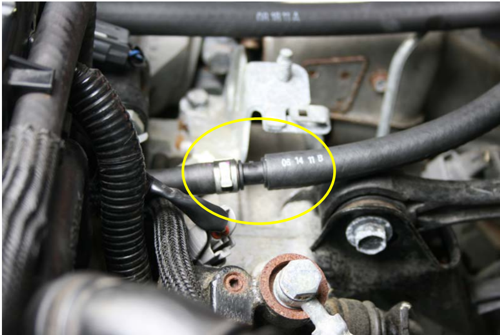
Step 18: Insert other end of 3/8 coupling into crank case vent line and reinstall clamp.
