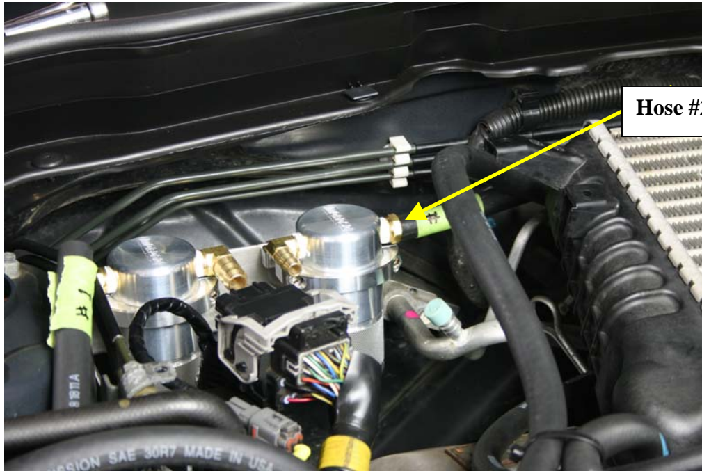
Step 47: Install hose #2 over straight barb as shown.
