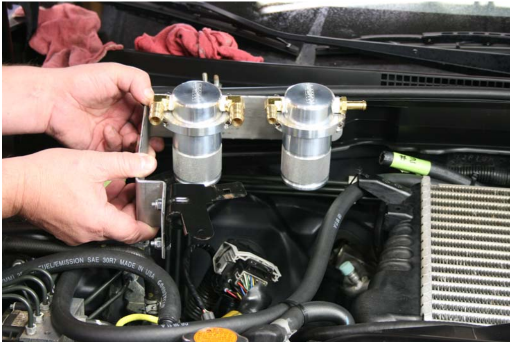
Step 44 Install Air Oil Separator assembly s shown using stock bracket hardware.
