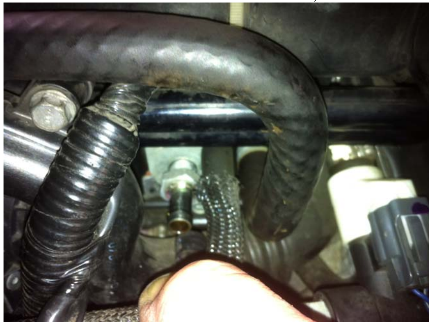
Step 15; Locate crank case vent line running between block and throttle body. (This line is locate on back side of block)
