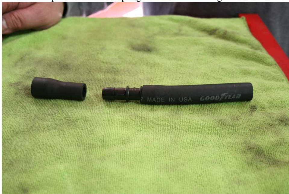
Step 26: Insert ½ side of line previously cut off in step 24 as shown.
