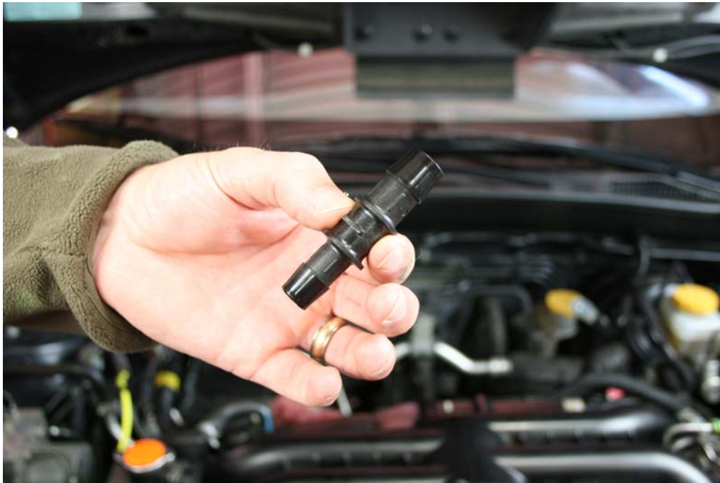
Step 8: Locate 1/2 to 5/8 coupling in kit.
