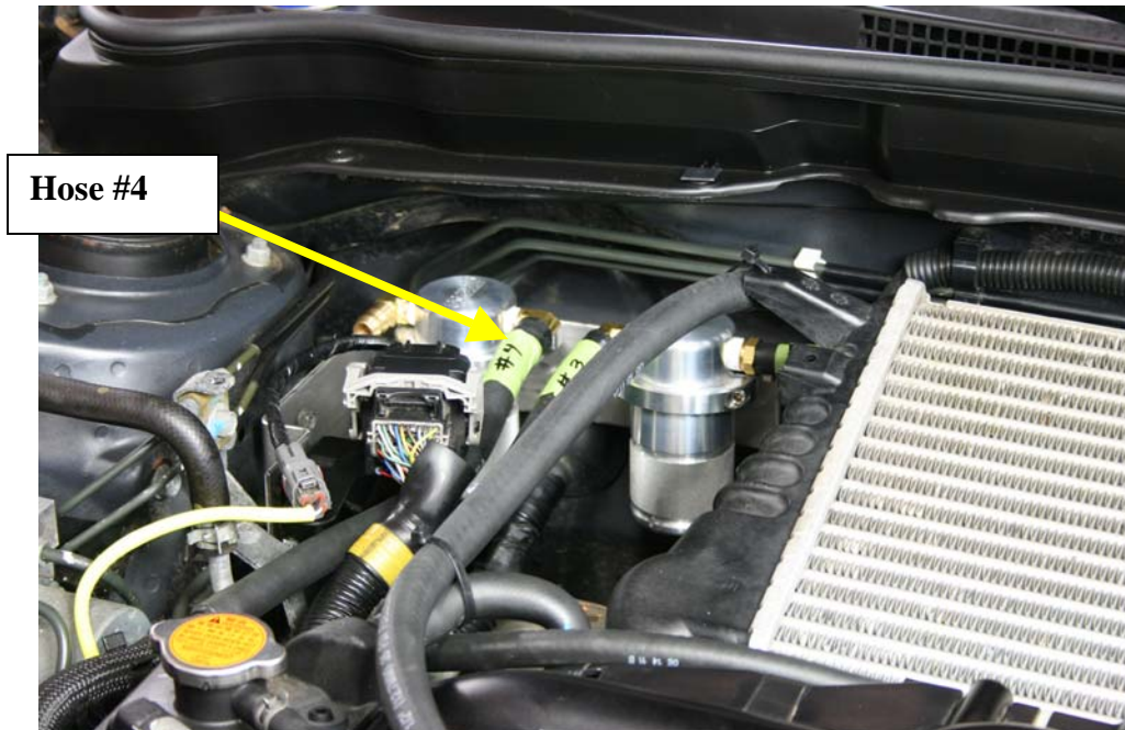
Step 50: Route hose #4 from valve cover crossover hose assembly to 1/2" 90 degree barb.
