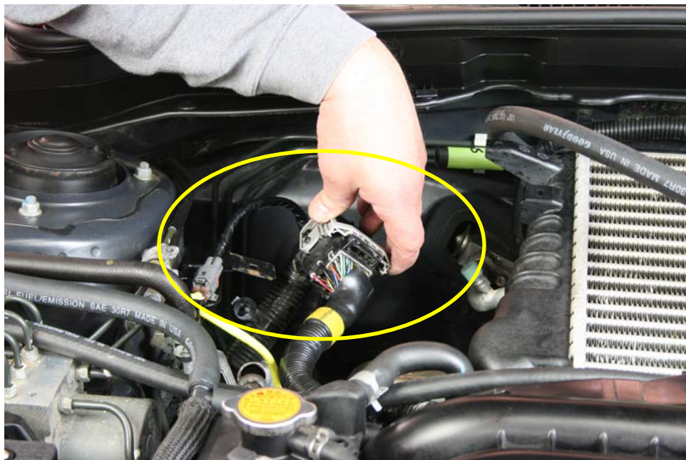
Step 35: Remove wire harness plug as shown from mounting bracket. (Locking tab on under side of harness plug)
