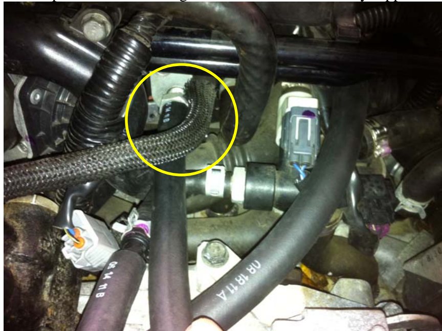
Step 20: Insert 31" long 3/8 hose over throttle body nipple.
