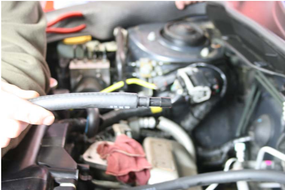
Step 17: Insert 3/8 coupling into one end of 21" long 3/8 hose. For Technical Assistance, call Moroso's Tech Line (203)-458-0542, 8:30am-5:00pm Eastern Time MOROSO PERFORMANCE PRODUCTS, INC.
