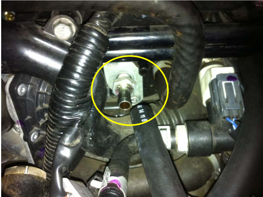
Step 20: Insert 31" long 3/8 hose over throttle body nipple.
