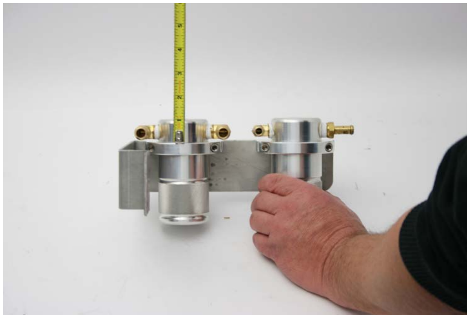
Step 42: Assemble barbed fittings into Air Oil Separators using Teflon tape and insert into billet clamps 1" from top of Air Oil Separator to top of billet clamp.
