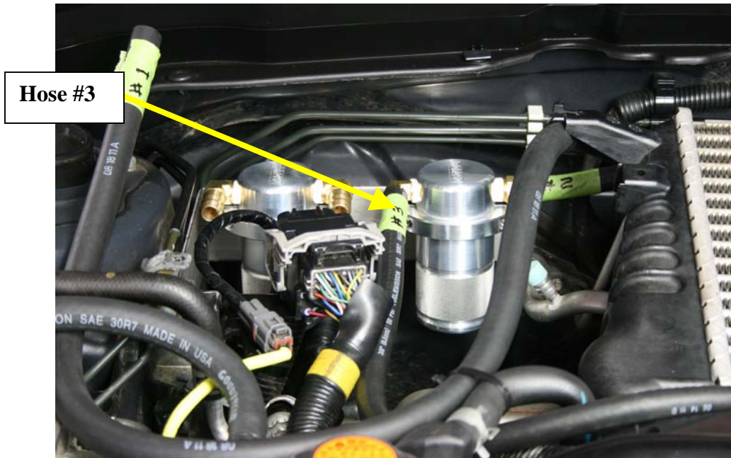
Step 49: Route hose #3 to Air Oil Separator as shown and install over 3/8" 90 degree barb.
