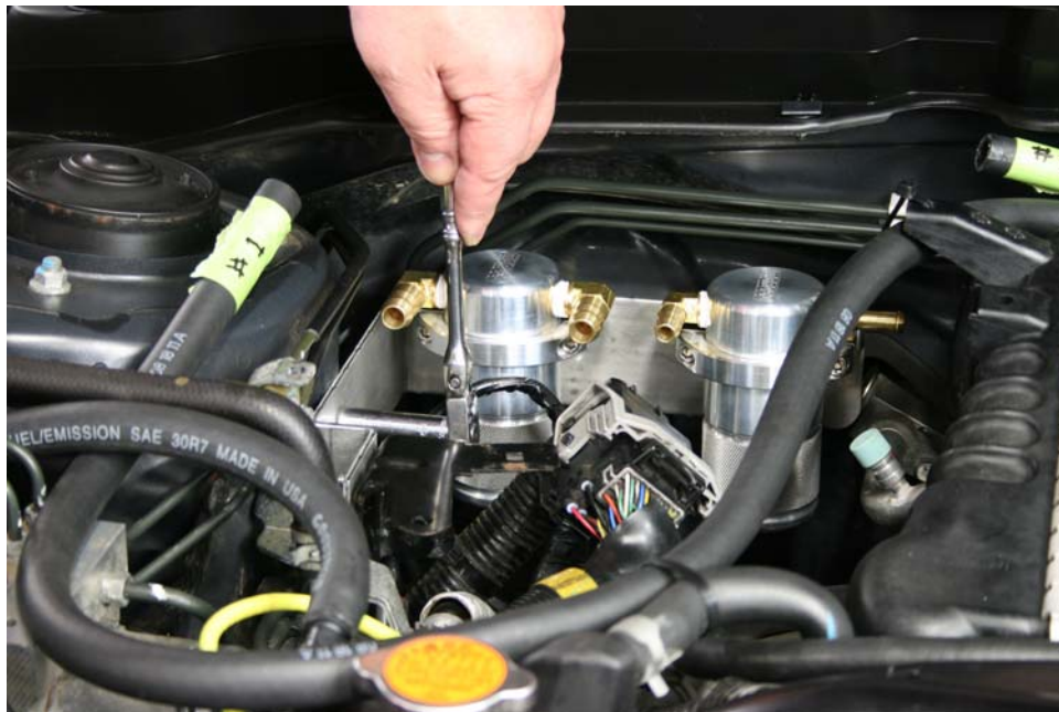
Step 44 Install Air Oil Separator assembly s shown using stock bracket hardware.
