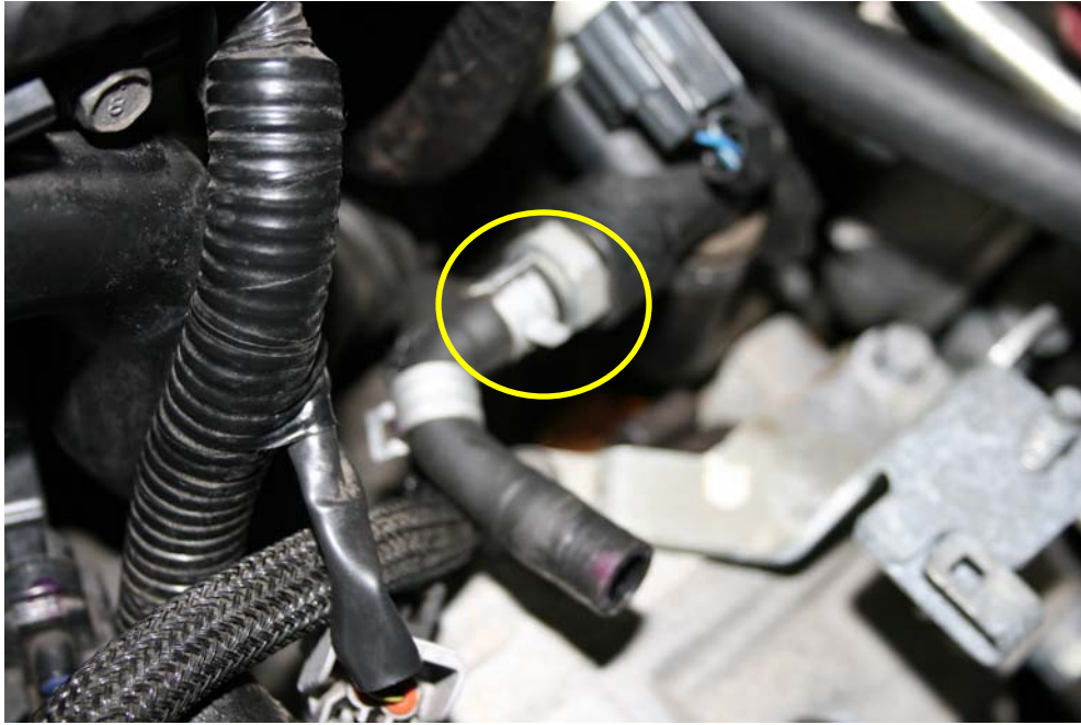
Step 16: Loosen clamp and turn crank case vent line back towards firewall.
