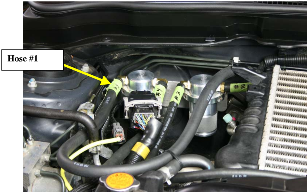
Step 51: Route hose # 1 to Air Oil Separator as shown and install over 1/2" 90 degree barb.
