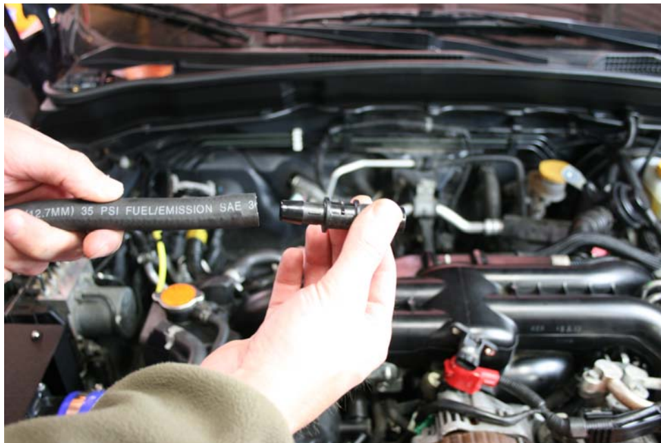
Step 9: Insert 1/2 side of coupling into one end of 58" long 1/2 hose.
