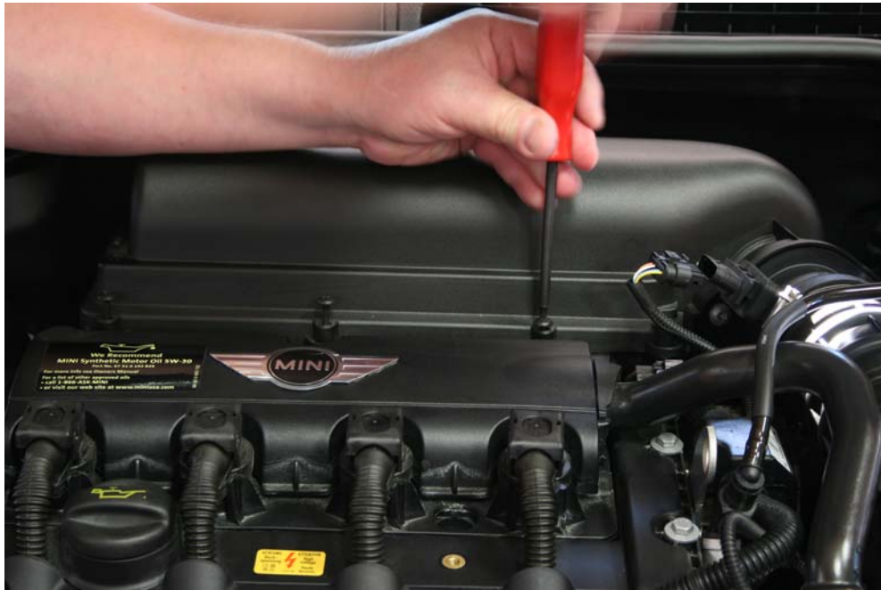
Step 3: Unscrew / Remove air box mounting hardware.
