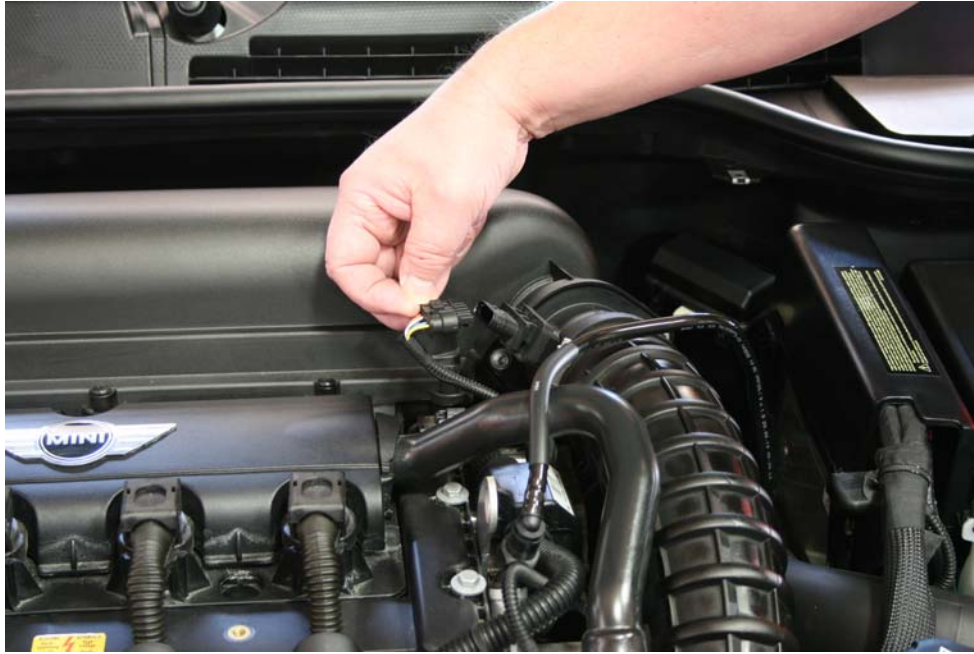
Step 1: Remove mass airflow sensor plug.
