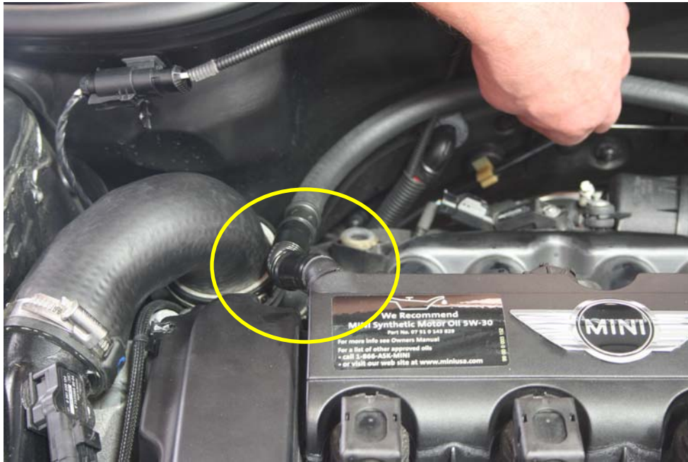
Step 23: Using Fitting / hose assembly from step 19 (With straight end) re-install fitting over valve cover nipple.
