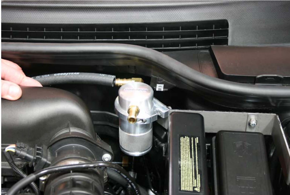
Step 36: Route valve cover hose to Air Oil Separator and install hose over 90 degree barbed fitting.
