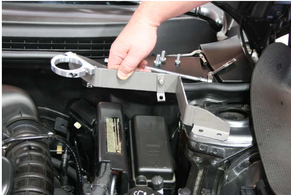
Step 32: Install mounting bracket with (2) 8mm x 20mm HHCS and (1) 6mm x 20mm HHCS
