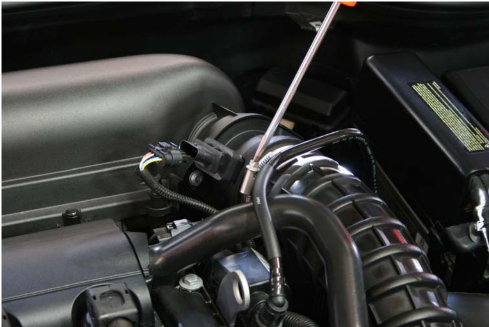
Step 2: Loosen air intake tube clamp.
