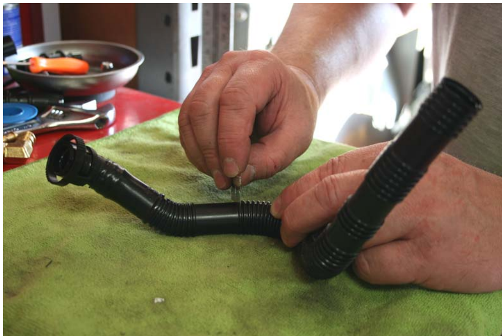
Step 17: Cut valve cover end of PCV line as shown.
