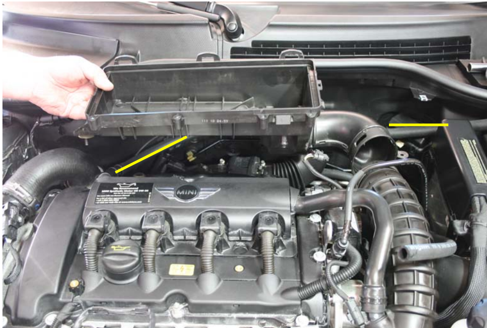
Step 24: Route hose as shown and re-install air box.
