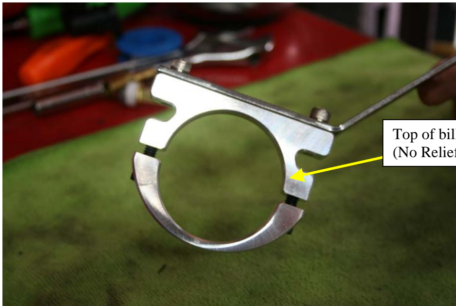
Step 28: Assemble billet clamp and billet clamp assembly to stainless mounting bracket, using (4) 1/4 x 20 x 5/8 SHCS.
