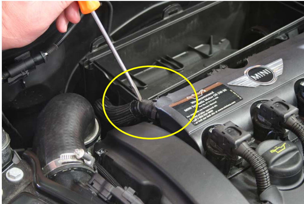
Step 7: Remove PCV line from valve cover.
