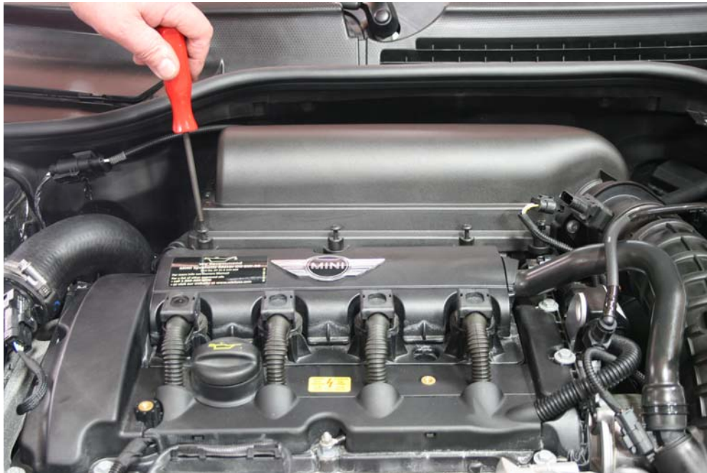
Step 26: Re-install air box top and mass airflow sensor plug.
