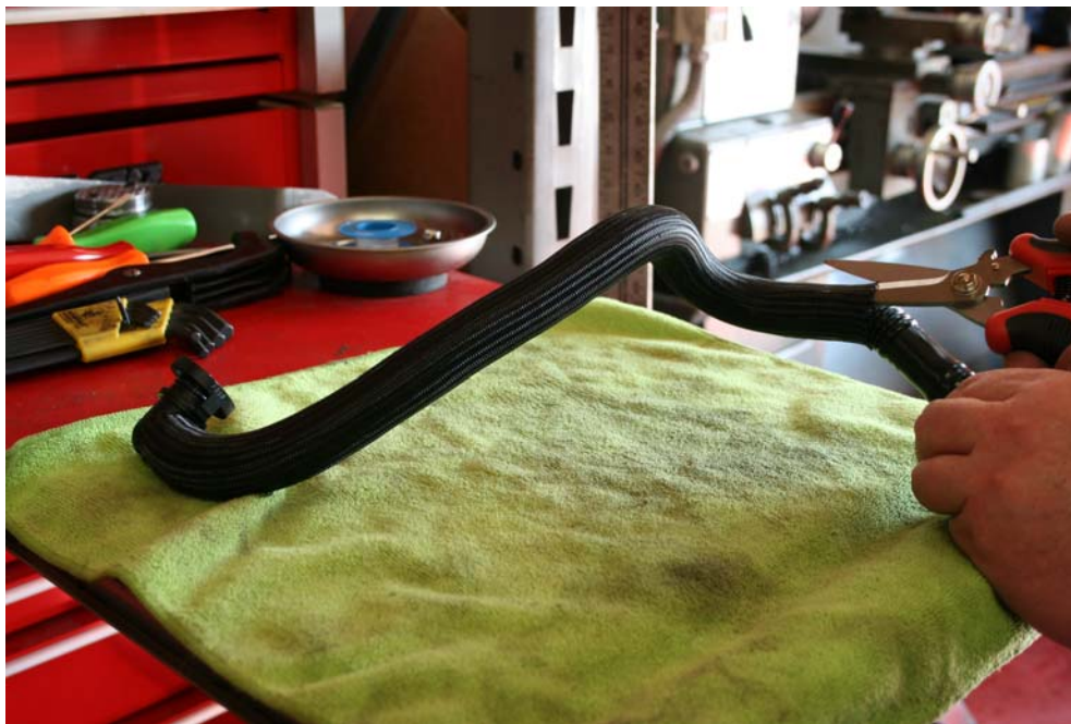
Step 12: Cut outer wrapping from PCV line as shown.
