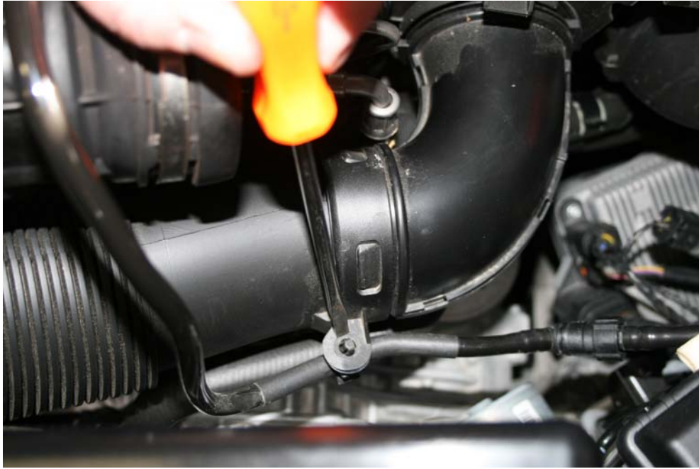
Step 6: Remove vacuum line from air intake tube as shown.
