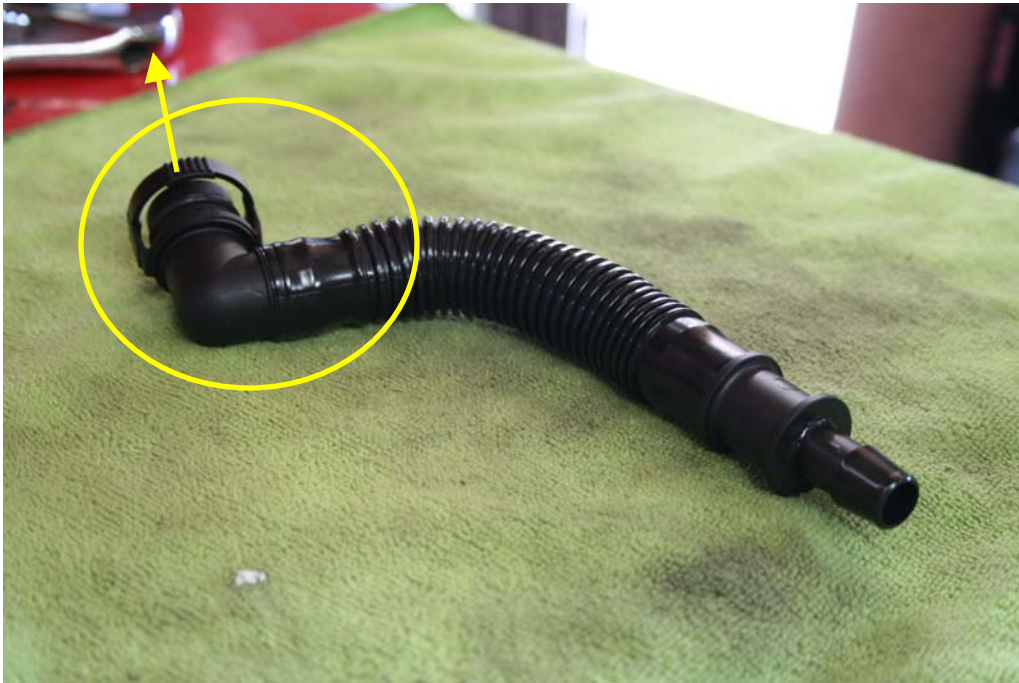
Step 15: Twist fitting 180 degrees as shown.
