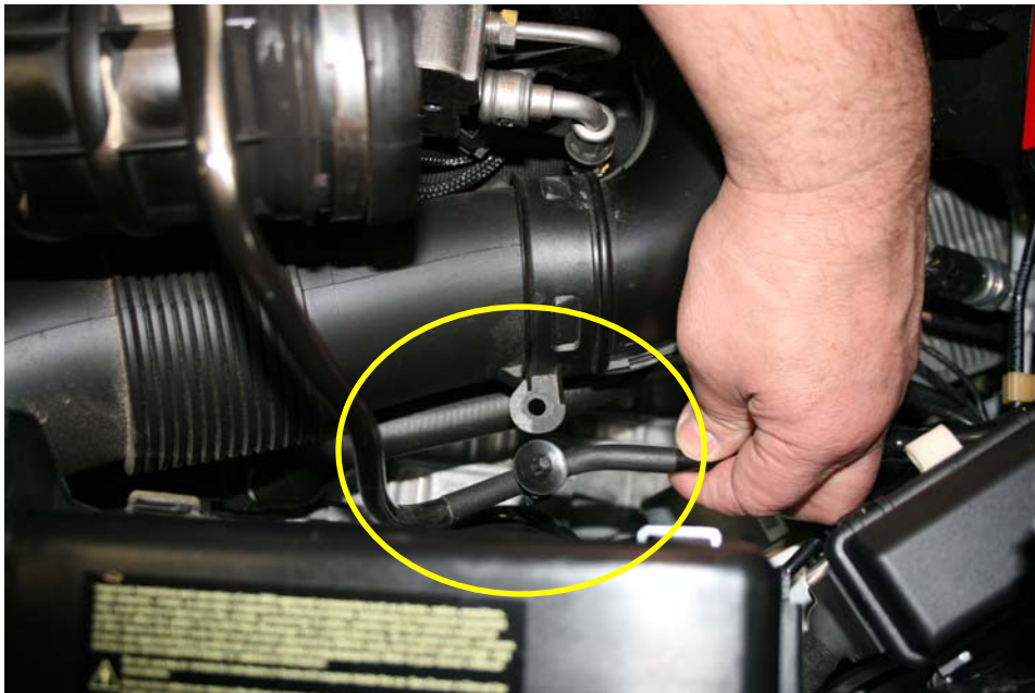
Step 6: Remove vacuum line from air intake tube as shown.
