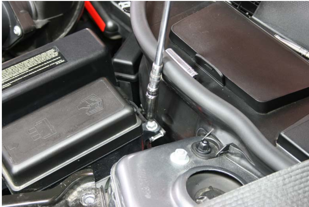
Step 31: Remove fuse box mounting bolt.
