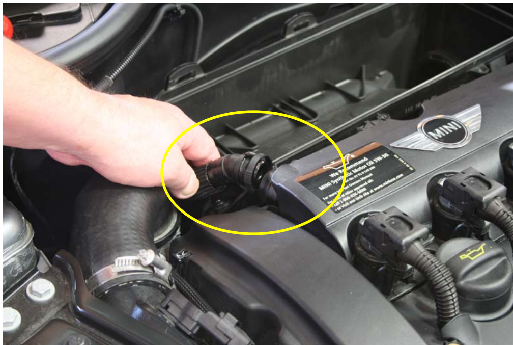
Step 7: Remove PCV line from valve cover.
