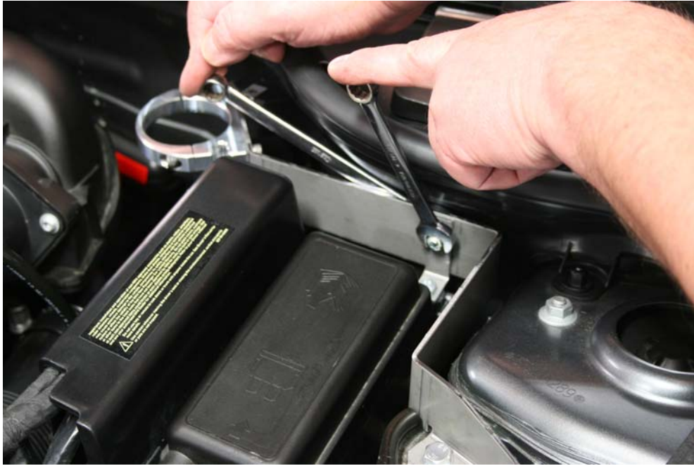
Step 33: Tighten fuse box tab hardware.
