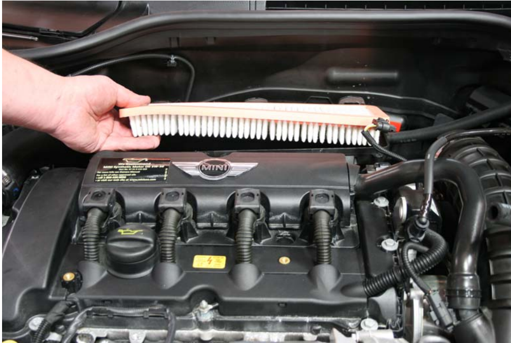
Step 25: Re-install air filter.
