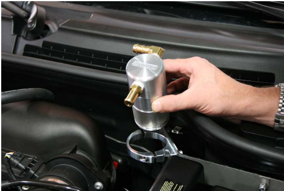
Step 34: Install Air Oil Separator into billet clamp with 90 degree barb facing passenger side of vehicle.
