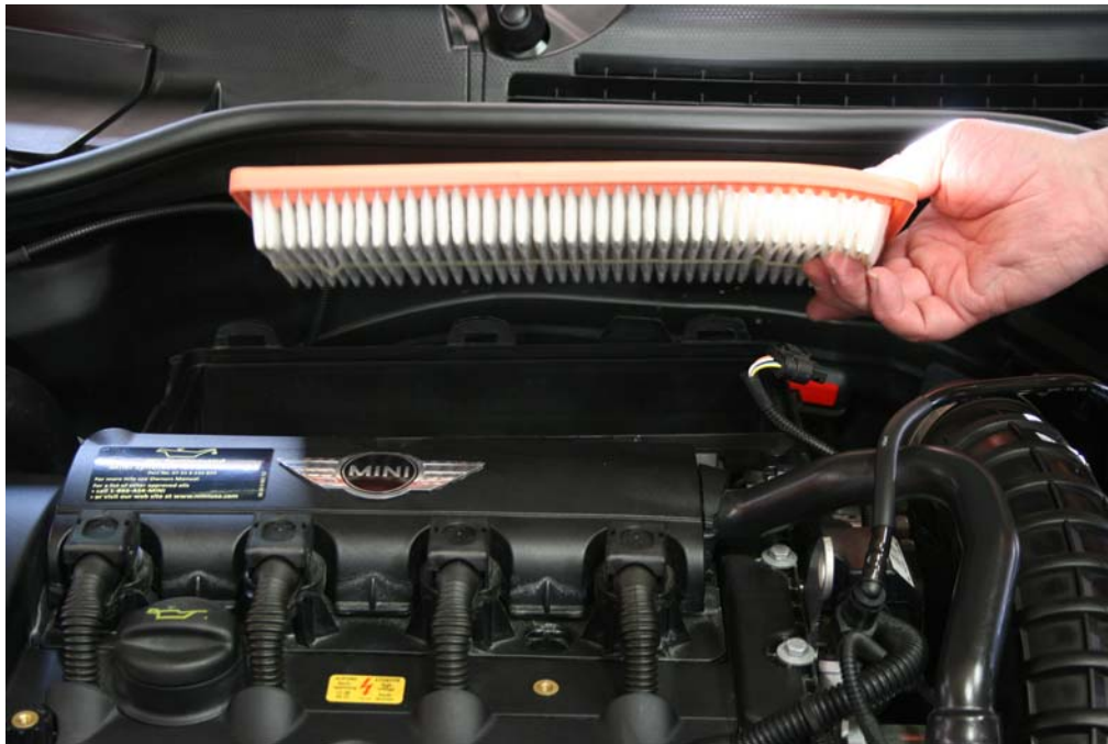
Step 5: Remove air filter.
