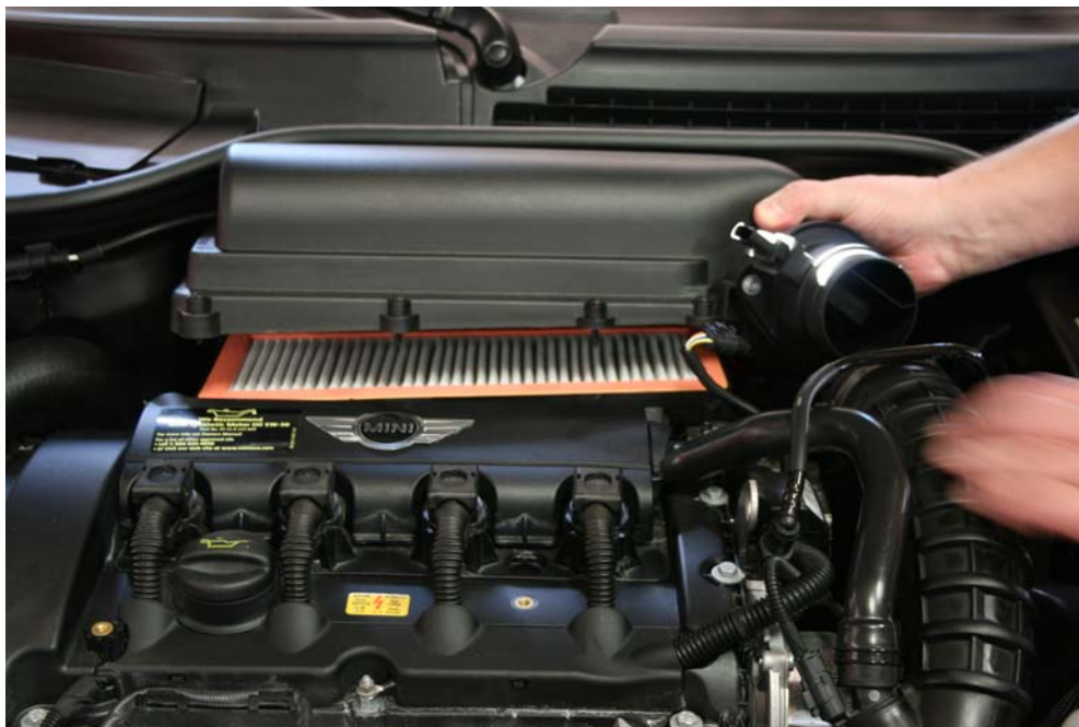
Step 4: Remove air box top from vehicle.
