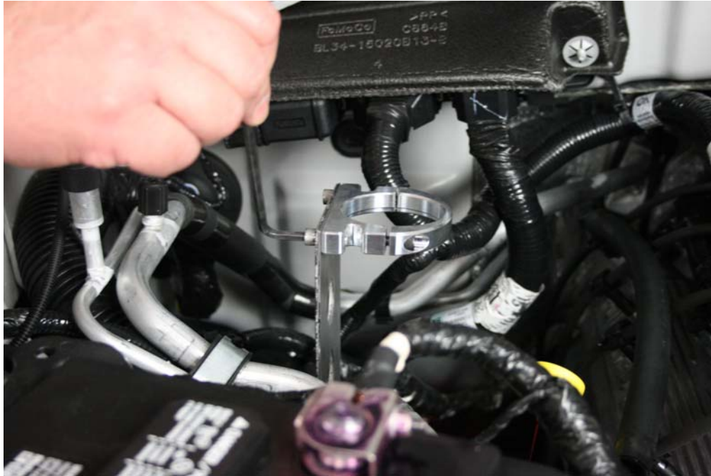
Step 14: Assemble billet clamp and stainless steel mount as shown using (2) ¼ - 20 x 5/8 SHCS.
