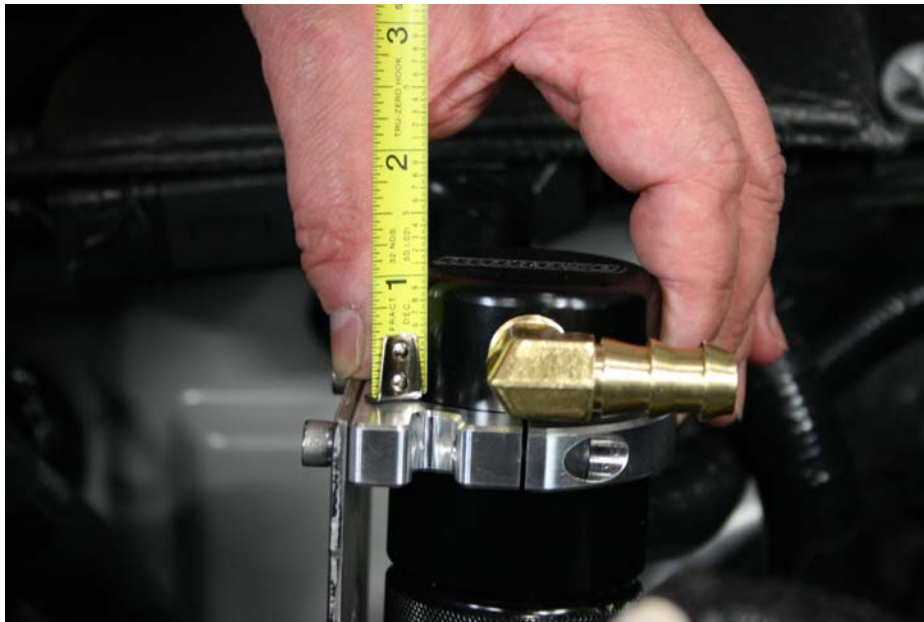
Step 17: Measure 1" down from top of Air Oil Separator and face barbed fitting toward valve cover / intake.
