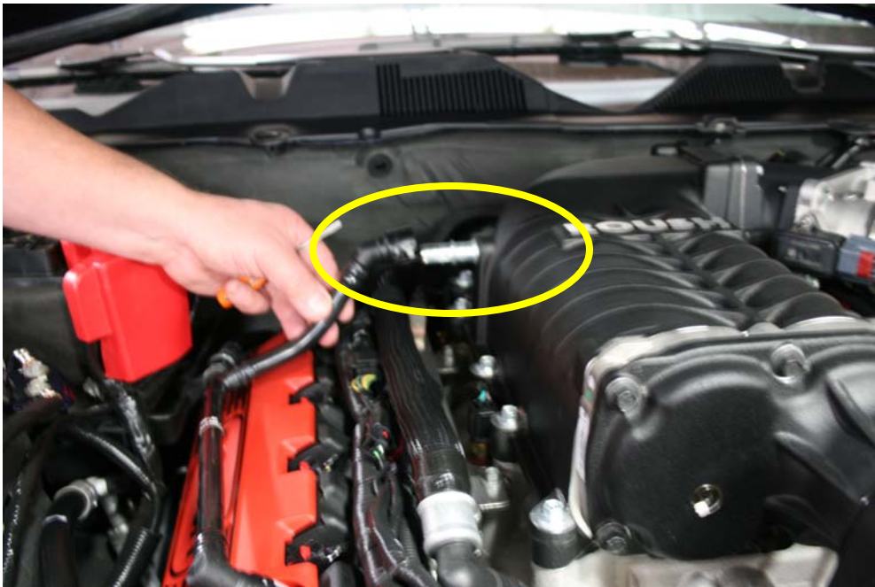
Step 2: Remove PCV line from Super Charger.
