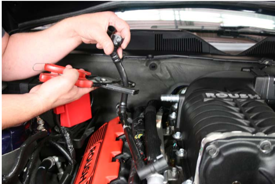
Step 4: Cut PCV line in the middle of radius area as shown.
