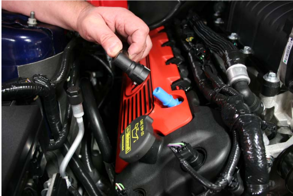
Step 3: Remove PCV line from valve cover.
