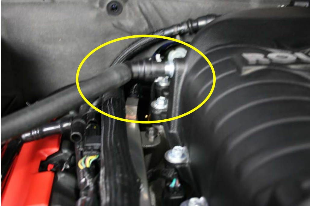
Step 10: Re-install 45 degree Super Charger fitting.
