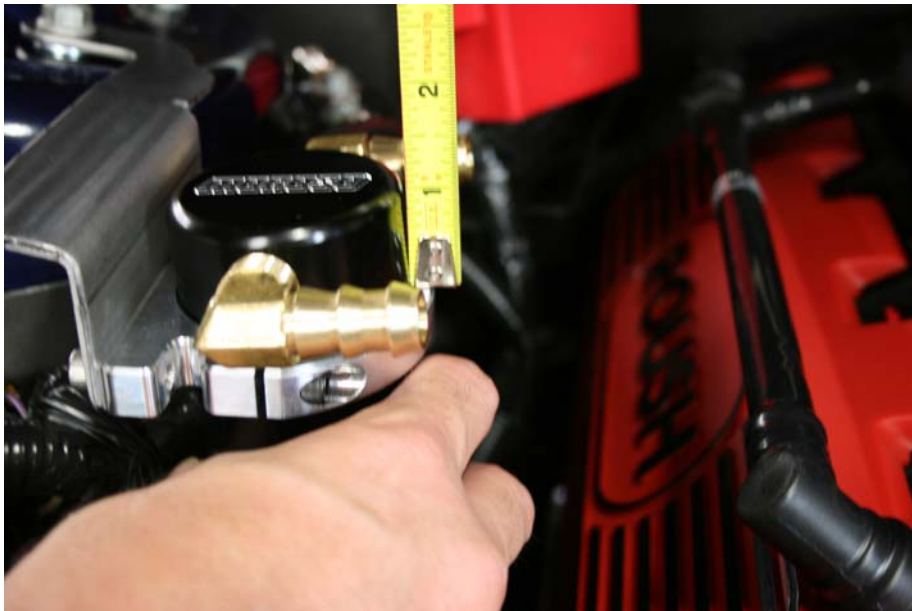
Step 19: Measure 1" down from top of Air Oil Separator and face barbed fitting toward valve cover / intake.
