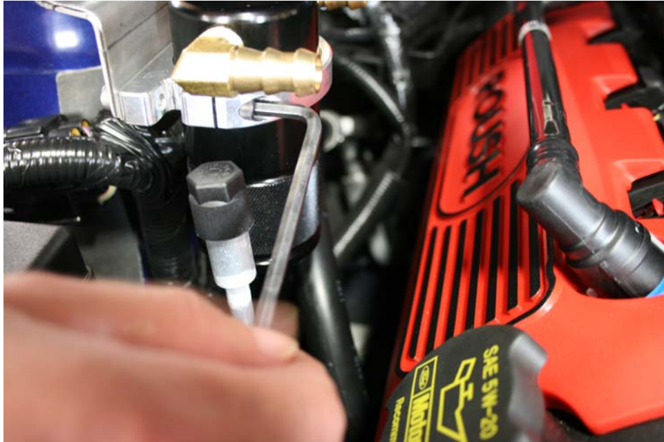
Step 20: Tighten socket head cap screws.
