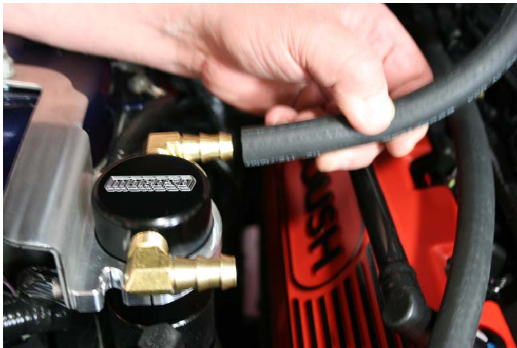
Step 21: Insert hose over barbed fitting from Super Charger to rear fitting on Air Oil Separator.
