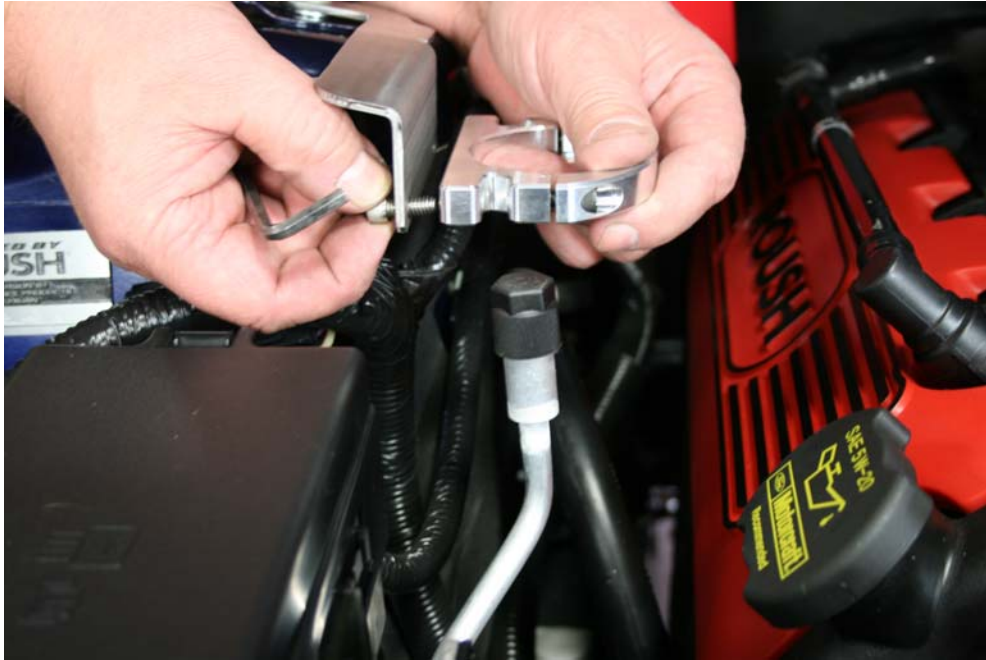
Step 17: Assemble billet clamp to stainless steel bracket using (2) 1/4-20x5/8.
