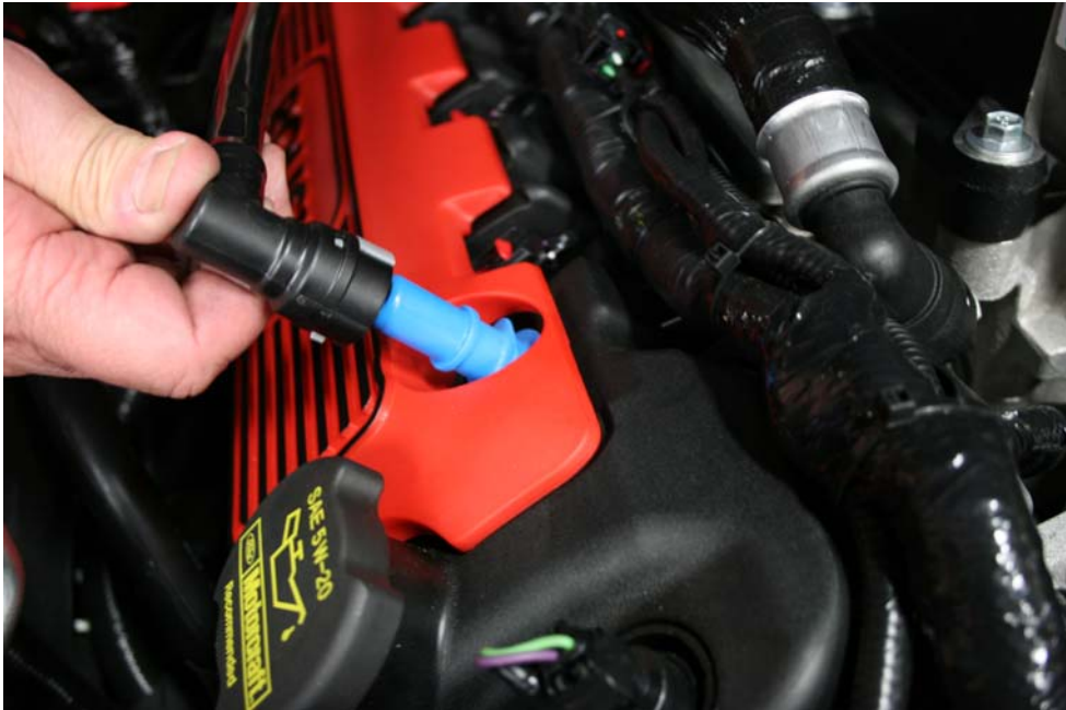
Step 8: Re-install valve cover fitting.
