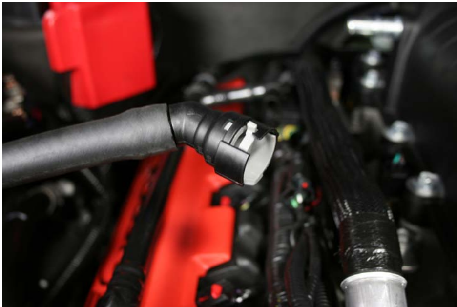
Step 9: Insert 45 degree fitting into 14" long hose.
