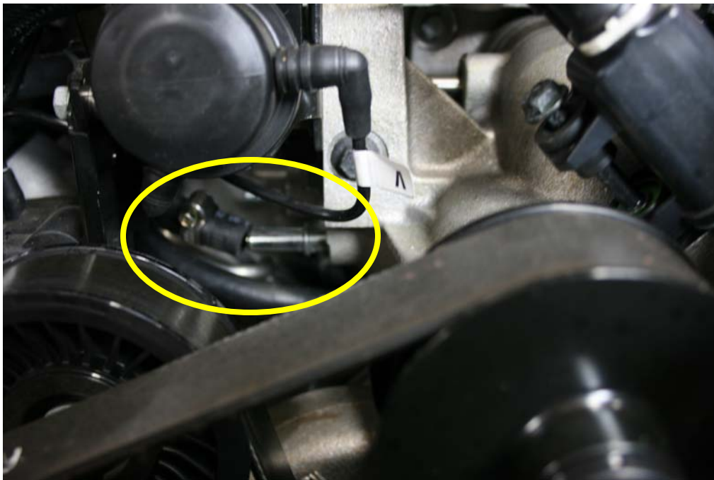
Step 16: Insert 48" long hose over intake nipple.
