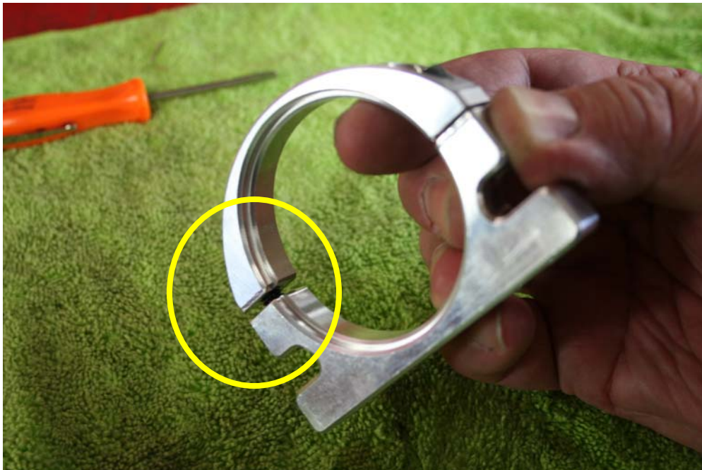
Step 5: Assemble billet clamp as shown with (2) \frac{1}{4} -20x5/8, make sure reliefs line up as shown. (Bottom of billet clamp shown)
