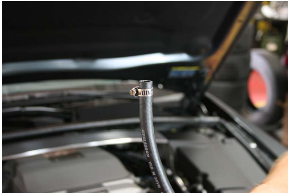
Step 12: Install hose clamp on 28" long hose.
