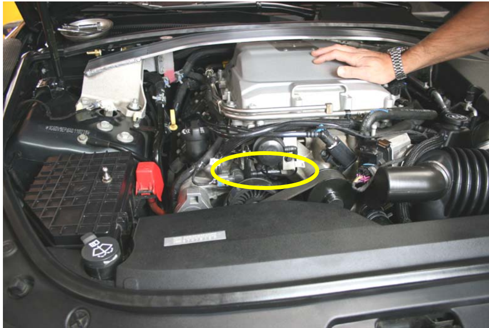
Step 10: Locate PCV line runs from bottom of intake to block valley.
