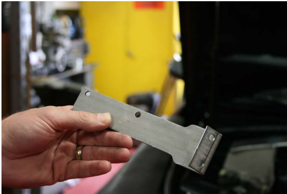
Step 4: Install stainless steel mounting bracket to filler neck mount using hardware previously removed.
