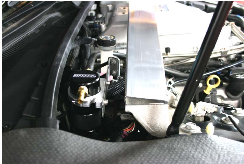
Step 15: Insert hose over Air Oil Separator nipple as shown.
