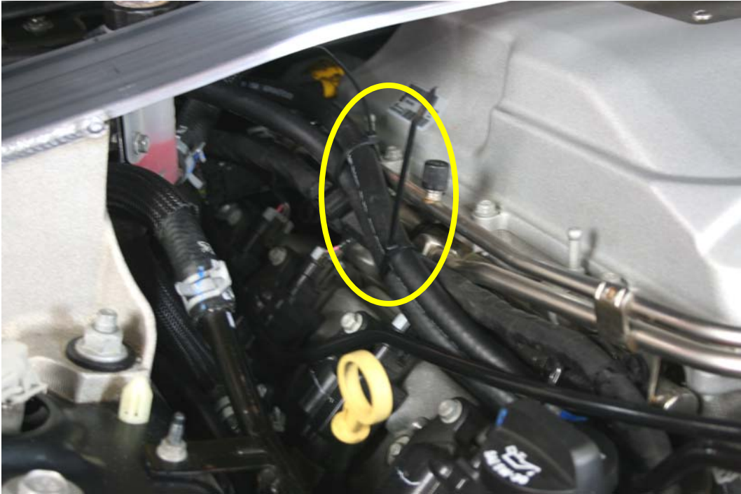
Step 19: Wire tie hoses as needed.
