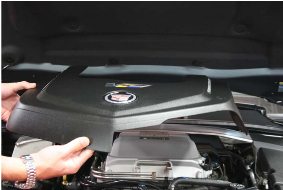
Step 1: Remove engine covers.
