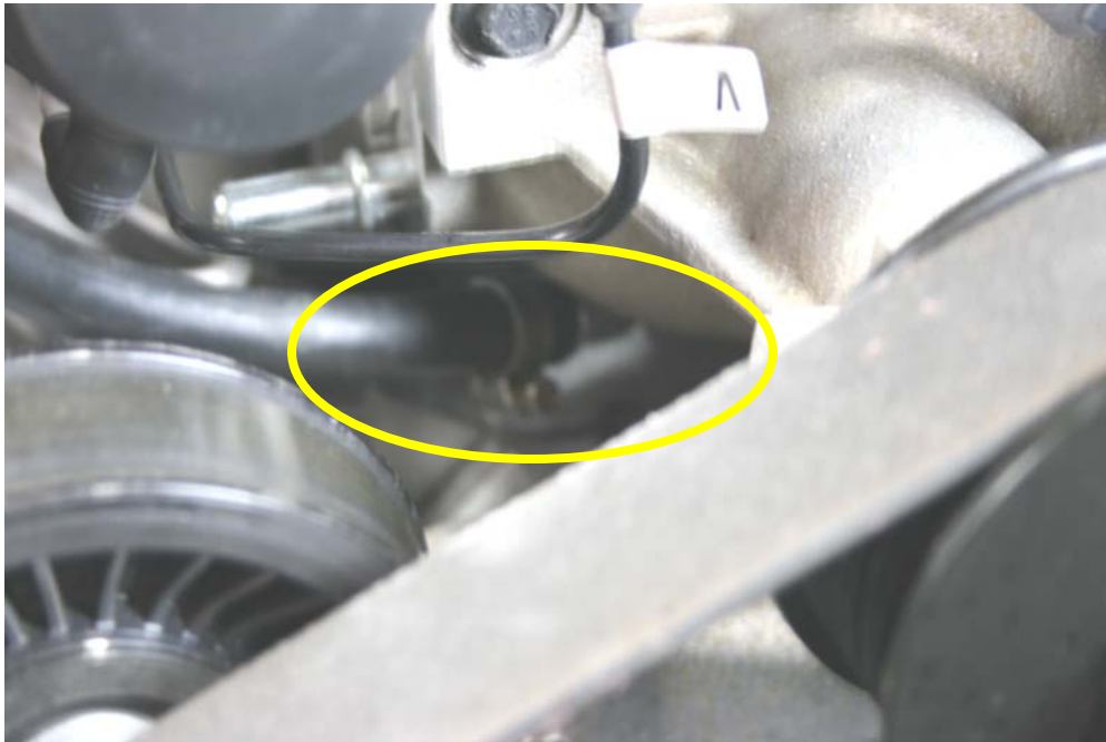
Step 13: Insert one end of hose over block valley nipple and tighten clamp.
