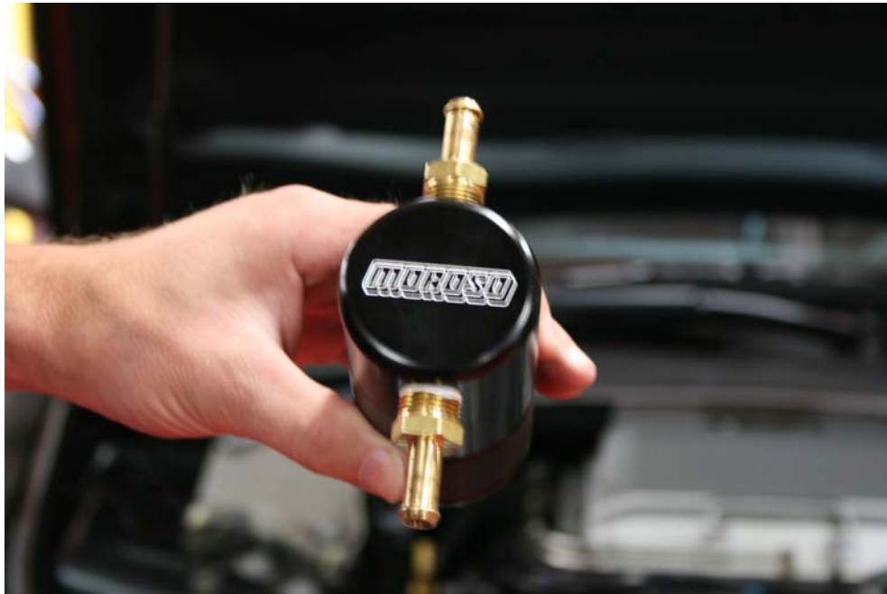
Step 6: Install brass fittings using Teflon tape.
