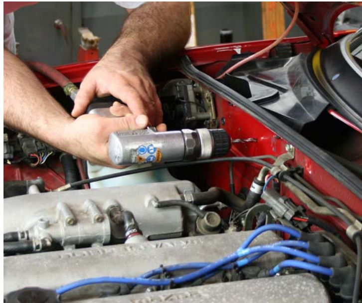
Step 7: Drill first 1/4" hole at marked location
