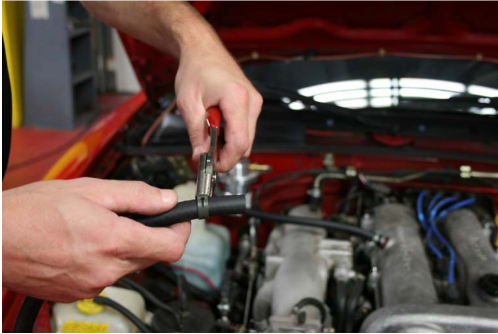
Step 18: Install (1) hose clamp on one end of 19" hose
