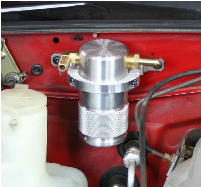
Step 10: Install Air Oil Separator using (2) \frac{1}{4} x 20 x \frac{5}{8} x BHCS
