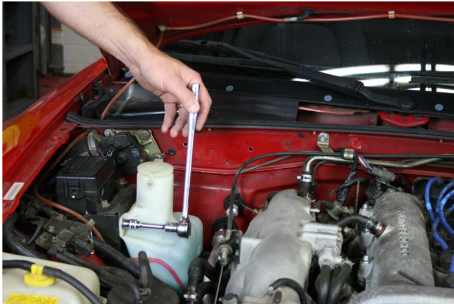
Step 9: Reinstall windshield washer tank mounting bolts
