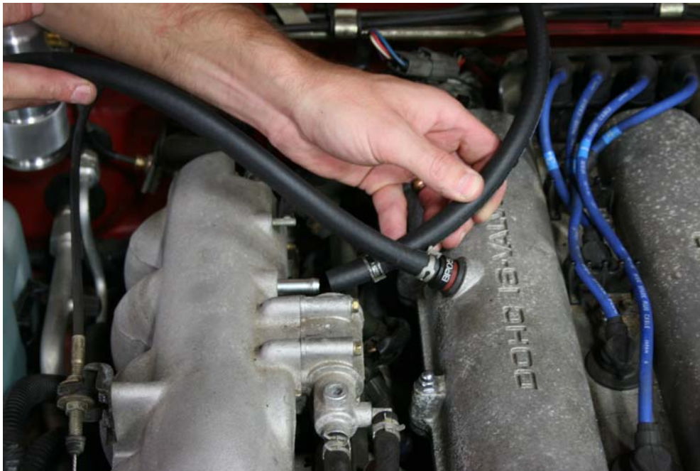
Step 19: Install hose over nipple and install hose clamp
