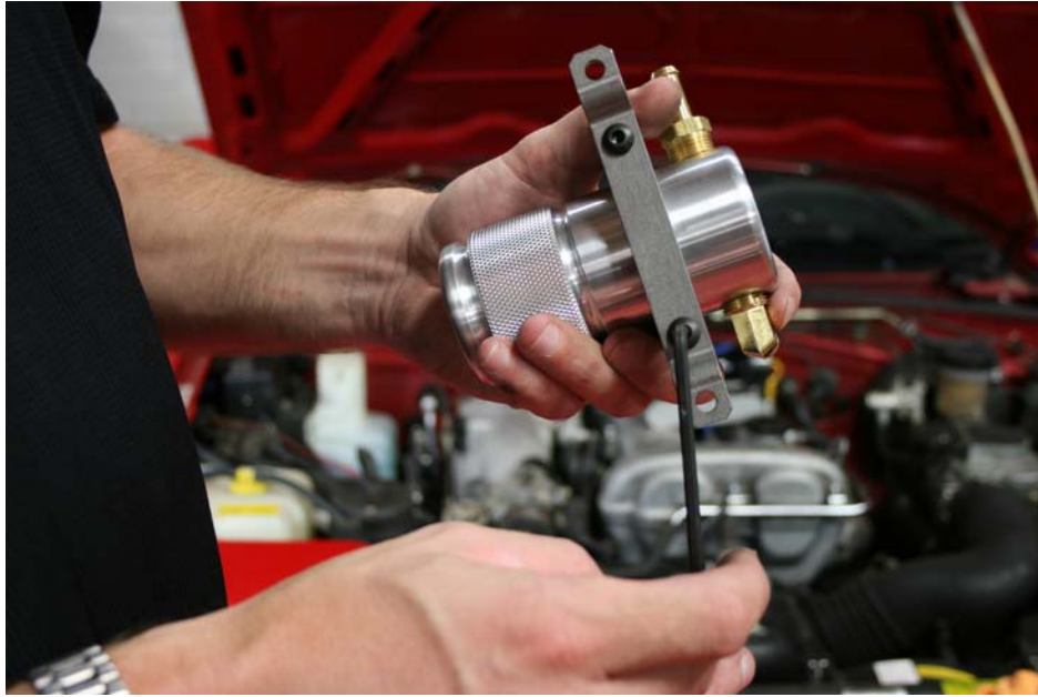
Step 3: Assemble billet clamp and stainless mounting bracket using (2) ¼ x 20 x 5/8 BHCS
