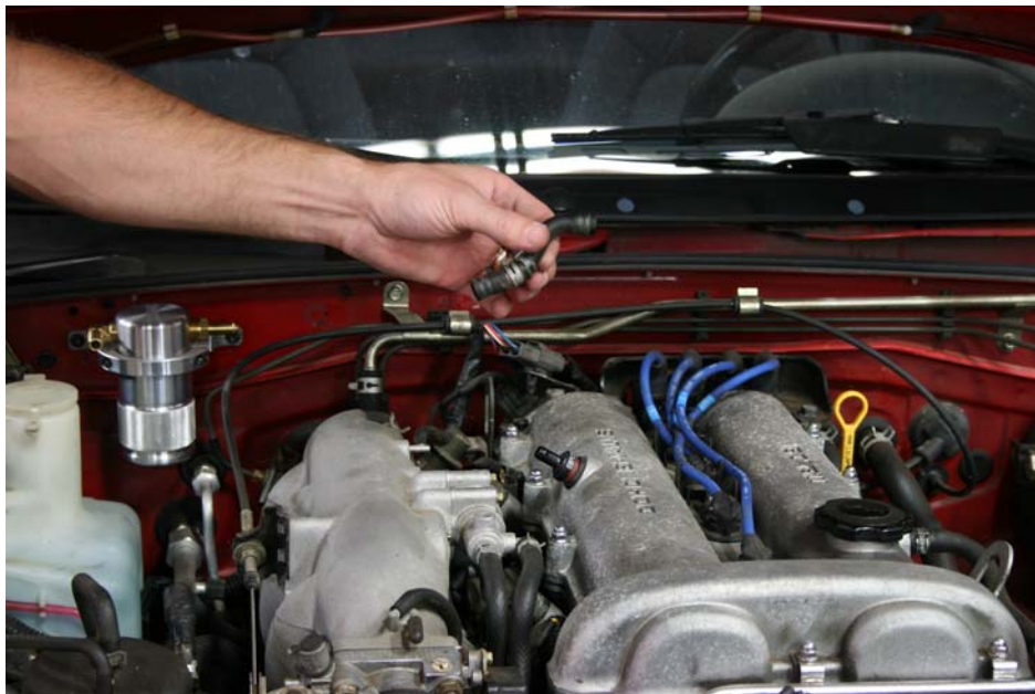
Step 14: Remove PCV line from vehicle and remove hose clamps for re-use
