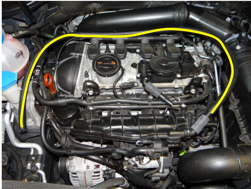
Step 7: Using ½" x 48" long hose provided in kit insert over nylon coupling nipple and route as shown.
