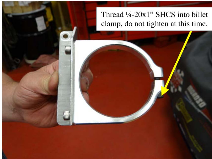
Step 11: Assemble billet clamp to stainless mounting bracket as shown using (2) 1/4-20x5/8 SHCS.
