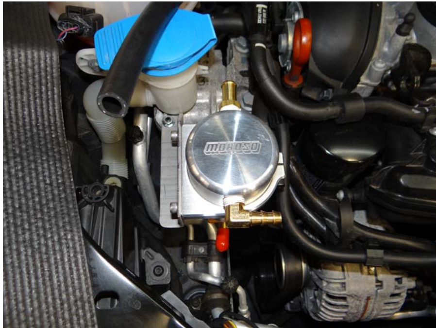
Step 15: Orient as shown and tighten clamp pinch bolt.
