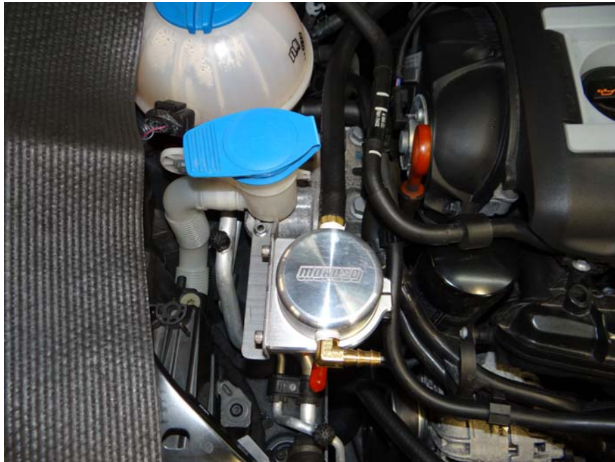
Step 16: Install hose to Air Oil Separator, trimming of hoses will be required.
