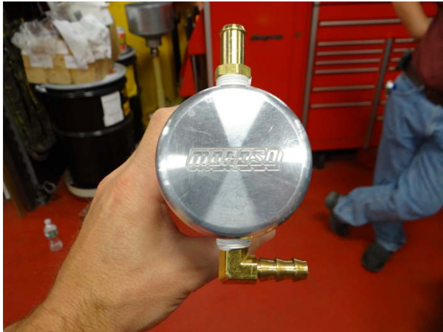
Step 13: Assemble Air Oil separator as shown using Teflon tap on all fittings.
