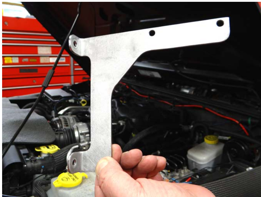
Step 13: Locate stainless mounting bracket from kit.
