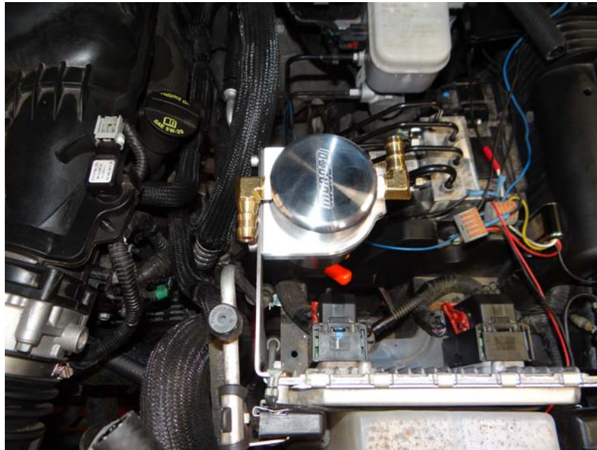
Step 19: Orientate as shown and tighten clamp.
