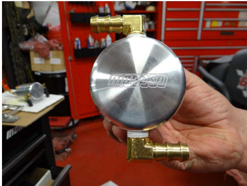
Step 16: Assemble air oil separator as shown using Teflon tape on fittings.
