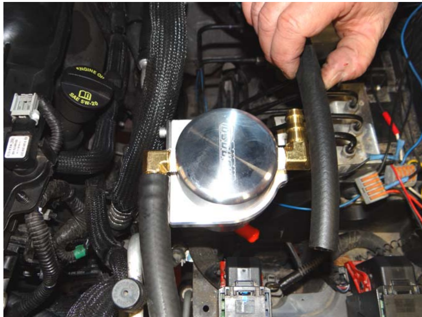
Step 22: Mark hose and cut to length as needed.
