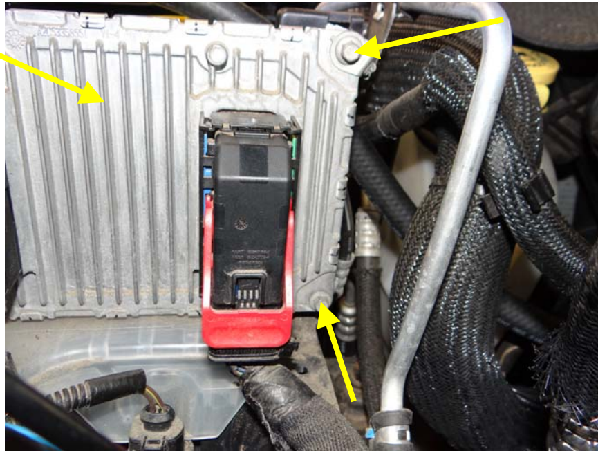
Step 12: Remove (2) mounting bolts shown.
