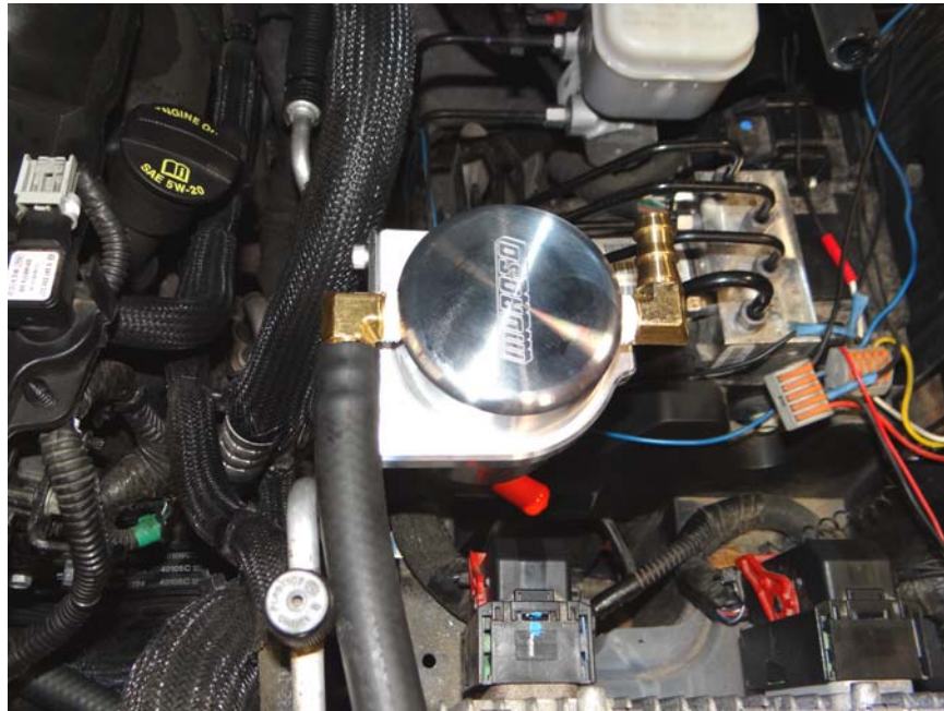
Step 21: Insert hose over nipple.
