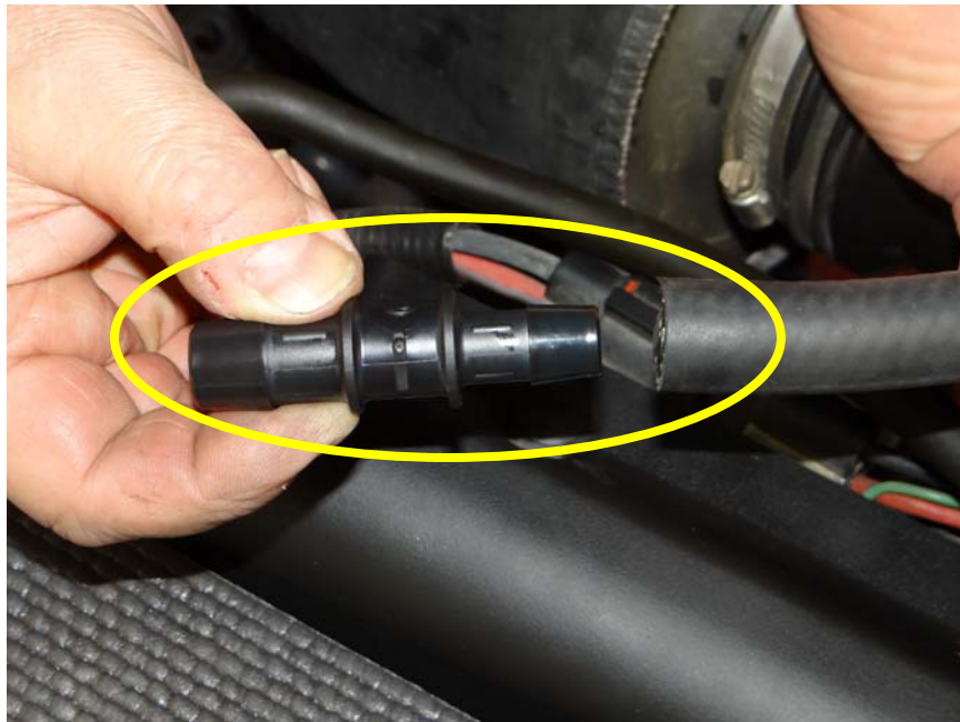
Step 4: Using 30" length of hose provided in kit insert coupling.
