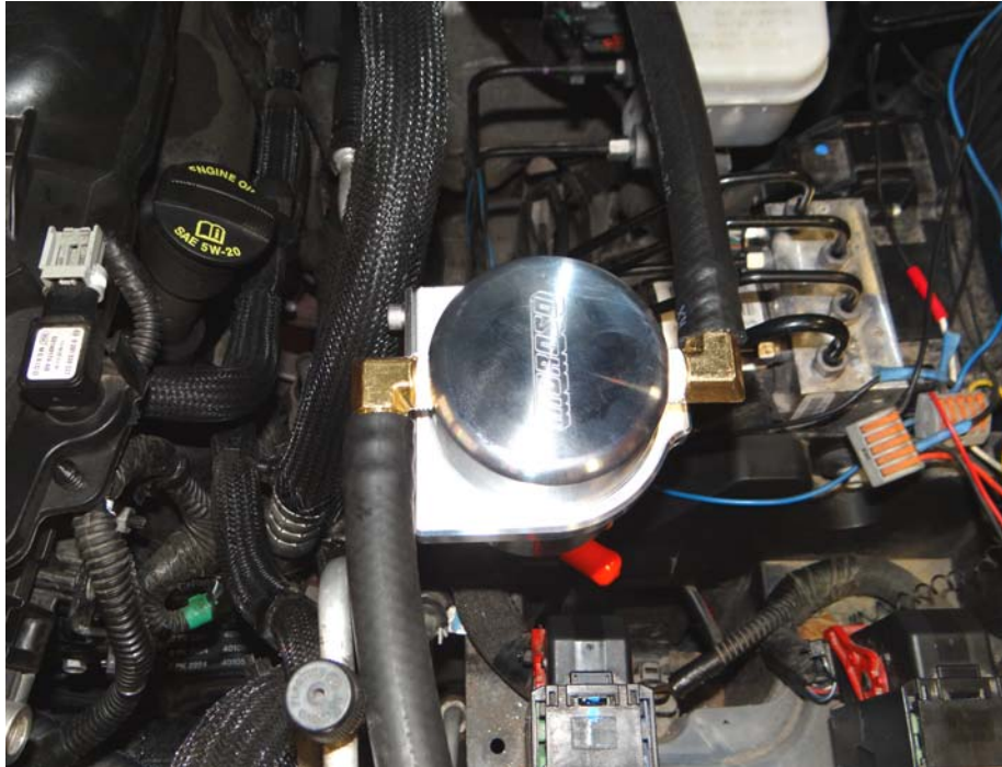
Step 23: Insert hose over nipple.
