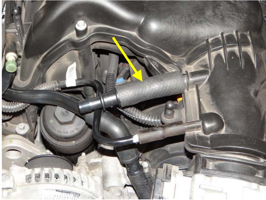
Step 8: Insert other end of 3" 5/8 hose to intake nipple.
