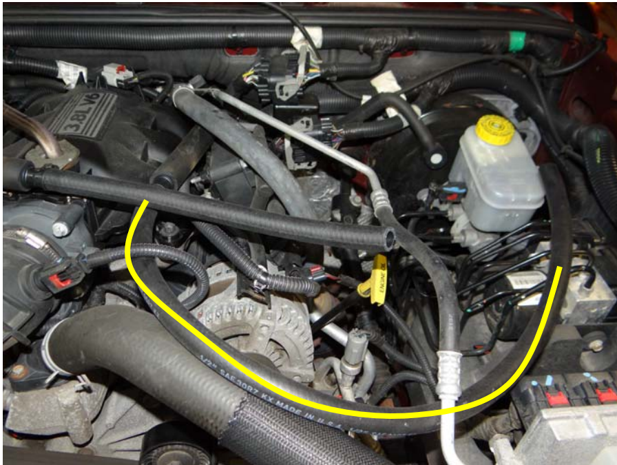
Step 8: Insert 24" length hose over coupling as shown.
