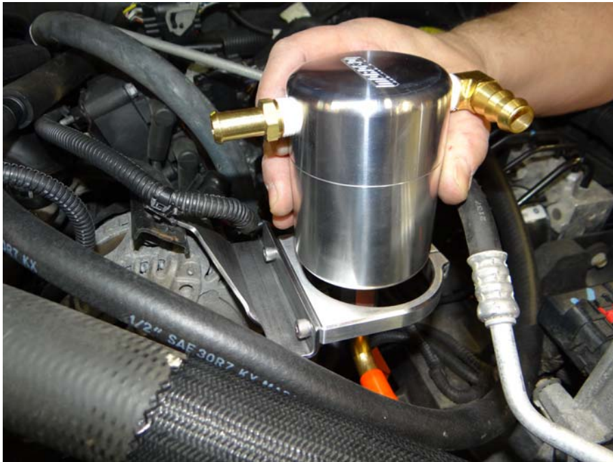
Step 13: Insert Air Oil Separator into billet clamp.
