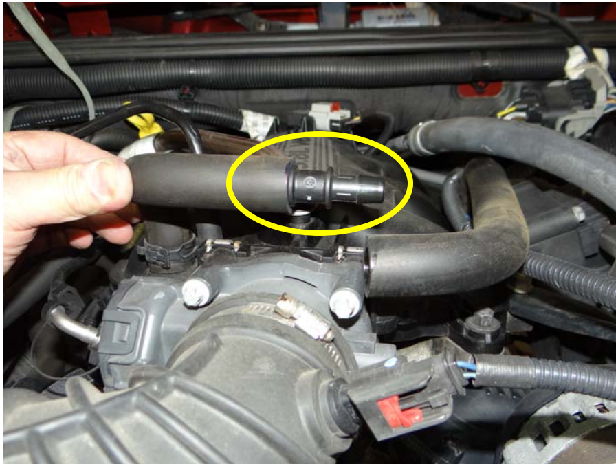
Step 4: Insert 1/2"x5/8" coupling into PCV hose.
