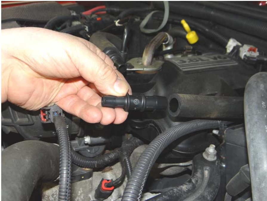
Step 6: Insert 1/2"x5/8" coupling into PCV hose.
