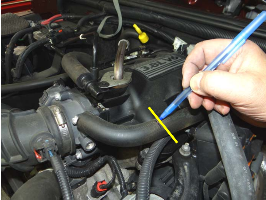
Step 5: Mark as shown and cut as shown in following illustrations.
