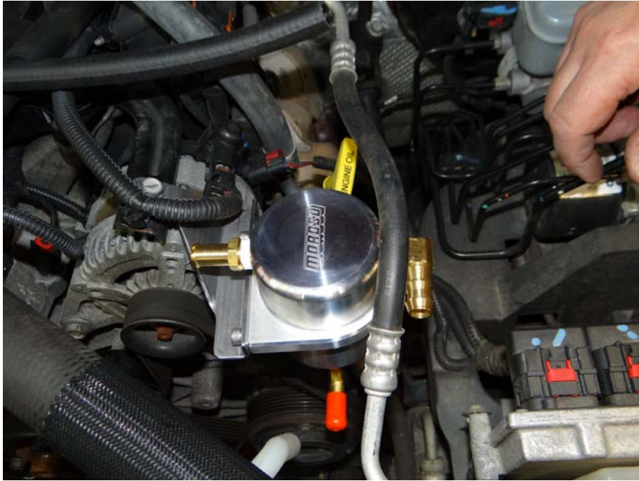
Step 14: Orientate as shown and tighten clamp pinch bolt.
