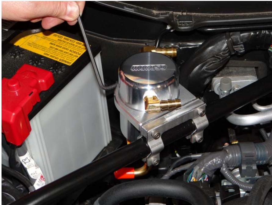
Step 13: Orientate barbed fitting towards driver's side and tighten clamp.
