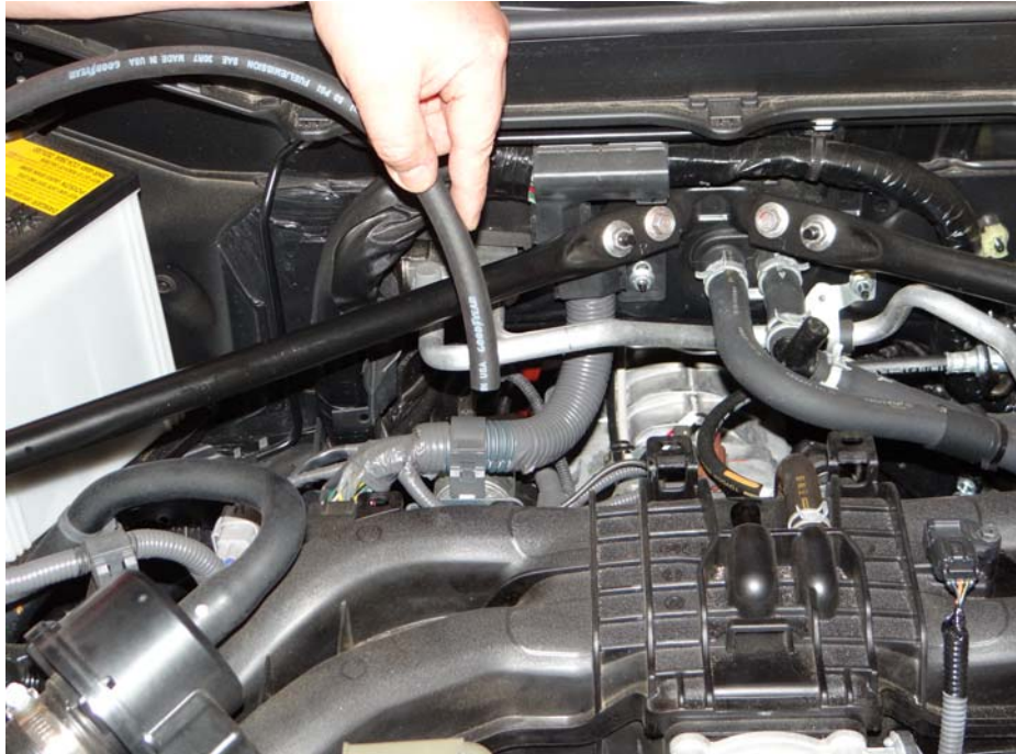
Step 5: Install 3/8" hose to PCV valve.
