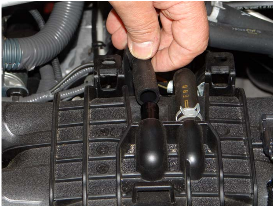
Step 3: Remove PCV line from intake.
