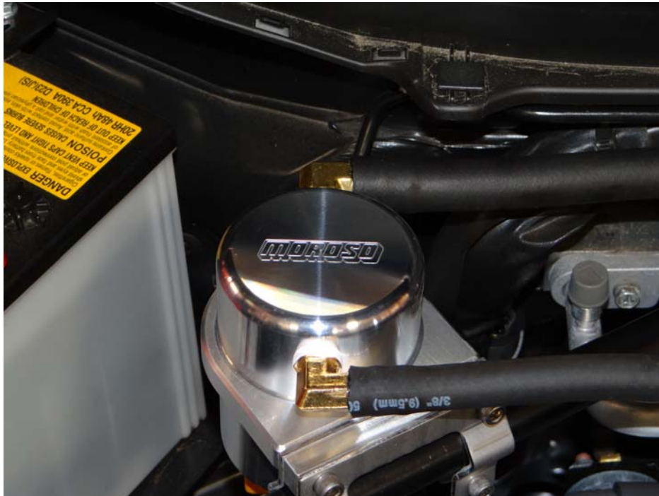
Step 15: Install 1/2" hose to 1/2" barbed fitting on Air Oil Separator.
