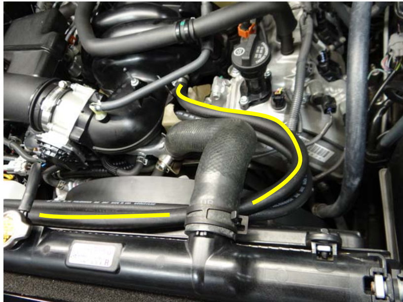
Step 6: Route lines previously installed over to passengers side of vehicle as shown.
