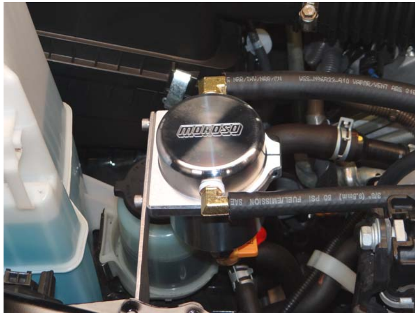
Step 14: Route 1/2" hose to Air Oil Separator, trim hose if needed and install.
