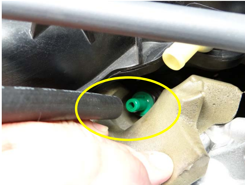
Step 4: Using 3/8" length of hose install over PCV valve.
