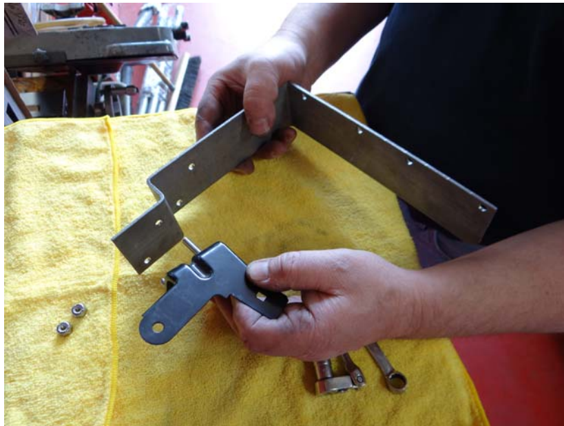
Step 31: Install wiring harness bracket previously removed from vehicle to stainless mounting bracket using (2) ¼-20 HHCS and (2) ¼-20 nylock nuts.
