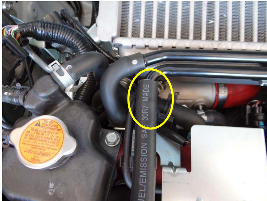
Step 29: Using 32" long 1/2 I.D.hose insert over crossover tube nipple as shown.
