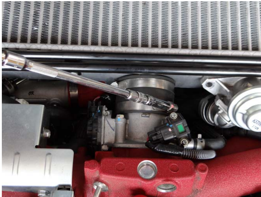
Step 6: Loosen Throttle body coupling clamps.
