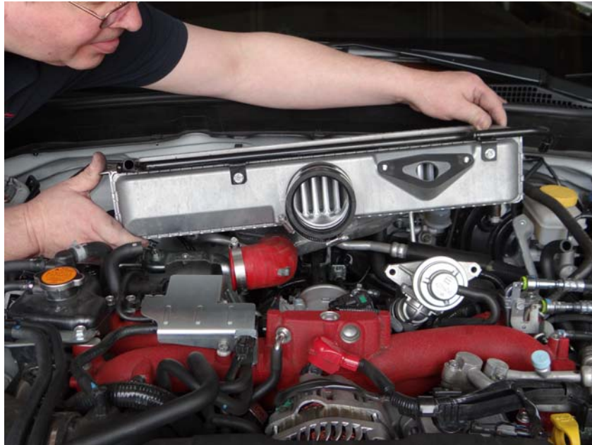
Step 9: Remove intercooler from vehicle.
