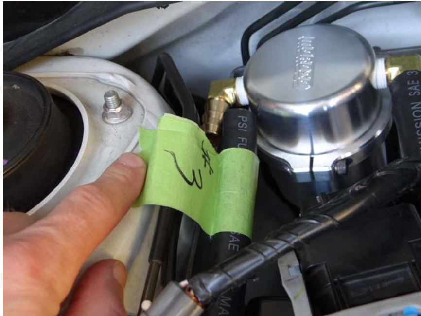
Step 44: Route hose #3 to Air Oil Separator, mark, trim and install.
