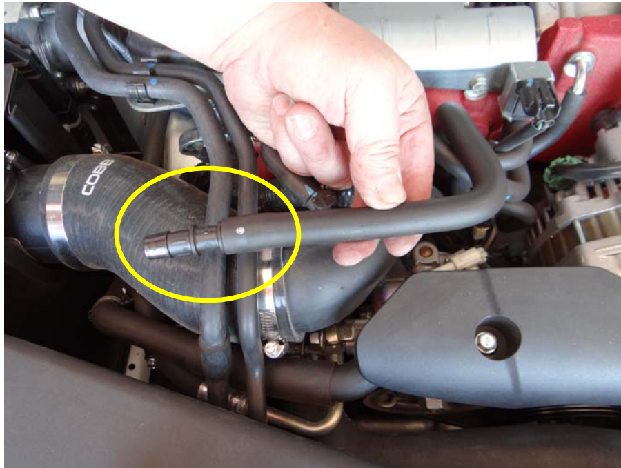
Step 26: Locate vacuum line previously removed in step 3, insert 1/2" coupling.
