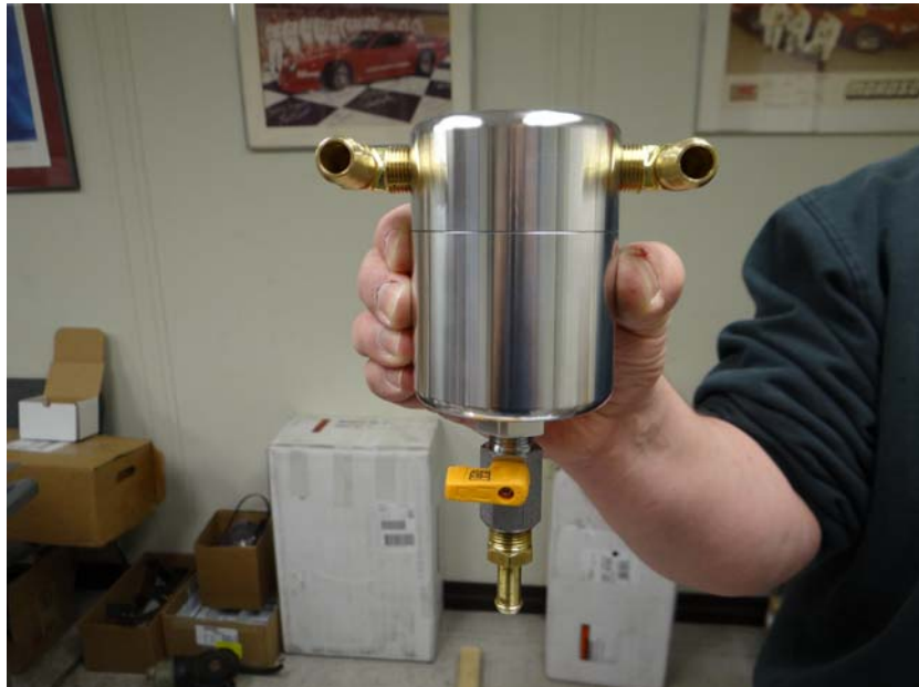
Step 36: Assemble ball valve and 3/8" straight barbed fitting in orientation shown using Teflon Tape.
