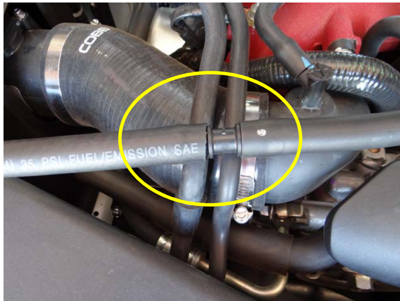
Step 27: Using 32" long 1/2 I.D.hose insert over 1/2" coupling.
