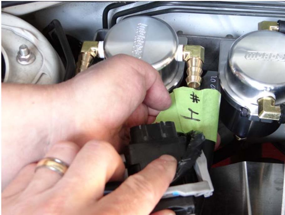
Step 43: Route hose #4 to Air Oil Separator, mark, trim and install.
