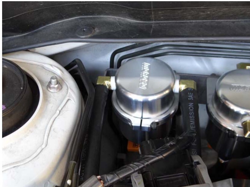
Step 44: Route hose #3 to Air Oil Separator, mark, trim and install.
