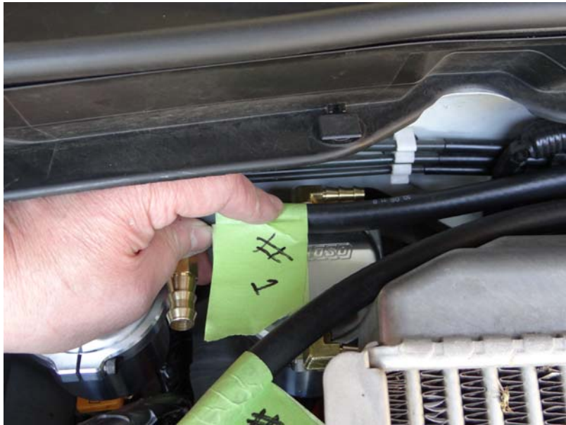
Step 40: Route hose #1 to Air Oil Separator mark and trim.
