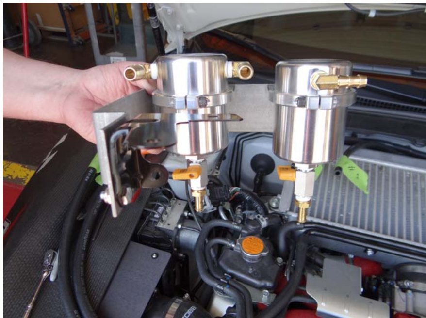
Step 37: Insert Air Oil Separators into billet clamps in the orientation shown.
