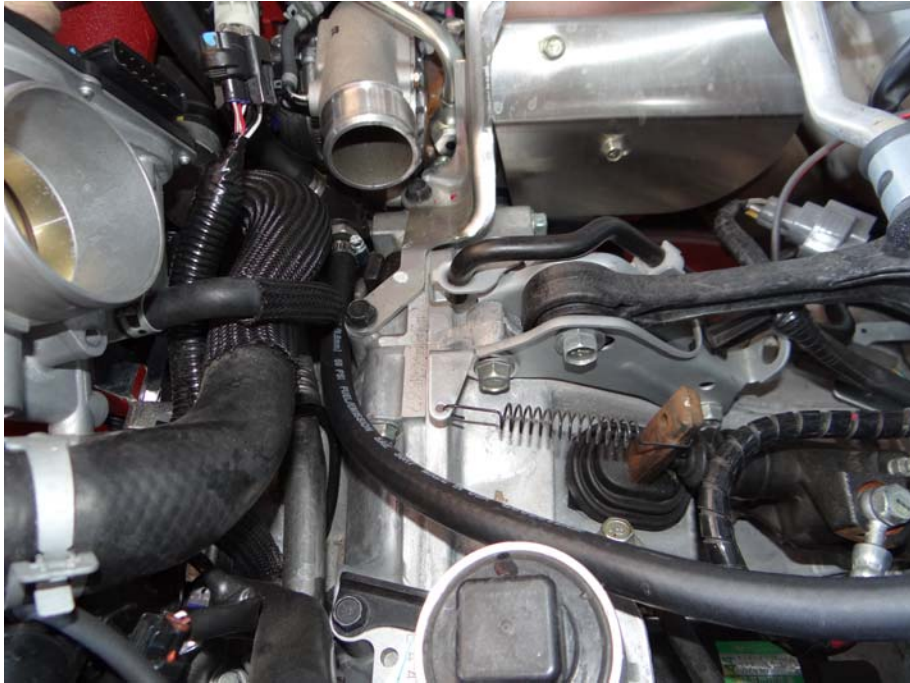
Step 17: Route 3/8 hose as shown to firewall and label hose #1.
