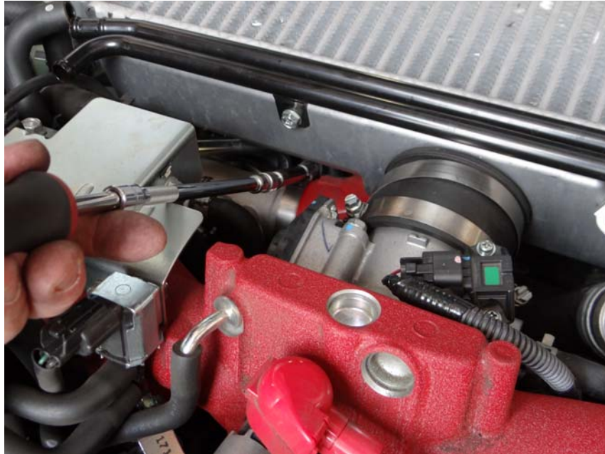
Step 7: Loosen intercooler inlet elbow clamp.
