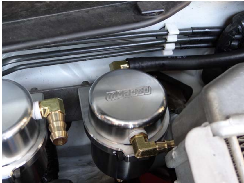
Step 41: Install hose #1 to Air Oil Separator.
