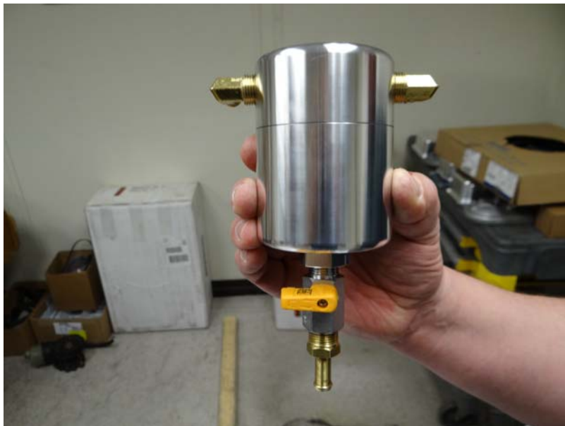
Step 34: Assemble ball valve and 3/8 straight barbed fitting in orientation shown using Teflon Tape.
