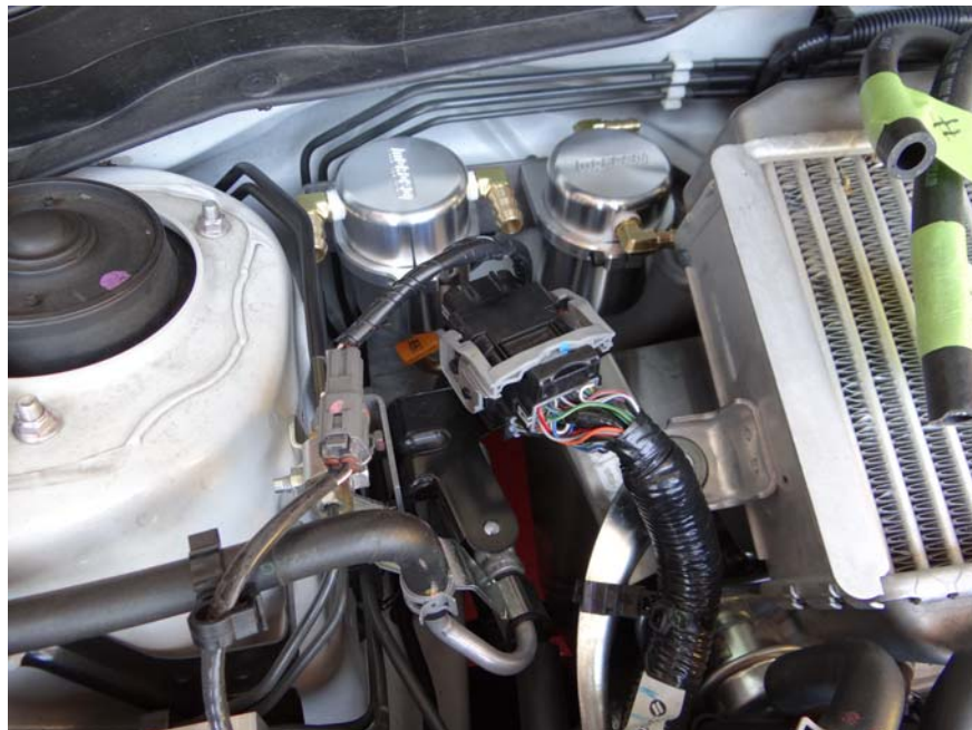
Step 39: Install assembly in vehicle using wiring harness bracket location and mounting hardware previously removed.
