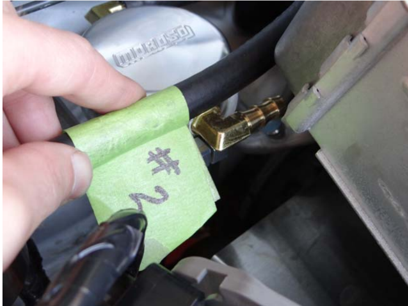
Step 42: Route hose #2 to Air Oil Separator, mark, trim and install.
