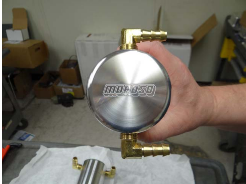
Step 33: Assemble (1) Air Oil Separator as shown using (2) 3/8" barbed fittings using Teflon tape.
