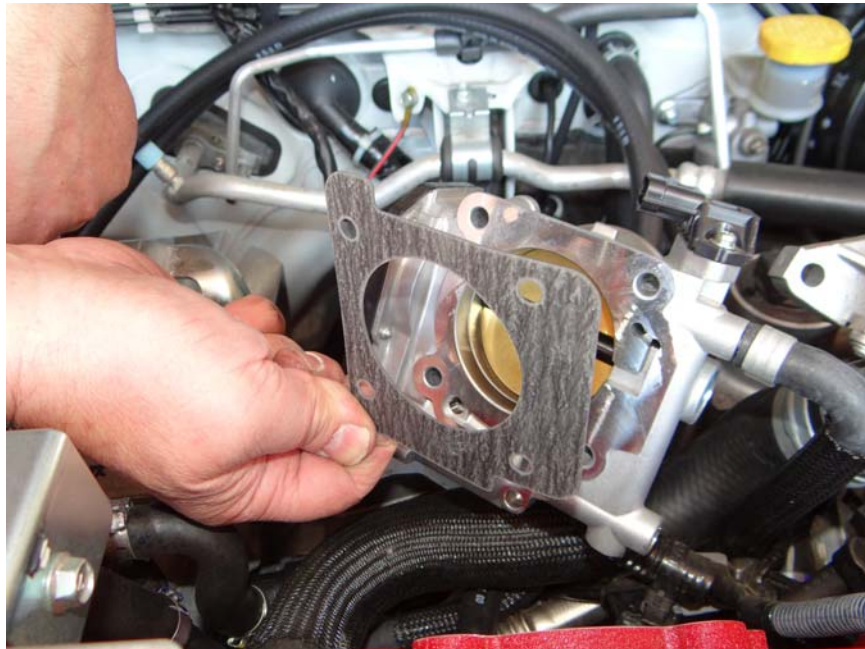
Step 21: Replace old throttle body gasket with new gasket provided in kit.
