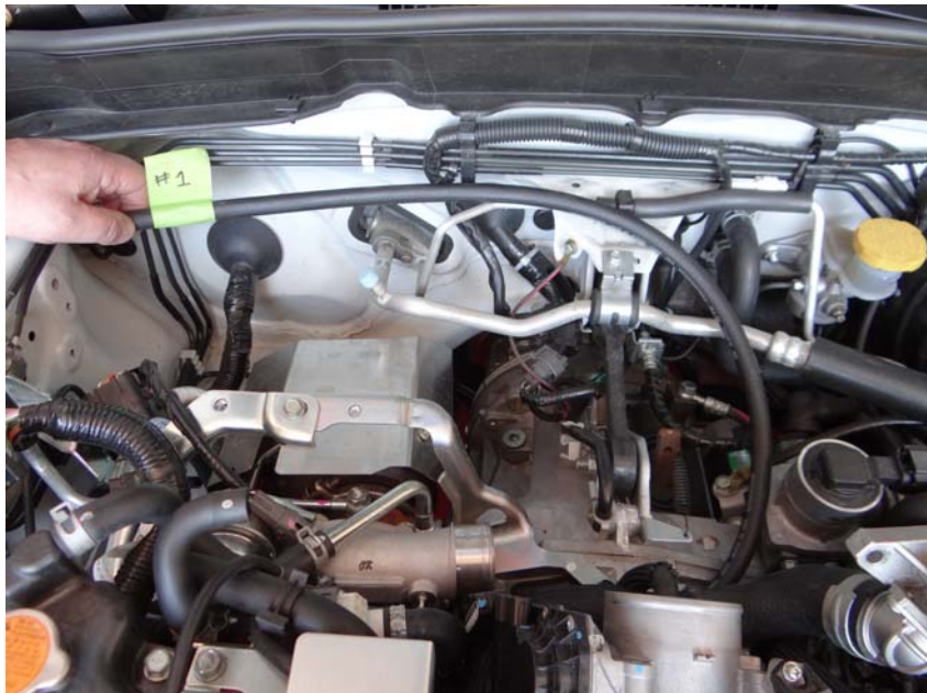
Step 17: Route 3/8 hose as shown to firewall and label hose #1.
