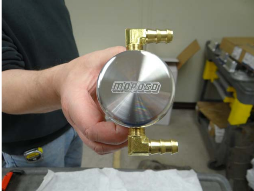
Step 35: Assemble (1) Air Oil Separator as shown using (2) 1/2" barbed fittings using Teflon tape.
