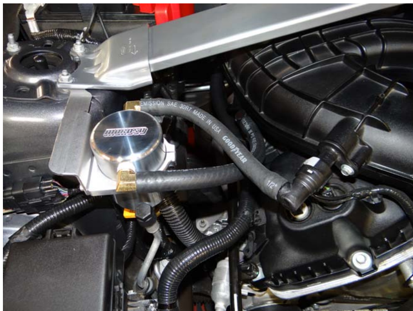
Step 15: Install other end to Air Oil Separator as shown.
