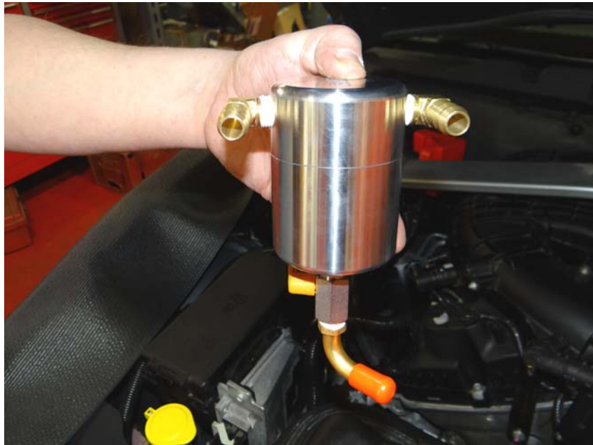
Step 11: Assemble Air Oil Separator as shown using Teflon tape on all fittings.
