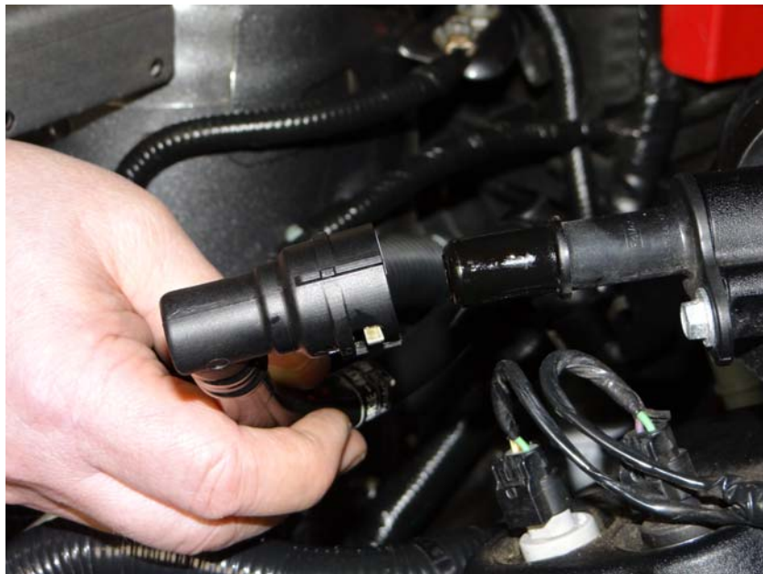
Step 6: Locate PCV tube and remove from vehicle.
