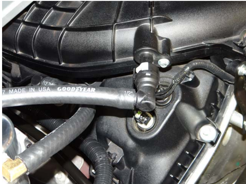
Step 15: Install 8 1/4" long hose to intake fitting as shown.
