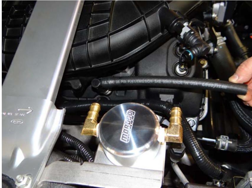
Step 13: Install 10" long hose to valve cover fitting as shown.
