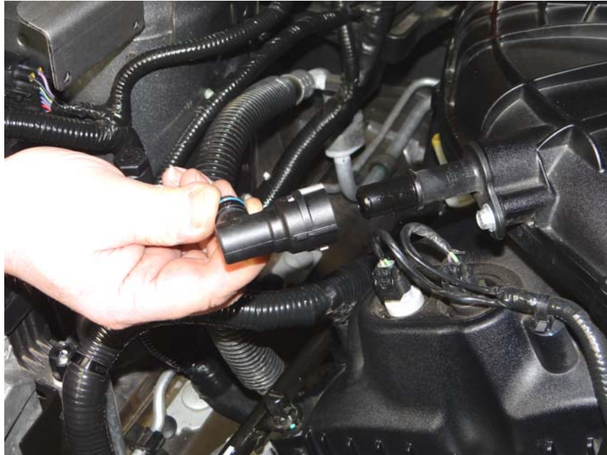
Step 8: Re-install 90 degree fitting in original location.
