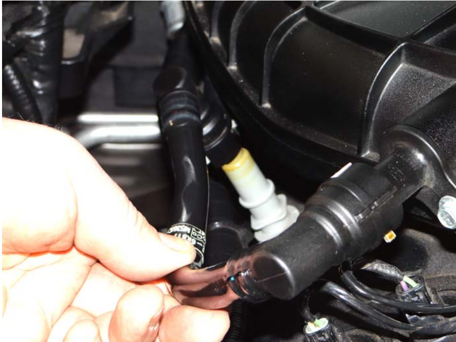
Step 6: Locate PCV tube and remove from vehicle.
