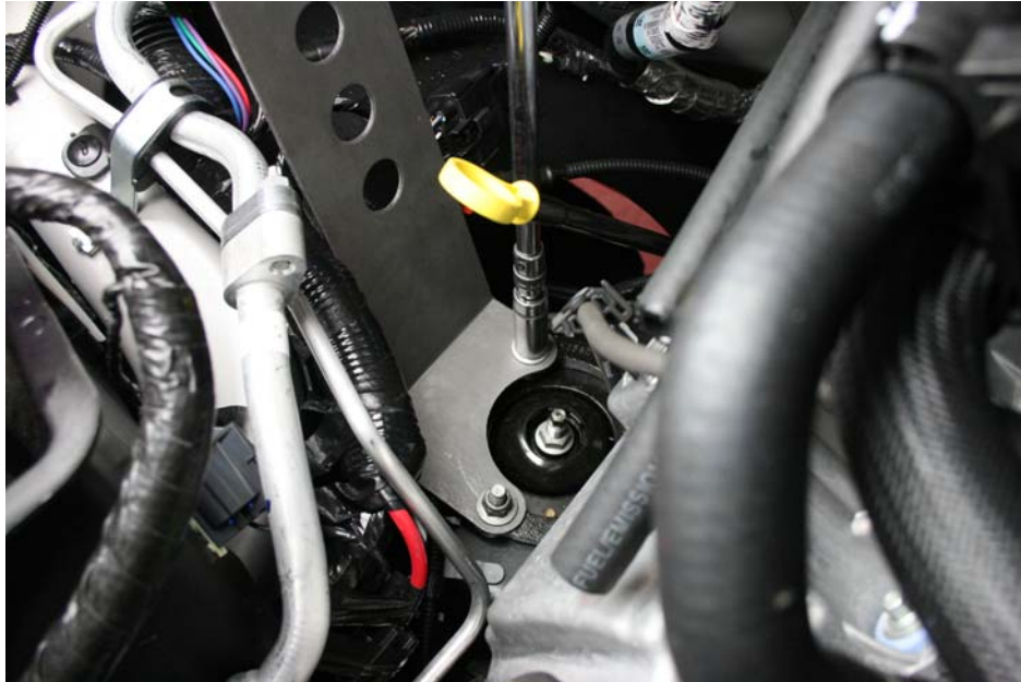
Step 12: Install and tighten strut tower mount nuts.
