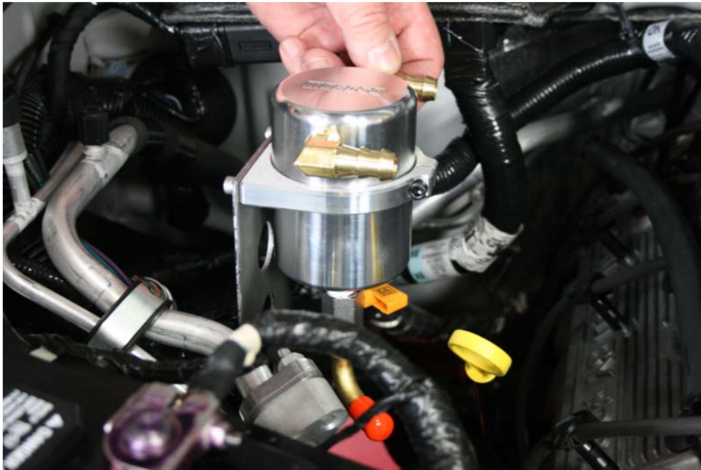
Step 17: Line up seam of Air Oil Separator with top of billet clamp, face barbed fitting toward valve cover / intake.
