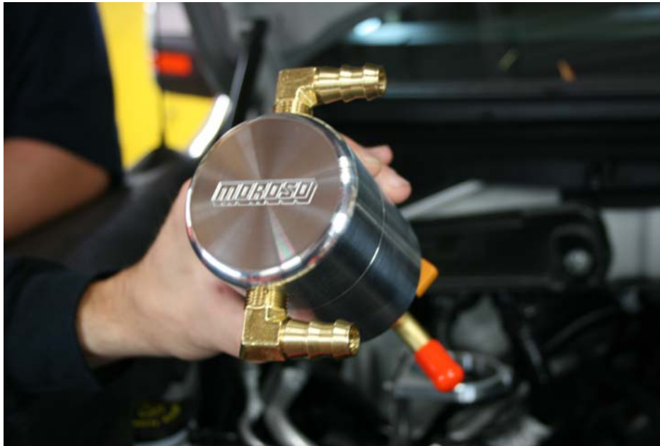
Step 15: Assemble Air Oil Separator as shown applying Teflon tape to all fittings.
