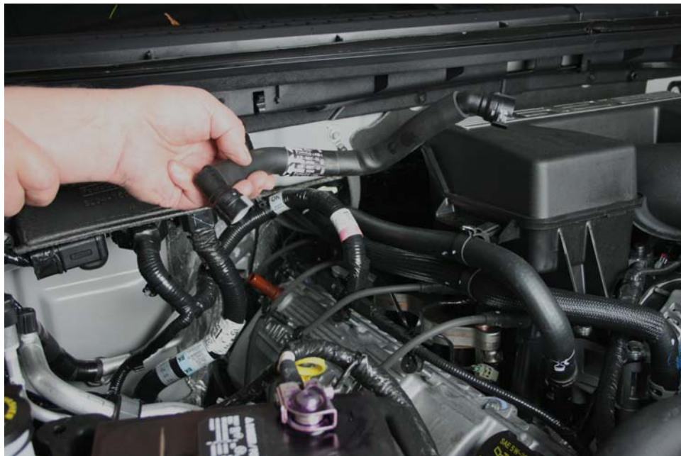
Step 2: Remove PCV line from vehicle.
