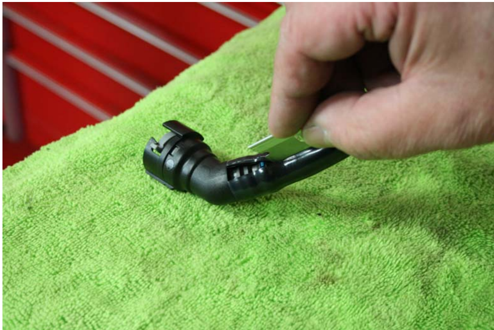
Step 4: Cut / slice PCV tubing from fitting using razor blade as shown.
