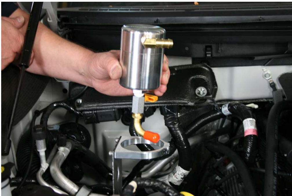
Step 16: Insert Air Oil Separator into billet clamp.
