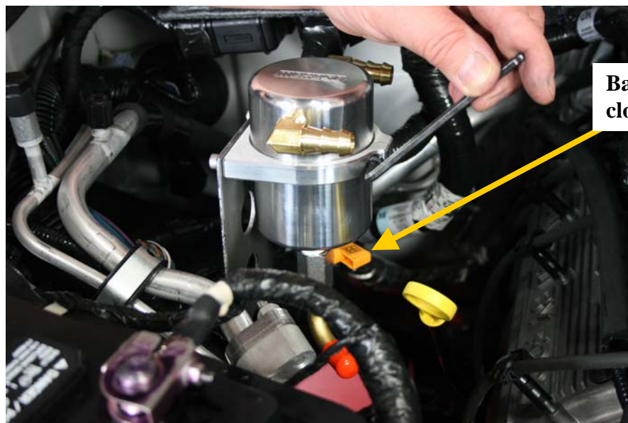
Step 18: Tighten socket head cap screw and make certain ball valve is in the closed position.
