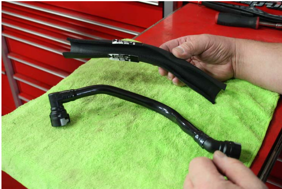
Step 3: Remove insulation from PCV line by slicing / cutting with razor blade.
