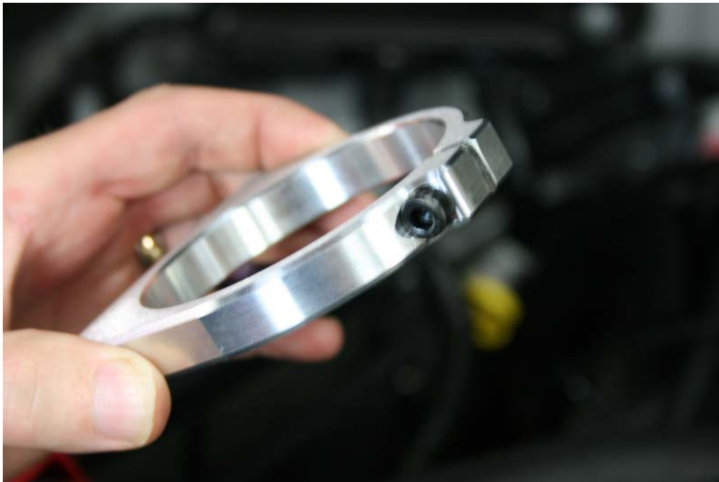
Step 13: Thread \frac{1}{4} -20 x 1 SHCS into billet clamp, do not tighten.
