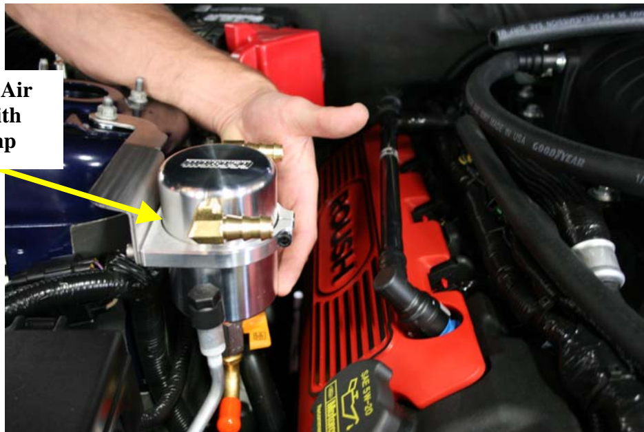
Step 19: Insert Air Oil Separator into billet clamp, line up seam with top of billet clamp, barbed fittings will need to face valve cover.
