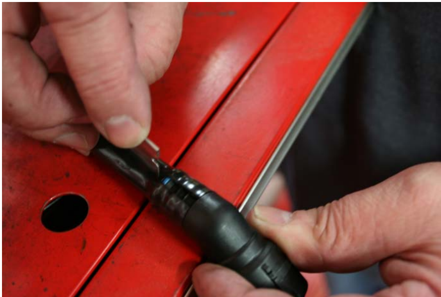
Step 5: Using a razor blade or knife slice the outer PCV line from 45 degree fitting removed from Super Charger.
