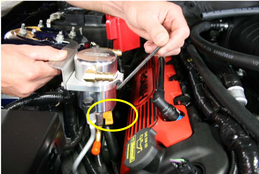
Step 20: Tighten socket head cap screw and make sure ball valve is in the closed position.
