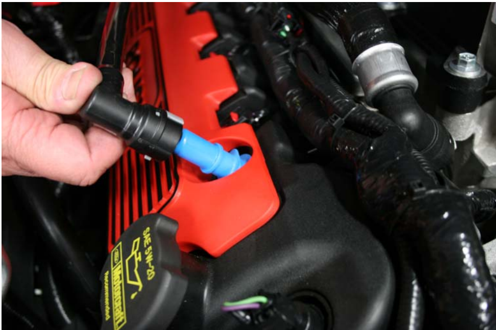
Step 8: Re-install valve cover fitting.
