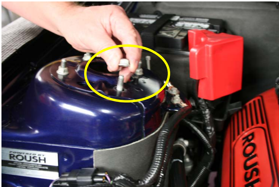
Step 13: Remove strut tower nut.
