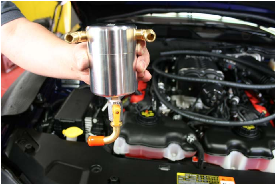
Step 18: Assemble Air Oil Separator as shown using Teflon tape on all fittings.
