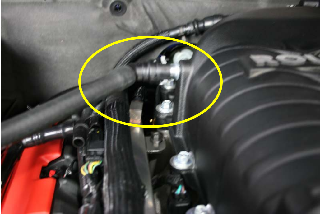
Step 10: Re-install 45 degree Super Charger fitting.
