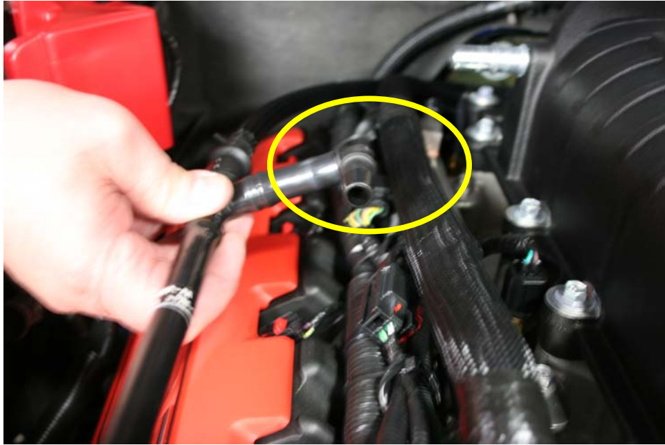
Step 7: Insert 90 degree fitting into PCV line as shown.
