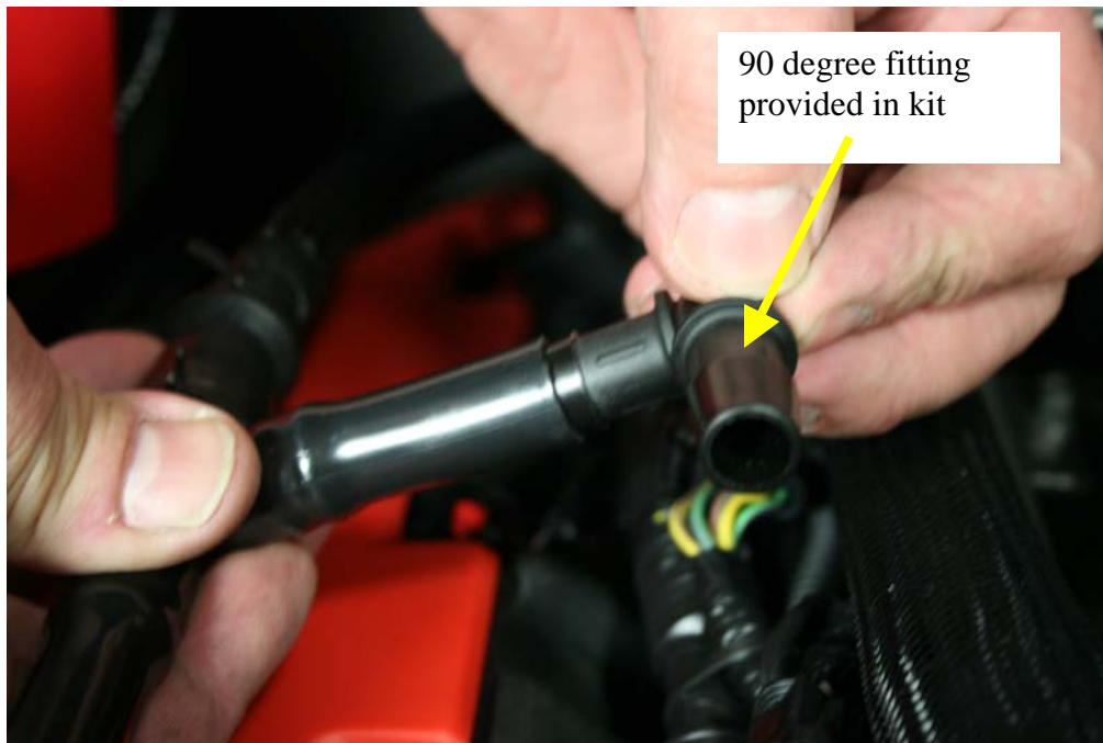
Step 6: Remove fitting from PCV line and set fitting aside.
