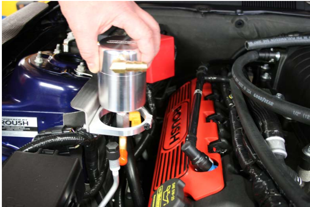
Step 19: Insert Air Oil Separator into billet clamp, line up seam with top of billet clamp, barbed fittings will need to face valve cover.
