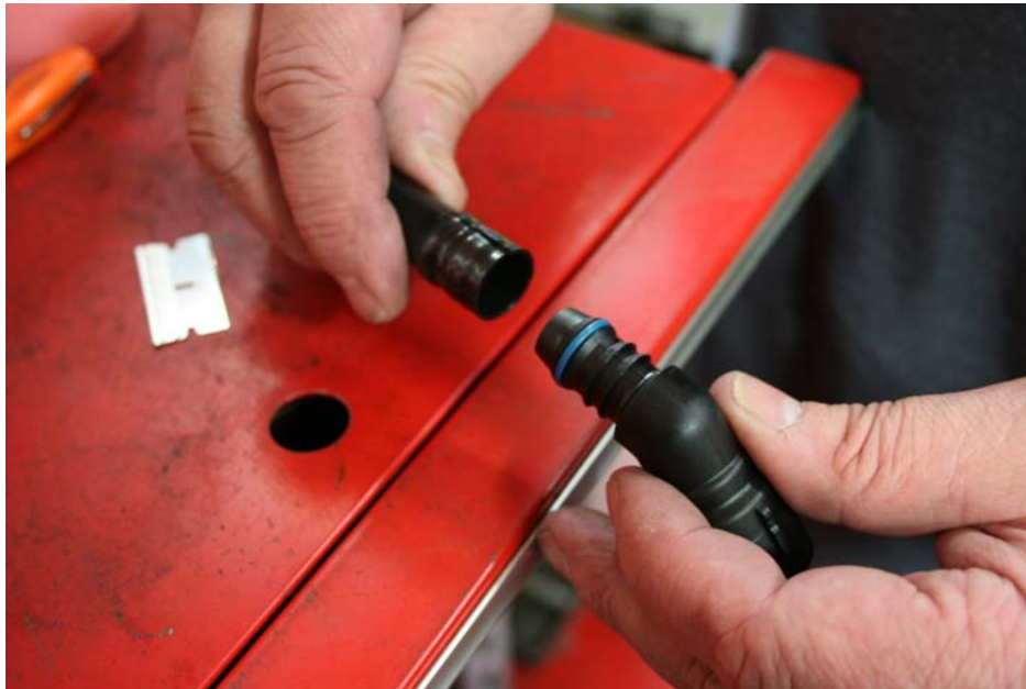
Step 6: Remove fitting from PCV line and set fitting aside.
