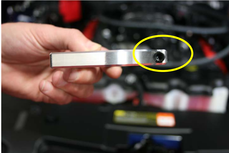
Step 16: Thread 1/4-20x1 SHCS into billet clamp do not tighten.
