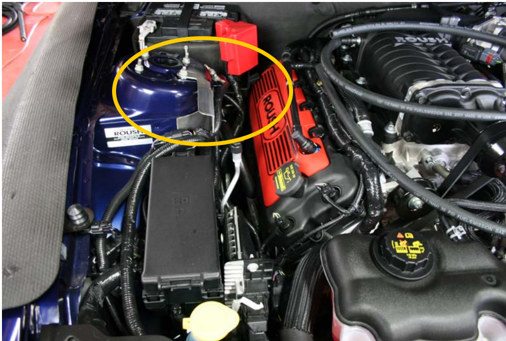
Step 15: Install and tighten strut tower nut previously removed.
