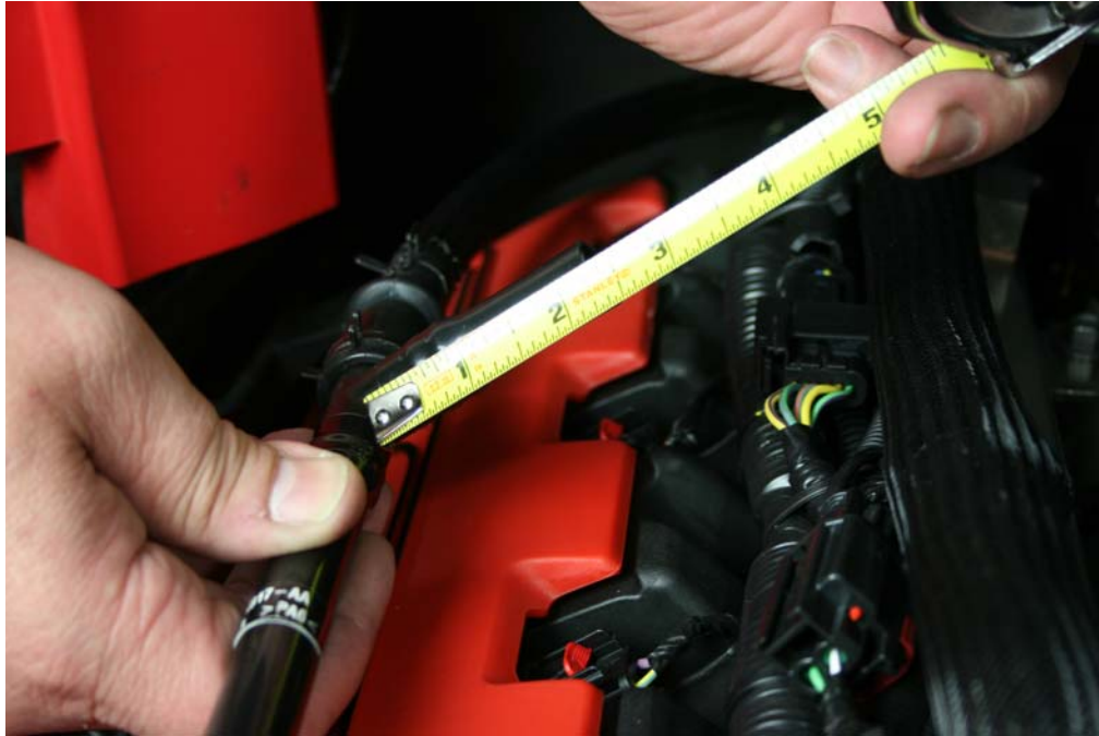
Step 4: Cut remainder of radius from PCV line leaving approximately 2 ¼" to 2 ½" long straight area.
