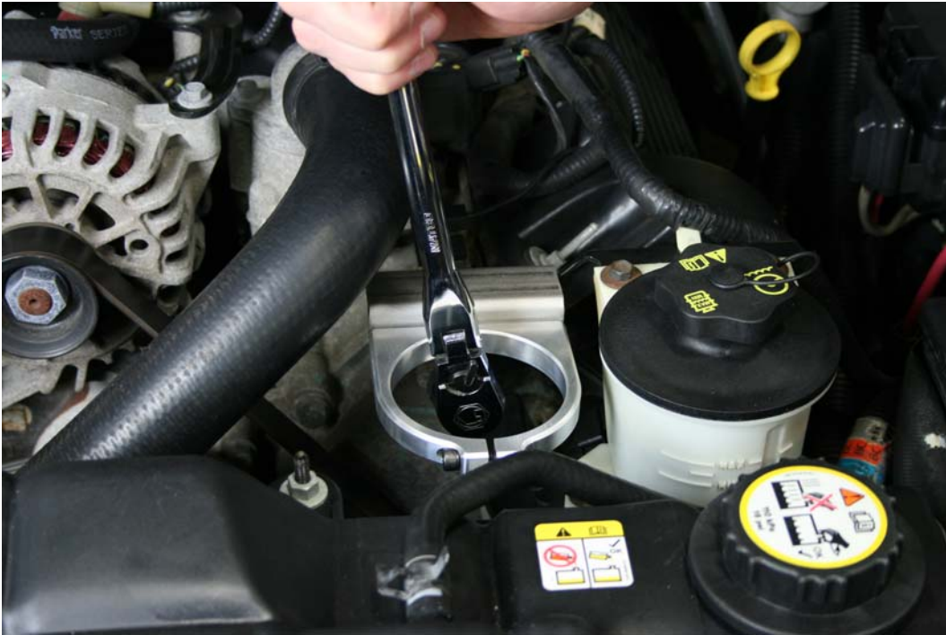
Step 1: Locate 8mm stud as shown and install Billet Stainless Mount
