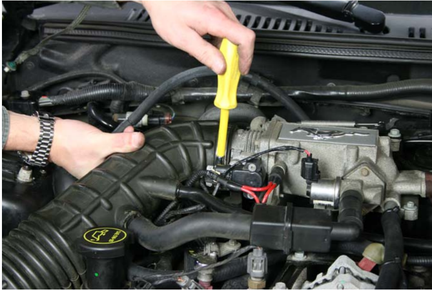
Step 30: Tighten clamp on throttle body side
