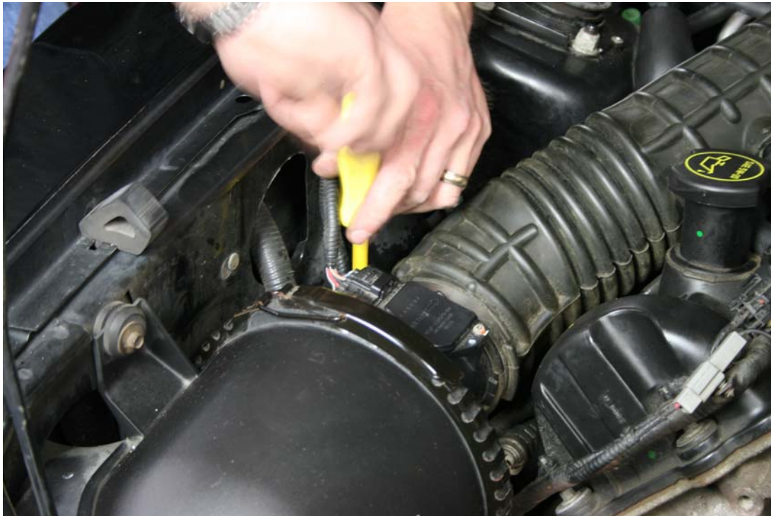
Step 31: Tighten clamp on Air Box side
