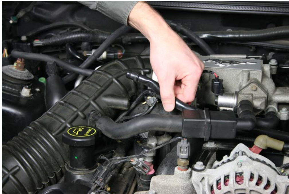
Step 2: Remove lines from Air Intake hose
