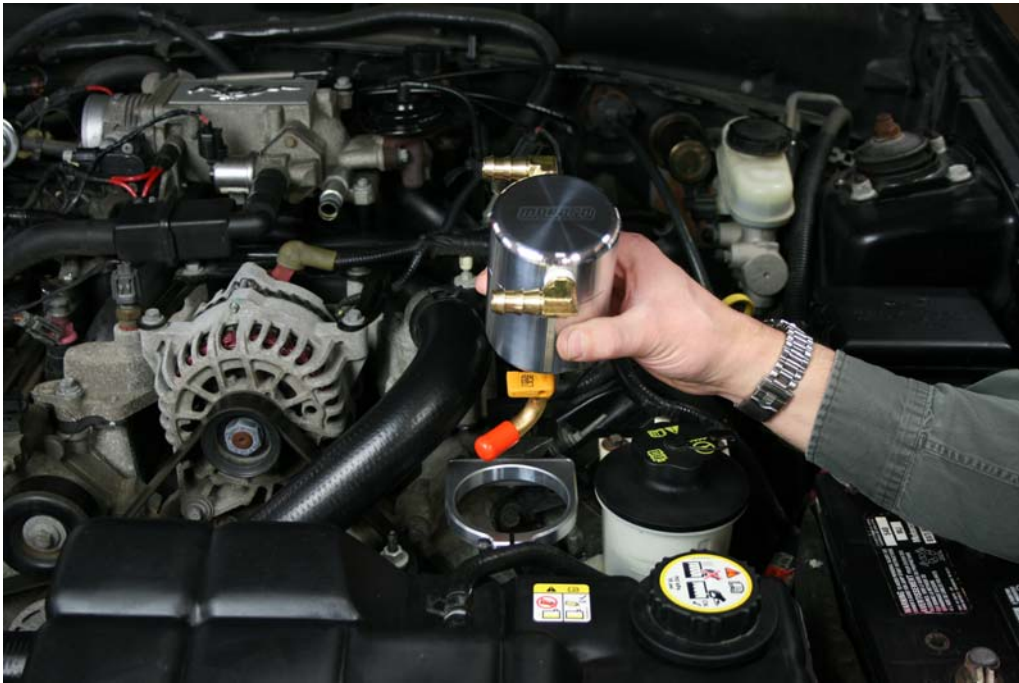
Step 12: Assemble Air Oil Separator as shown, apply Teflon Tape to all fittings
