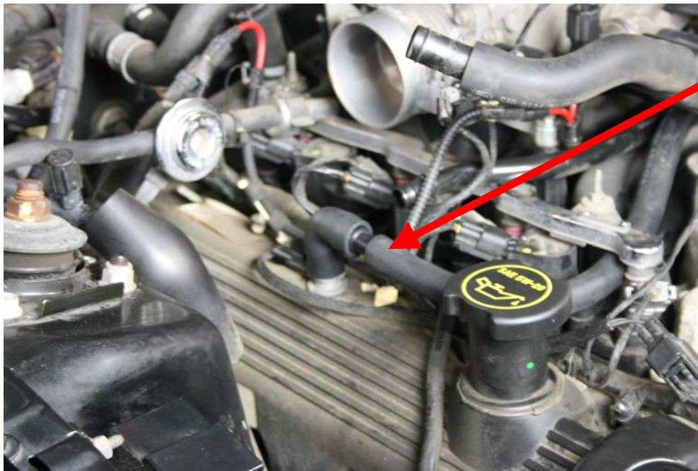
Step 19: Insert 1/2" hose over coupling
