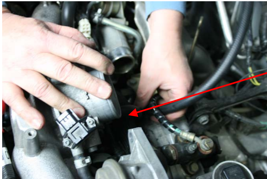
Step 20: Install 3/8" ID hose to PCV Valve under throttle body using hose clamp
