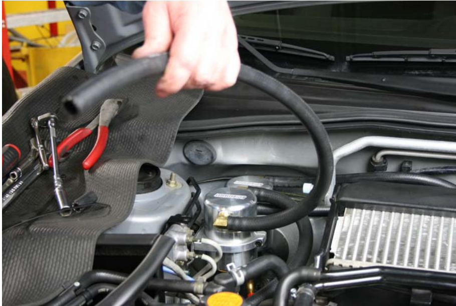
Step 34: Connect one end of 1/2" ID hose to front push lock fitting on Air Oil Separator
