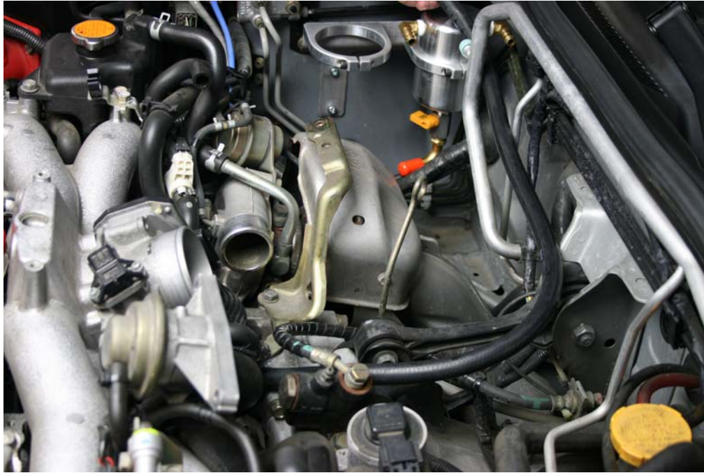
Step 21: Route 3/8" ID hose from PCV valve to air oil separator as shown
