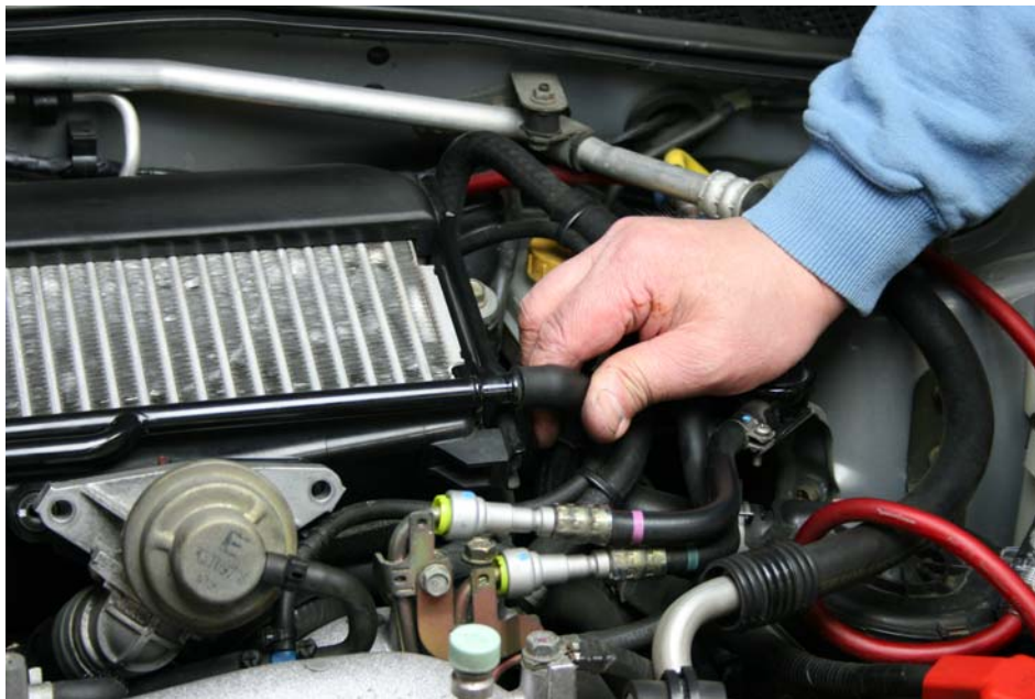
Step 31: Re-install intercooler cross over lines
