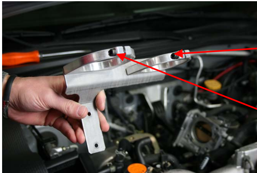
Step 16: Assemble billet clamps to stainless mounting bracket. Note orientation of 1/4" Allen head bolts
