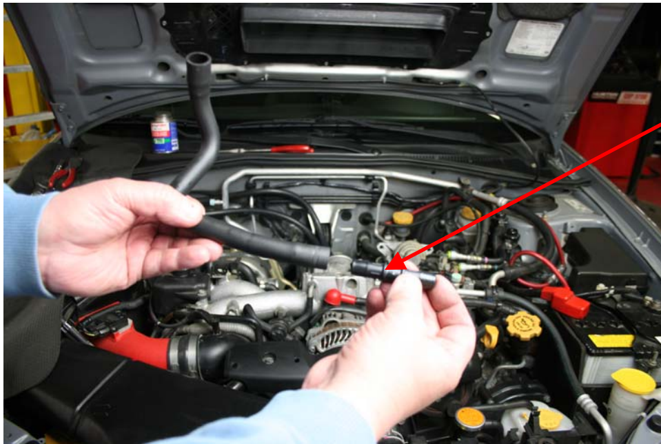
Step 26: Insert plastic nipple into breather hose that was removed in Step 15
