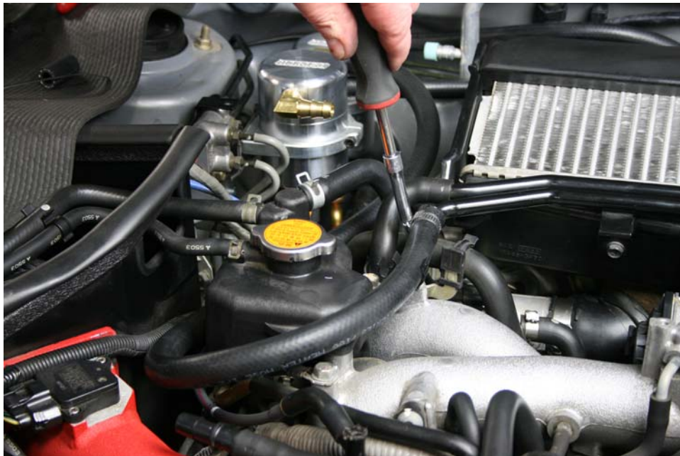
Step 33: Route 1/2" hose from Air Oil Separator to intercooler as shown, trim hose to length and secure with hose clamp on intercooler side
