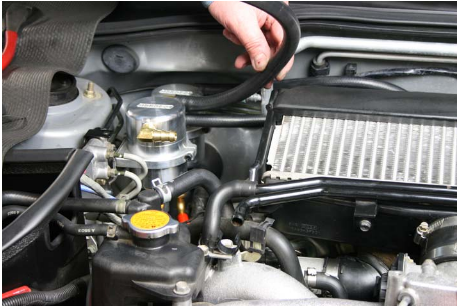
Step 32: Connect one end of 1/2" ID hose to rear push lock fitting on Air Oil Separator
