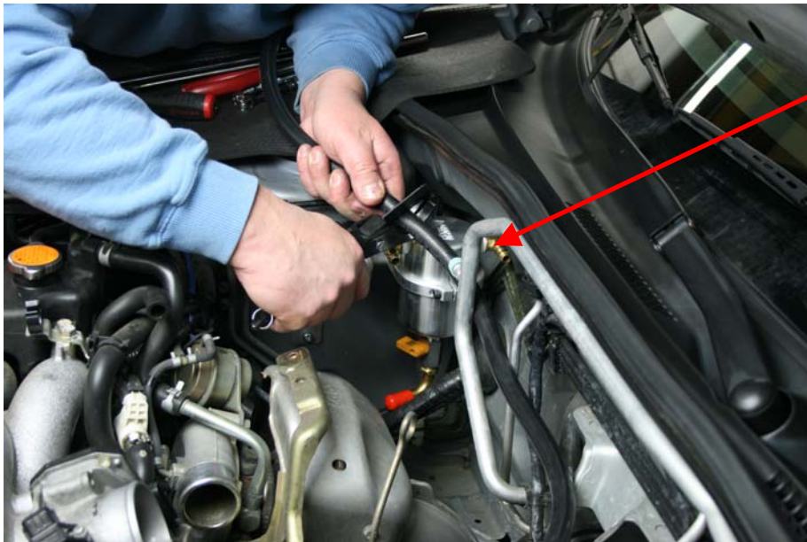
Step 22: Trim hose as needed and install to the rear 3/8" push lock fitting on the air oil separator
