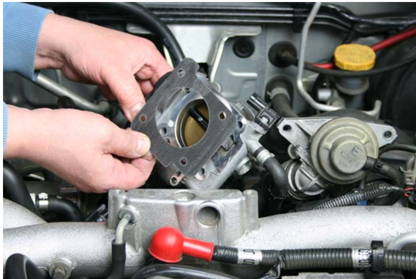
Step 28: Re-install throttle body using new gasket provided, re-connect electrical connections and install throttle body coupler
