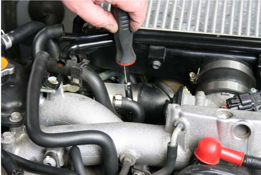
Step 7: Locate and loosen turbo outlet coupler
