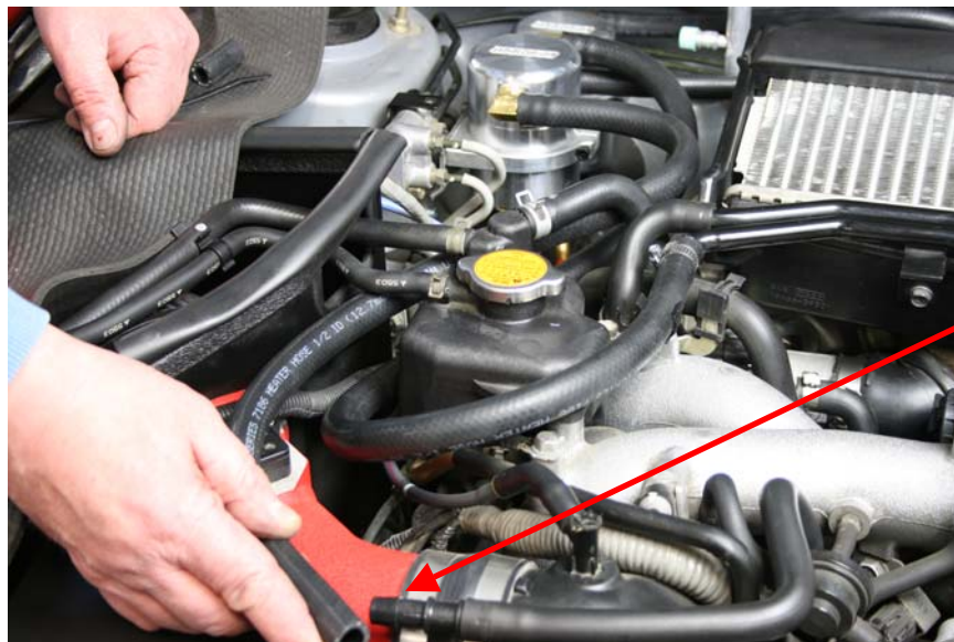
Step 35: Route 1/2" hose from air oil separator to breather hose as shown, trim hose to length and install to nipple
