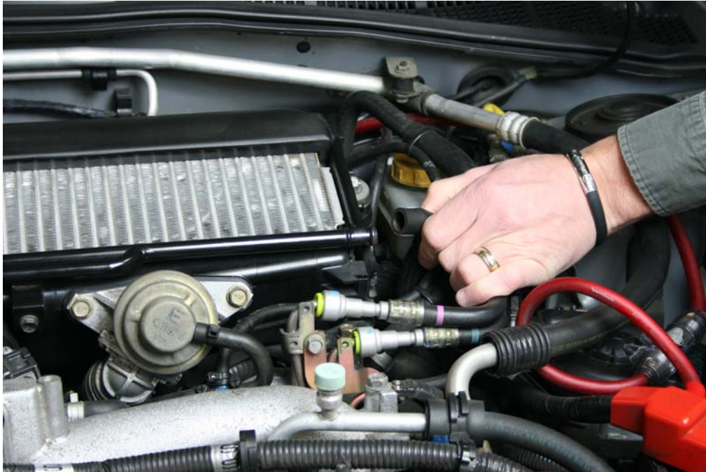
Step 2: Locate and remove intercooler cross over line on drivers' side
