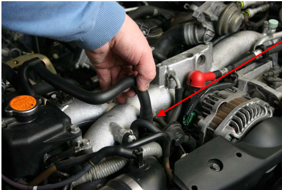
Step 15: Locate and remove other end of breather hose, set aside for re-use
