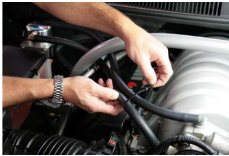
Step 9 Install 25 1/2" hose from top of intake to Air Oil Separator.
