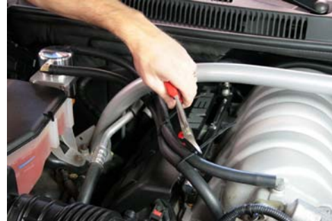
Step 10 Install wire ties as shown in 3 places.
