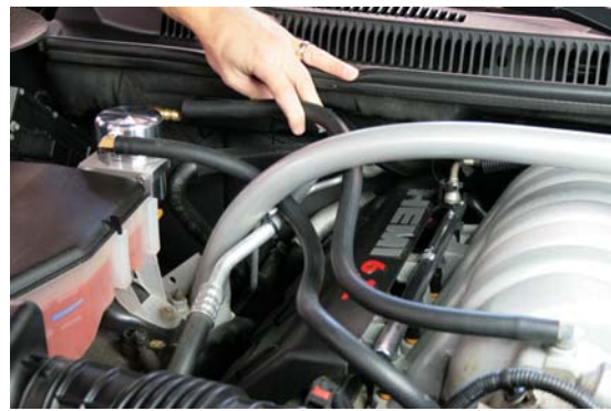
Step 9 Install 25 1/2" hose from top of intake to Air Oil Separator.
