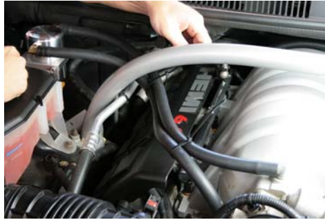
Step 9 Install 25 1/2" hose from top of intake to Air Oil Separator.
