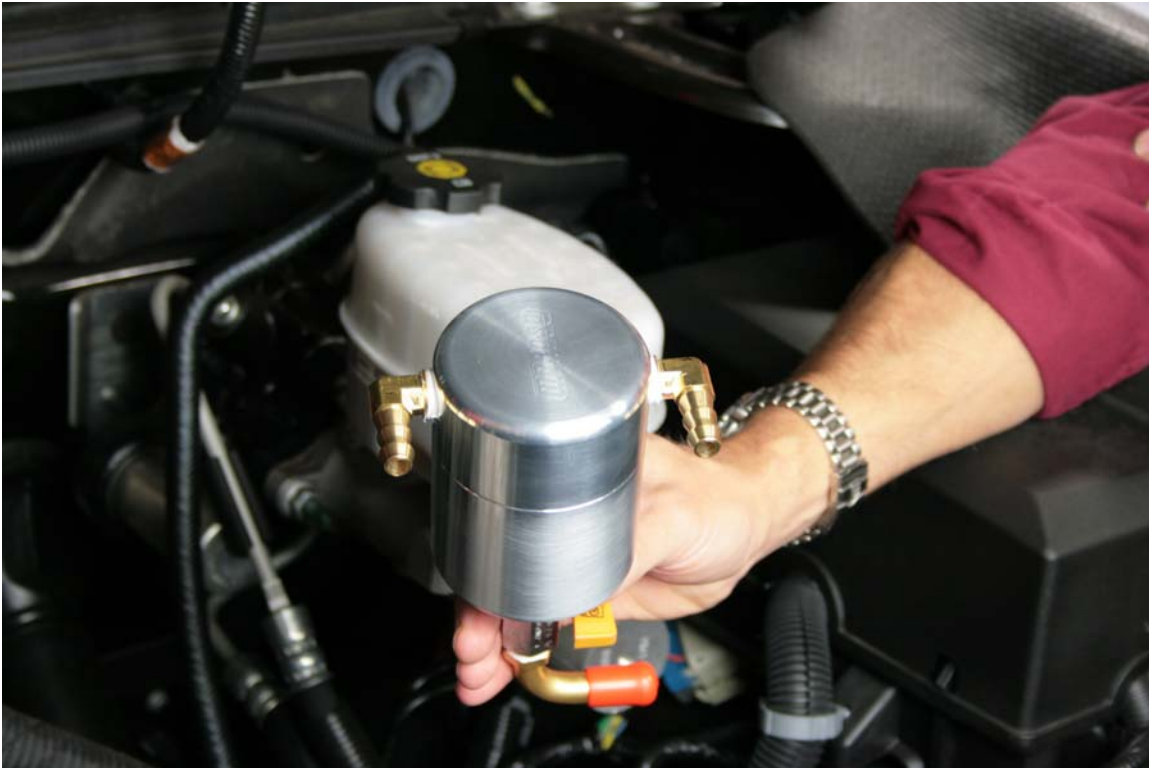
Step 19 Assemble air / oil separator as shown (note orientation of fittings, apply Teflon tape to all fittings)
