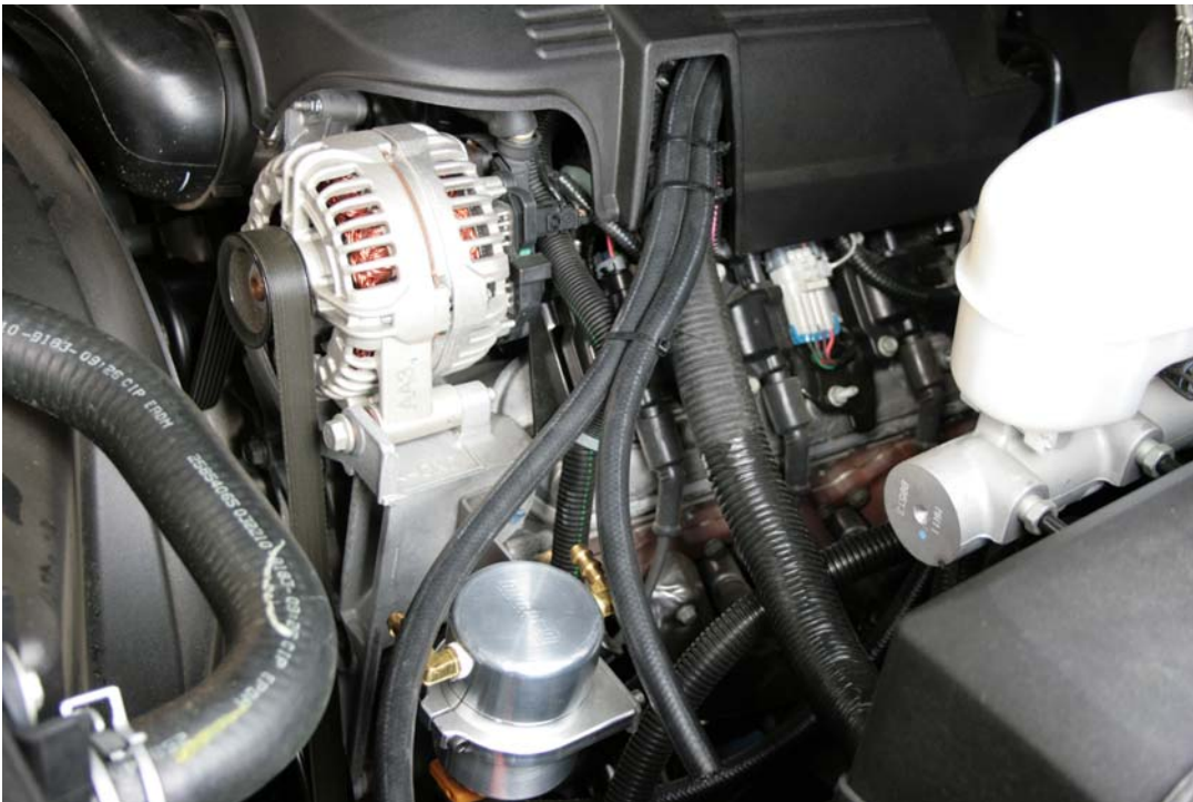
Step 23 Wire tie 3/8" lines as shown
