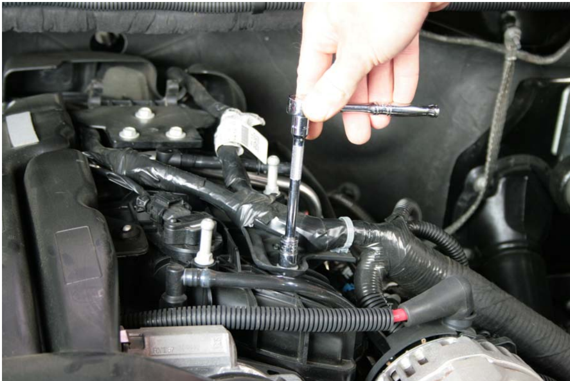
Step 15 Re-install wiring harness as shown
