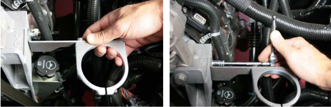
Step 18 Install billet / stainless bracket to upper hole on alternator bracket
