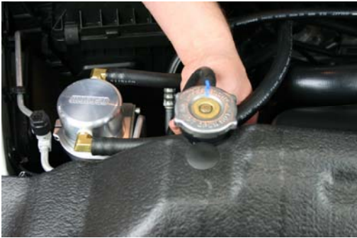
STEP 17 INSTALL 29" HOSE TO AIR OIL SEPARATOR
