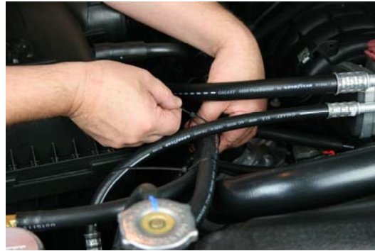
STEP 18 WIRE TIE 29" AND 36" HOSE TOGETHER
