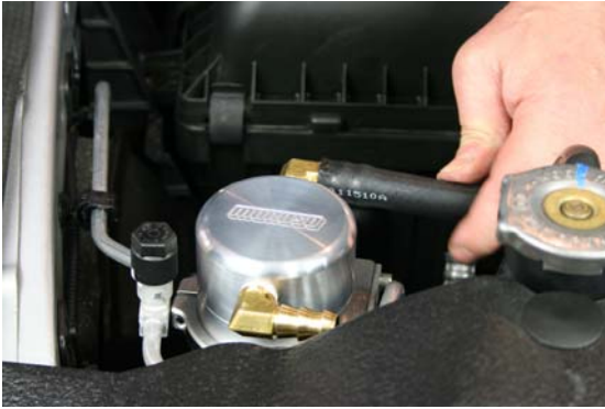
STEP 15 INSTALL 36" HOSE TO AIR OIL SEPARATOR
