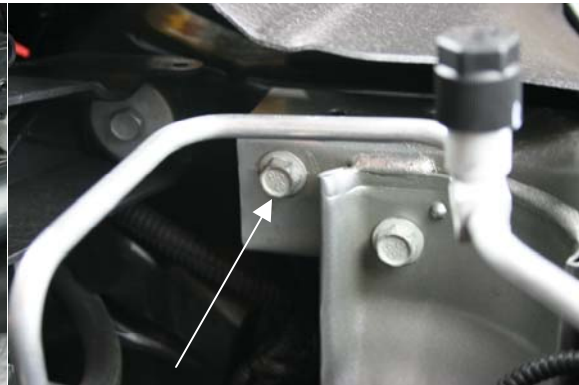
STEP 7 LOCATE MOUNTING BOLT ON RADIATOR SUPPORT PASSENGER SIDE
