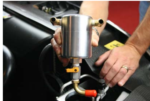
STEP 11 ASSEMBLE TANK BODY (NOTE ORIENTATION OF FITTINGS AND BALL VALVE) (APPLY TEFLON TAPE TO ALL FITTINGS)
