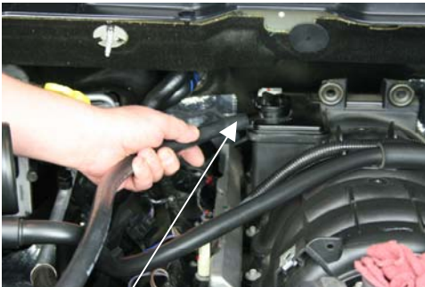
STEP 14 INSTALL 36" HOSE ROUTE AS SHOWN
