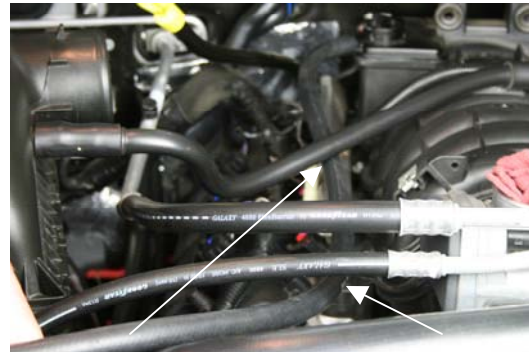
STEP 13 CUT (1) LENGTH OF HOSE @ 36" AND (1) LENGTH OF HOSE @ 29"
