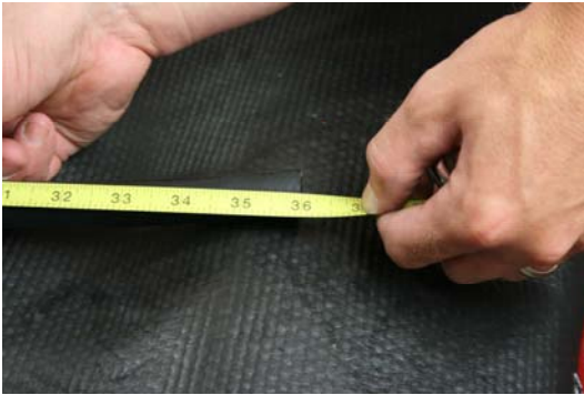
STEP 13 CUT (1) LENGTH OF HOSE @ 36" AND (1) LENGTH OF HOSE @ 29"
