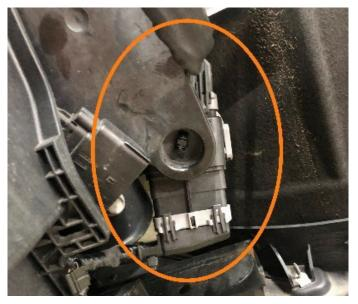
Remove the fresh air duct from the grille shutter assembly by pulling apart at this junction.
