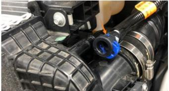
Remove 1x 8mm bolt securing the factory intercooler to the radiator.
