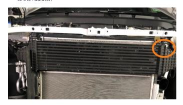
14. It may be helpful to use a pick tool or similar to start to remove the charge pipes from the intercooler so that the charge pipes come off the intercooler more easily when it is pulled away from the vehicle. Pinch the clip on the passenger side of the intercooler and pull the intercooler away from the vehicle. Then pull the intercooler up and away from the vehicle while removing the charge pipes.
