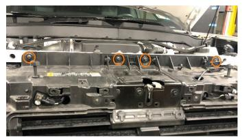
10. Remove the 7x 10mm bolts holding the bottom of the grille shutter assembly to the vehicle. If you have a 2020+ model, there may be 6x aluminum rivets instead of the 7x bolts. Drill the 6x rivets out using a ¼" or similar size drill bit.
