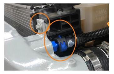
Install the MAP sensor and tighten with included 14mm long bolt (the longest of the 5 included bolts). Torque to approx. 89in-lbs.
