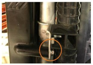
20. Trim the foam shrouds with scissors as shown to minimize contact with the Mishimoto intercooler and reinstall with factory clips.
