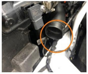
Remove hood latch cable by un-clipping cover and removing the cable. Move the cable out of the way.
