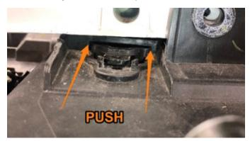
12. Remove the EVAP vacuum line with the blue connector by pushing the two blue tabs toward the rear of the car and push down. Loosen the clamp on both the inlet and outlet of the factory intercooler. It maybe beneficial to use a pick tool to loosen the coupler.
