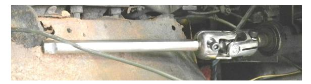
5. Slide support bearing with bracket up shaft. Line bracket up with holes on frame as pictured and bolt bracket down.
