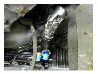
3. Slide upper u-joint on column so that the yokes are lined up in the same way and insert pinch bolt.
