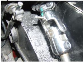
4. With supplied drill bit, drill a hole thru the u-joint and shaft, using the pre drilled hole as a pilot.
