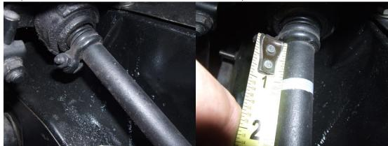
2. Cut steering shaft on 1" mark and remove the lower part of the stock steering shaft.
