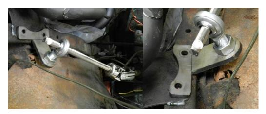
6. Insert middle joint with lower shaft so that the yokes on the joint are facing the same direction as the lower and upper (marked in red in the picture). You will have to trim the lower shaft to fit. Make sure all joints are lined up correctly and the support bearing is adjusted out where it needs to be before making your cut. Then grind a notch for the pinch bolt. Re-assemble the shaft kit, check for binds, and then tighten everything down.
