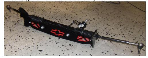
5. Now to install your new kit. With supplied hardware (2: ½-13 bolts and 2: 3/8-16 bolts). Bolt new R&P kit up into frame. Note: ½" bolts are used in drivers side and 3/8" bolts are for passenger side.
