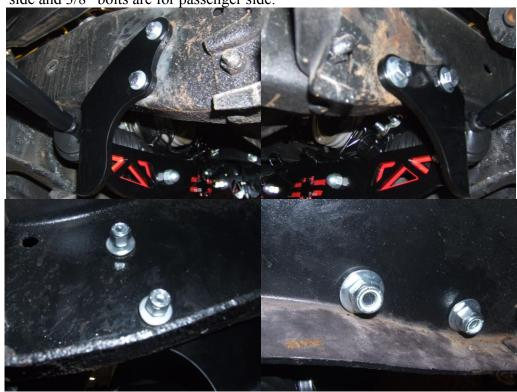
6. With new R&P system bolted into truck, its time to hook up the steering. Bolt tie rod ends into spindles.
