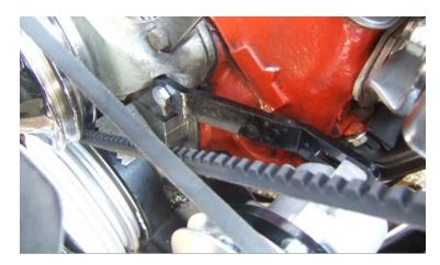
2. Replace stock water pump pulley with a two groove aftermarket pulley, as it is required to power new power steering pump.
