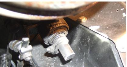
3. Install new intermediate shaft kit on the rack using the lower u-joint. Slide the upper u-joint onto the exposed remaining column shaft. Slide the intermediate shaft into the upper u-joint. Note: make sure end of existing steering shaft is flush with inside of u-joint. Tighten set screw on u-joint against the shaft with the u-joints phased 90 Degrees off one another.
