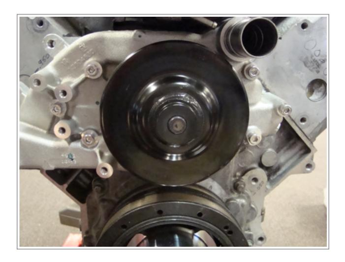
Mount the alternator (P587) in the upper outer hole just below the drivers head. Use a M10 x 80 MM SHCS (S562) and space the alternator from the block using a (AC7-.312) aluminum spacer as shown.
