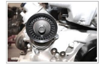
**PHOTO-10** Mount the power steering pump (P343) to the power steering bracket (19922A-08) with (2) M8 x 25 MM SHCS (S551). Note the pump mounts to the backside of the Bracket.
