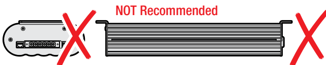
FIGURE 2.2.1.3: Do NOT mount the unit upside down
