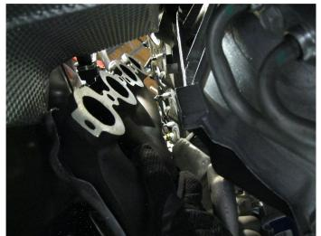
**Step 8.** Using a 1/2" socket unbolt both OEM header flanges. The OEM manifold assemblies can now be removed.
