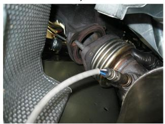
**Step 6.** Using a 15mm socket unbolt both catalytic converter inlet flanges from the OEM manifolds.
