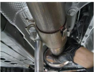
**Step 5.** Using a 15mm socket loosen both OEM clamps attaching the catalytic converter assembly to the OEM muffler assembly.
