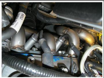
**Step 9.** Install your new header assemblies with the supplied gaskets and attach using the supplied header bolts with a 10mm socket to the manufacturers torque specifications.
