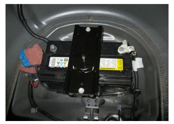
**Step 1.** Before removing the OEM header system, first disconnect the battery located in the vehicles trunk. Be sure not to close the trunk as it opens electronically.
