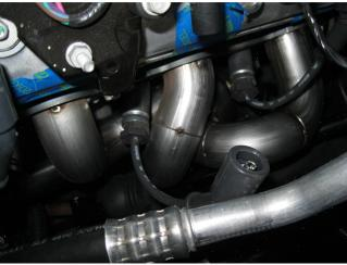
**Step 3.** Remove all spark plug wires from the coils and the plugs, then set aside. Next using a 5/8" socket remove the spark plugs for clearance.
