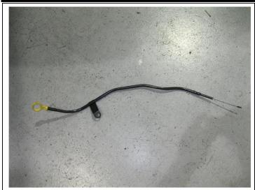
**Step 7.** Using a 15mm socket unbolt the dipstick assembly from the passenger side of the vehicle and remove.
