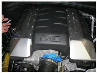
**Step 2.** Remove the engine cover by gently pulling to disengage it from the rubber grommets.
