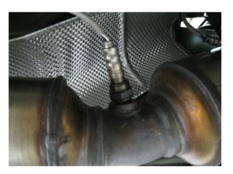
**Step 4.** Using a 7/8" wrench remove the O2 sensors in the catalytic converter assembly.
