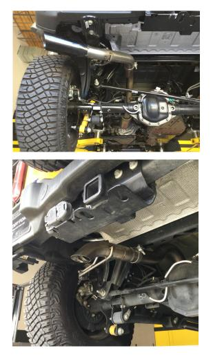
**Step 6**: Next attach the Tailpipe Assembly (either the Side Exit or Turn Down) to the Over Axle Pipe Assembly with the supplied 3.00" clamp and fit the hanger into the rubber insulator. .
