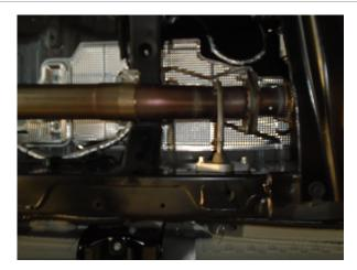
**Step 3**: Begin installation of your new MAGNAFLOW system by attaching the Resonator Assembly to the flex pipe using the supplied Fasteners. Engage the welded hanger to the rubber insulators. Keep all fasteners and clamps loose until final adjustment.
