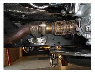
**Step 1**: Begin removal of the OE exhaust system by removing the fasteners attaching the exhaust to the flex pipe.
