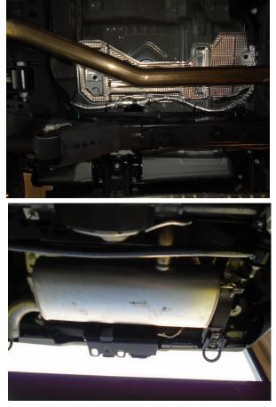
**Step 2**: With the system supported, working front to rear disengage the hangers from rubber insulators and remove the OE system. Do not discard or damage the clamp or rubber insulators as they will be used to install the new system.
