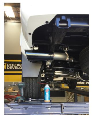
**Step 5**: Install the Tailpipe Assembly to the Over Axle Pipe fitting the hanger into the rubber Insulator.
