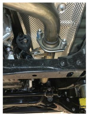
**Step 1:** To remove the OE exhaust system, remove the fasteners at the flange inlet at the front of the vehicle. Working front to rear disengage the hangers from the rubber insulators and drop the system. (Retain the Inlet fasteners, gasket and rubber insulators as they will be used to install your new system.)
