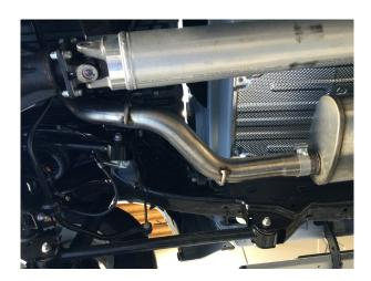
**Step4:** Next, attach the Overaxle pipe to the Muffler Assembly using the supplied 3.00" clamp and fit the hangers into the rubber insulators.
