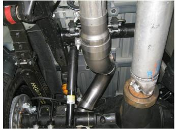
**Step 2.** Begin installation of the Magnaflow system by first clamping the 4"-5" Adapter Nipple to the newly cut outlet of the DPF using a supplied 4.00" clamp. Then attached the Over Axle Assy to the Adapter Nipple using the supplied 5" clamp and fitting the hangers in the rubber insulators (leave all clamps loose for final adjustment of the complete system).
