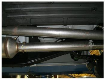
**Step 1.** To begin the removal of the OEM system you will need to cut 31.50" behind the DPF. You can then disengage the welded hangers from the rubber insulators, working rearward finish removing the system. Do not damage or discard the rubber insulators, as they will be reused to mount the new system.
