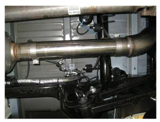
**Step 3.** The longer Inlet Pipe Extension will be needed for Long Bed applications only.
