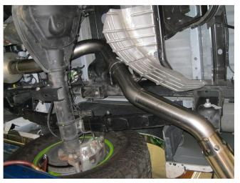
**Step 6.** Next Install the Tail Pipe Assembly in a similar fashion using the supplied 5.00" clamps and by fitting the welded hangers into the rubber insulators.
