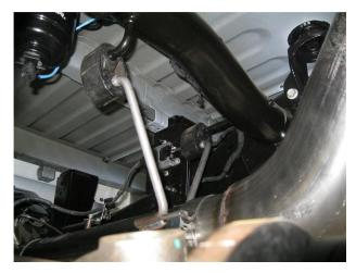
**Step 4.** When using the long bed extension pipe attach the OEM cable bracket using the OEM bolt.
