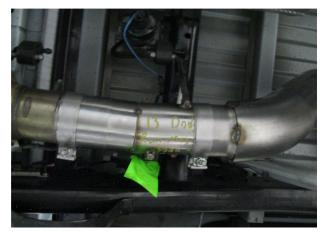
**Step 5.** The shorter Inlet Pipe Extension will be needed for all Mega Cab applications.
