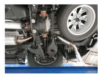
**Step 3.** Next Install the Mid pipe to the Resonator Assembly using a supplied 3.00" clamp. Complete the installation by attaching the Tailpipe / Muffler Assembly using the supplied 3.00" clamp and fit the welded hanger into the rubber insulator.
