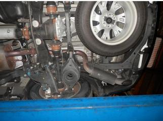
**Step 1.** To remove the OEM exhaust system begin by un-fastening the 2 bolt flanges at the catalytivc converter outlets and behind the muffler. Next, working rearward with the exhaust supported disengage the hangers from the rubber insulators and remove the system. Do not damage or discard the rubber insulators or fasteners as they will be re-used to mount the new system.
