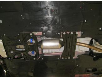
**Step 1.** Removal of the exhaust system requires cutting and de-burring the pipe 2.25" behind the rear hanger attachment point at the rear of the catalytic converter. To accomplish this you must remove the cross brace and catalytic converter shield.
