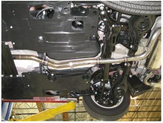
**Step 3.** Next attach the Resonator Assembly to the outlet of the catalytic converter using the supplied 2.50" Clamp followed by the Mid-Pipe using a 2.25" clamp. Leave all clamps loose until final adjustment
