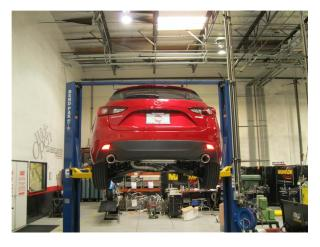
**Step 5.** Once a final position has been chosen for the new exhaust system, evenly tighten all clamps from front to rear using the torque specifications on page one of the instructions. Replace the shield and cross brace. Inspect all fasteners after 25-50 miles of operation and re-tighten if necessary.
