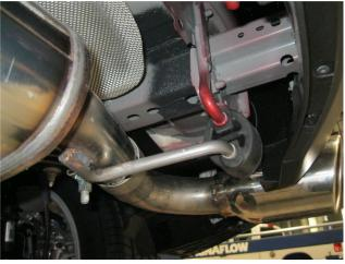
**Step 4.** Finish by installing both the Muffler Assembly and both Tip Assemblies using the supplied 2.25" clamps, fitting the hangers into the rubber insulators.
