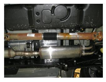
**Step 2.** Begin installation of the new system by attaching the Muffler Assembly to the factory outlet using the supplied 3.00" clamp and fit the hangers into the rubber insulators. Ensure that the indexing slot on the inlet is properly engaged with the pin. Leave all clamps loose until final adjustment.
