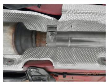
**Step 3.** Begin installation of the new system by slipping the new Inlet Pipe over the outlet of the catalytic converter that you have just cut. Loosely secure using the supplied 2.25" clamp.
