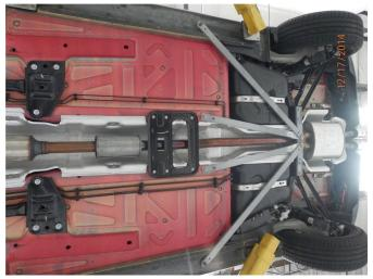
**Step 1.** Removal of the OEM exhaust system requires removing the underbody chassis braces by unbolting them. Use the 10mm socket and T-150 Torx.
