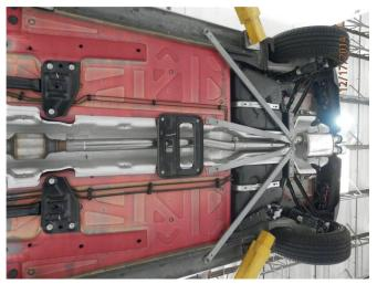
**Step 4.** Loosely install the Muffler Assembly using the supplied 2.50" clamp. Locate both welded hangers to the OEM rubber insulators. At this point replace both underbody braces.
