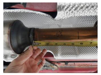
**Step 2.** Next, cut the OEM exhaust pipe 5.50" behind the catalytic converter as shown. Deburr and clean any rough edges. Disengage the welded hangers from the rubber insulators. The OEM exhaust may now be removed. Be sure to retain all mounting hardware as it will be needed to install your new MAGNAFLOW performance exhaust system.
