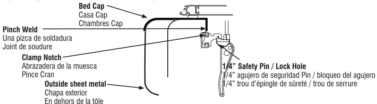
**If traveling with the Tonneau in the folded position it is recommended to use a safety pin or lock in the front clamps.**
