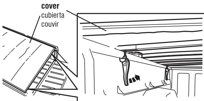
**Rotate clamp up from its install position into its storage position as shown left. Make sure that latch handle matches illustration on bow caution label.**
