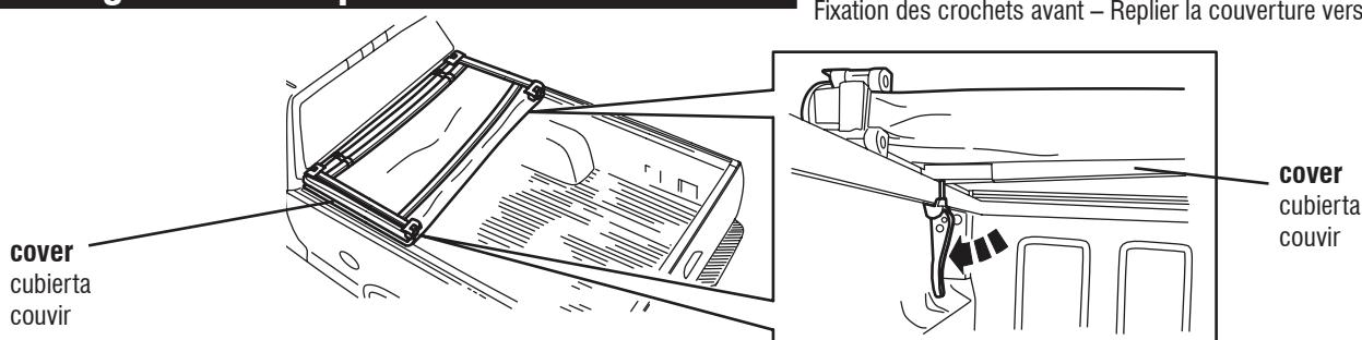
**NOTE: Clamp handle must rotate completely down to the stop to be locked. If something interferes with the handle (bed liner, bed extender or cargo, etc.) it must be modified or removed.**
