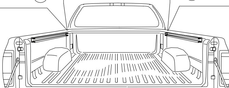
**Insert 2 adapters (item B) into each bed sidewalk track as shown and re-install caps.**
