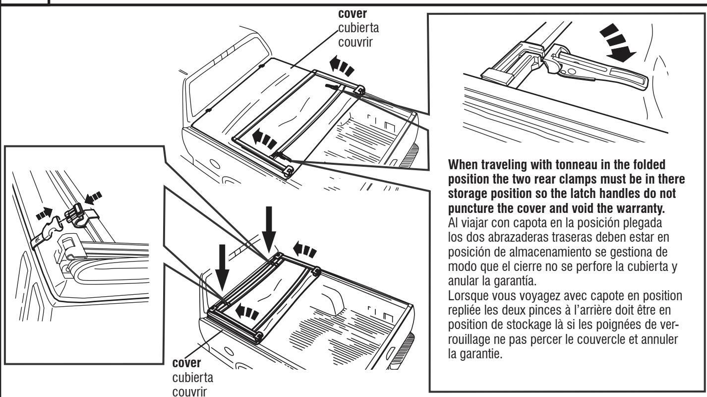
**When traveling with tonneau in the folded position the two rear clamps must be in there storage position so the latch handles do not puncture the cover and void the warranty.**
