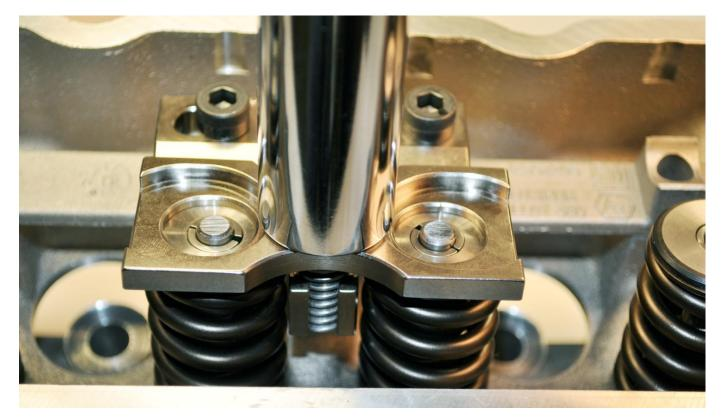
Make sure the valves stems and locks are centered in the windows on the compressor top. Begin compressing the springs using a 7/8 deep socket.
