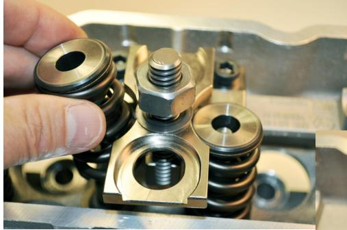
No need to remove the frame top in order to remove and replace springs!
