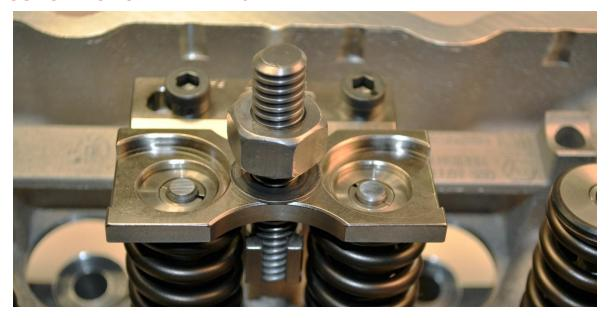
Remove the rocker arms on the cylinder you will be changing springs. Bolt the SC-167 in place using the 8mm cap screws approximating 8-10 ft. lbs. of torque. The main idea is not to over tighten the cap screws. Again, make sure the piston is up in that hole so you don't drop the valves or use a suitable air fitting adaptor in the spark plug hole and compressed air to hold the valves in place.
