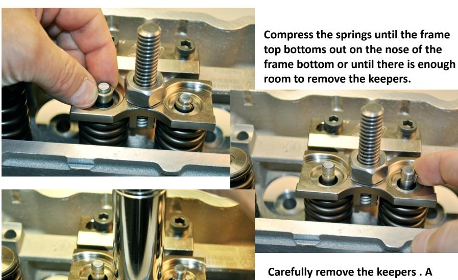
Carefully remove the keepers . A magnetic tool can be helpful for this. After removing the keepers raise the frame top .
