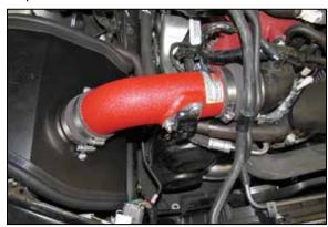
14. Install the K&N® intake tube into the coupler at the turbo inlet tube and align with the filter adapter, slide the coupler onto the filter adapter, adjust the tube for best fit and secure with the hose clamps. Secure the heat shield with the provided hardware.
