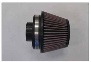
9. Install the K&N® air filter onto the provided filter adapter and secure with the provided hose clamp.
