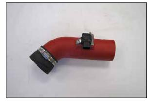
12. Install the provided hose coupler (084036) onto the intake tube. Do not completely tighten the hose clamp at this time.
