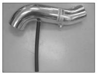
20. Install the provided hose onto the K&N throttle body tube as shown. **NOTE**: Before installing the hose, inspect the inside of the tube for any debris, then clean the inside out with water and a towel. Inspect the tube one more time before proceeding to the next step.
