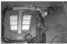
37. Reinstall the engine cover as shown
