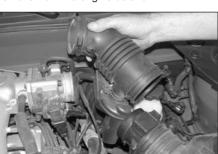
7. Loosen the hose clamps at the throttle body and at the mass air sensor, then, remove the stock intake tube as shown.
