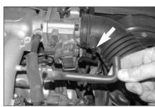
6. Disconnect the crank case vent hose and remove from the engine as shown.
