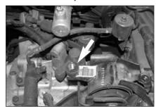
18. Install the provided rubber mounted stud into the original air cleaner mounting hole as shown.
