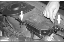
31. Secure the fuse box using the original bolts.
