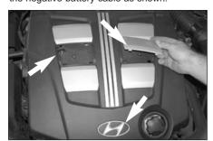
2. Remove the three engine cover panels using a flat blade screwdriver.
