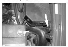
14. Remove the bolt that secures the air cleaner duct to the inner fender as shown.
