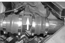
32. Reconnect the mass air sensor and secure with the wire clip as shown.
