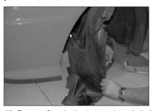
12. Remove five plastic rivets and one bolt, then, pull in the inner fender valance down as shown.
