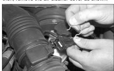
5. Remove the wire clip, then, disconnect the mass air sensor electrical connection as shown.
