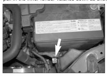
13. Remove the bolt that secures the air inlet duct to the battery tray as shown.
