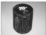
29. Install the K&N Drycharger onto the K&N Filtercharger as shown.
