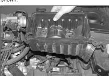
9. Remove the lower air cleaner assembly, which is secured by three bolts.
