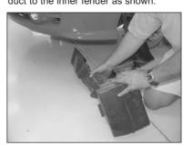
15. From underneath the vehicle remove the two bolts and one clip, then, remove the resonator from the vehicle as shown.
