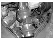
25. Slide the mass air sensor assembly onto the throttle body tube and snug the hose clamp but do not tighten completely at this time.
