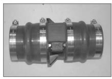
24. Install the two silicone hump hoses and hose clamps onto the mass air sensor and secure as shown.
