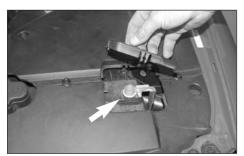
1. Turn the vehicles ignition off and remove the negative battery terminal cover, then, disconnect the negative battery cable as shown.
