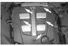
3. Remove the engine cover, which is secured by 5 bolts as shown.
