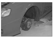
11. Raise the vehicle up and support it with a jack stand, then, remove the front tire as shown.
