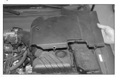
4. Remove the two plastic rivets and one bolt, then, remove the air cleaner cover as shown.
