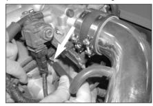
22. Connect the crank case vent hose to the crank case vent as shown.
