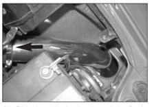
27. Slide the cold air tube through the fender from underneath the vehicle and into the silicone hump hose as shown.
