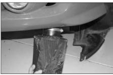
30. Install the Filtercharger from under the vehicle and secure with the provided hose clamp as shown.
