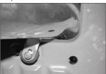
28. Line up the cold air tube bracket with the rubber mounted stud from step 26 and secure with the provided hardware as shown.
