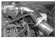
21. Slide the intake tube into the silicone hose on the throttle body, then line up the threaded boss with the bracket from step 19 and secure with the provided hardware, but do not tighten at this time.
