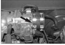
17. Install the silicone hose and hose clamps onto the throttle body and secure as shown.
