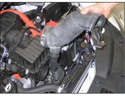
5. Remove the fresh air intake scoop from the vehicle.
