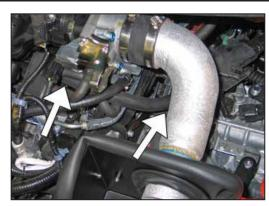
26. Attach the provided crankcase vent hose to the valve cover port, and then attach the open end to the 90° fitting in the intake tube.
