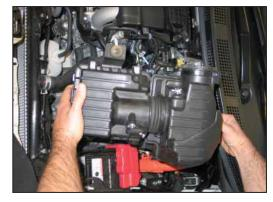
8. Remove the airbox assembly from the vehicle. NOTE: It will be necessary to release the spring clamp securing the crankcase vent tube and hold the crankcase vent tube while removing the airbox.
