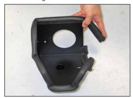
20. Install the 42" long edge trim around the heat shield.
