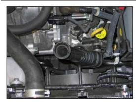
10. Reinstall the lower fresh air duct onto the factory plastic duct as shown.
