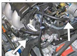
14. Remove the cap plugs and install the bypass hose onto the coolant fittings and secure with the provided hose clamps.
