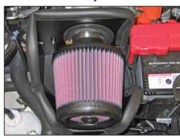
27. Install the K&N® air filter onto the intake tube and secure with the provided hose clamp.
