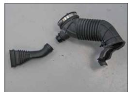
9. Separate the lower intake duct from the fresh air intake scoop.
