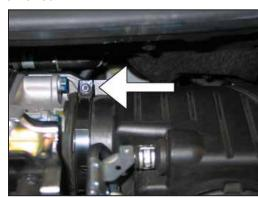
6. Loosen the hose clamp securing the intake hose to the throttle body.
