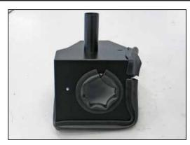
21. Install the 11" long edge trim into the hole of the heat shield.
