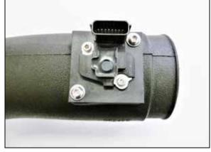
14. Install the mass air sensor assembly into the K&N intake tube and secure with the provided hardware. Be sure to install the sensor in the correct direction as shown.
