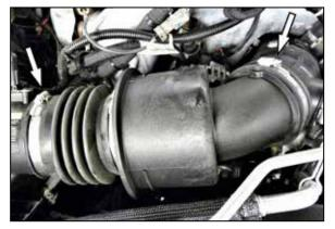
2. Loosen the two hose clamps securing the factory intake hose and then remove the hose from the vehicle.
