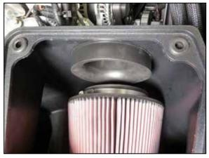
9. Install the filter adapter into the filter housing and secure with the provided hardware.
