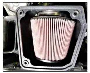
10. Slide the K&N air filter onto the filter adapter and secure with the provided hose clamp.
