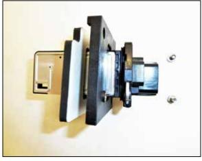
13. Remove the mass air sensor from the factory air filter housing. Assemble the mass air sensor, adapter and gasket as shown.
