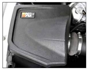
11. Install the K&N badge onto the lid and then install the lid onto the air filter housing as shown.
