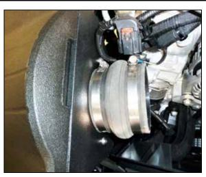
12. Install the provided hump coupler onto the filter adapter and secure with the provided hose clamp.
