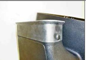
5. Using the provided push pins, install the fresh air intake hood seal onto the K&N air filter housing.
