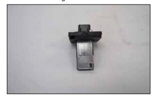
13. Remove the mass air sensor from the factory air filter housing and install the sensor and provided gasket into the K&N® mass air sensor adapter using the provided hardware.
