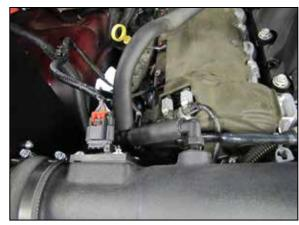
20. Using the provided vent hose, connect the factory vent to the 90° fitting installed into the K&N® intake tube. Reconnect the mass air sensor electrical connection.
