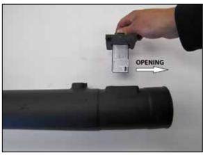
14. Install the mass air sensor assembly into the K&N® intake tube as shown, secure the sensor with the provided hardware.
