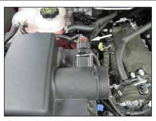
5. Release the red locking tab and then disconnect the mass air sensor electrical connection and unhook the harness from the air filter housing.
