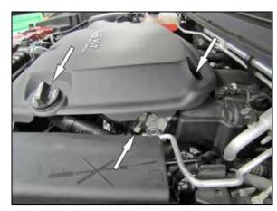
3. Remove the oil fill cap and loosen the hose clamp securing the intake hose to the throttle body. Remove the bolt securing the intake plenum to the engine.
