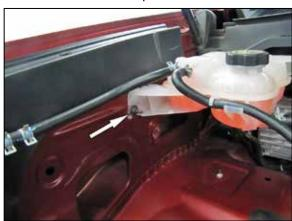
11. Remove the nut that secures the coolant reservoir to the inner fender.
