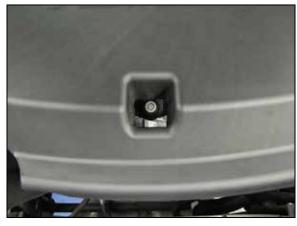
4. Remove the front center bolt securing the intake plenum to the engine and remove the intake plenum from the vehicle.
