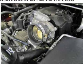
15. Install the provided coupler (08186) onto the throttle body and secure with the provided hose clamp
