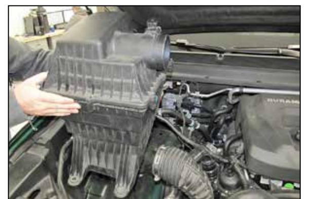
5. Remove the complete air filter housing from the vehicle.
