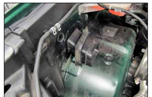
6. Remove the inlet duct from the inner fender.
