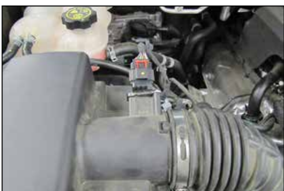
2. Disconnect the mass air sensor electrical connection.
