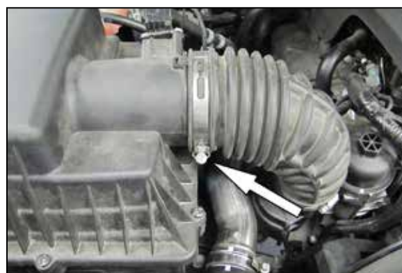
3. Loosen the hose clamp that secures the intake tube to the air filter housing and then disconnect the intake tube from the air filter housing.
